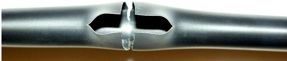
(c) Post-test image of rupture view
