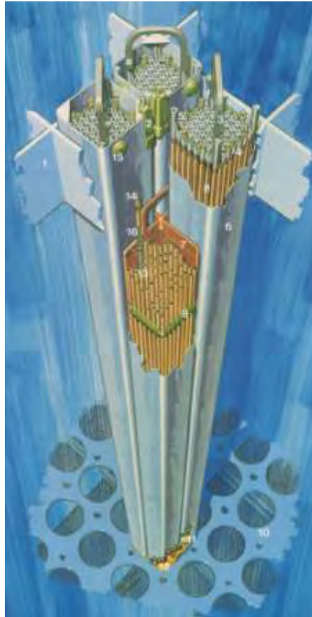
Figure 4-5 Module of Four BWR Fuel Assemblies and Associated Channel Boxes 8
