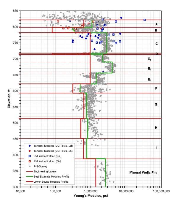
Figure 2.5.4-241 Elastic Modulus Models for Settlement Analysis
