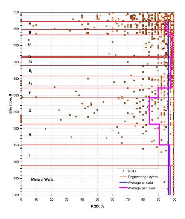
Figure 2.5.4-240 Rock Quality Designation vs. Elevation
