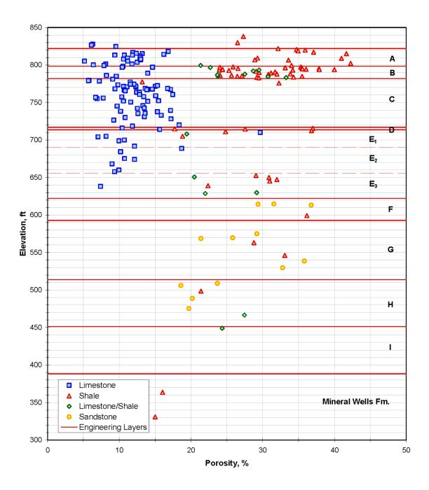
Figure 2.5.4-221 Calculated Porosity vs. Elevation
