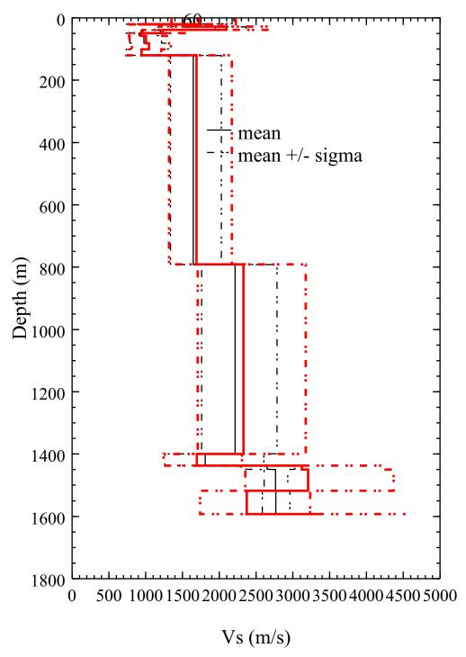
Note: The calculated median+sigma from the artificial profiles (black dashed line) is lower than the target median+sigma at depths greater than 800 m because the distribution of Vs is truncated by the Vs of bedrock (9200 fps or 2,804 m/s) implicit in the EPRI attenuation equations.
