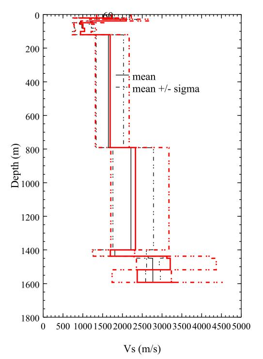
Note: The calculated median+sigma from the artificial profiles (black dashed line) is lower than the target median+sigma at depths greater than 800 m because the distribution of Vs is truncated by the Vs of bedrock (9200 fps or 2,804 m/s) implicit in the EPRI attenuation equations.
