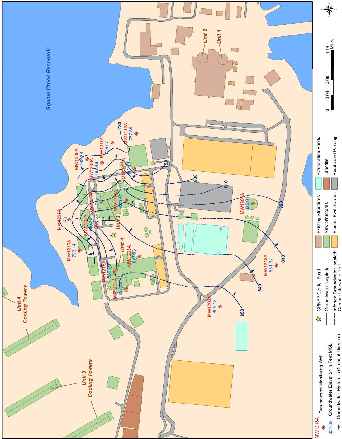
**Figure 2.4.12-210 Potentiometric Surface Maps (Sheet 3 of 4)**
