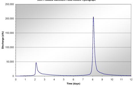
Figure 2.4.3-207 SCR Probable Maximum Flood Inflow Outflow Hydrographs
