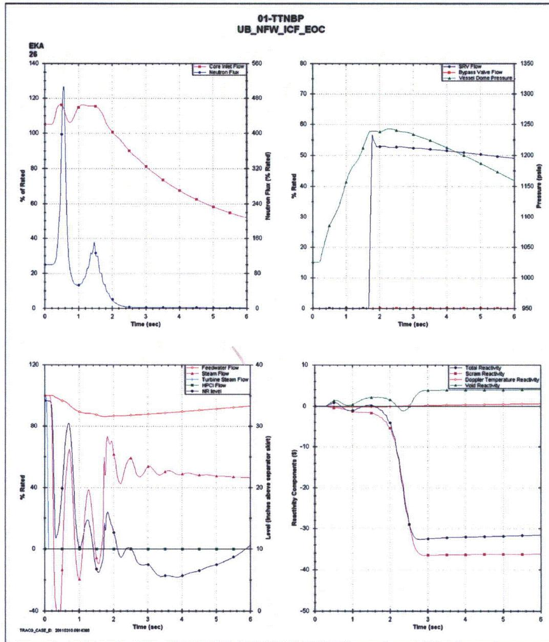
**Figure 4 Plant Response to Turbine Trip w/o Bypass
