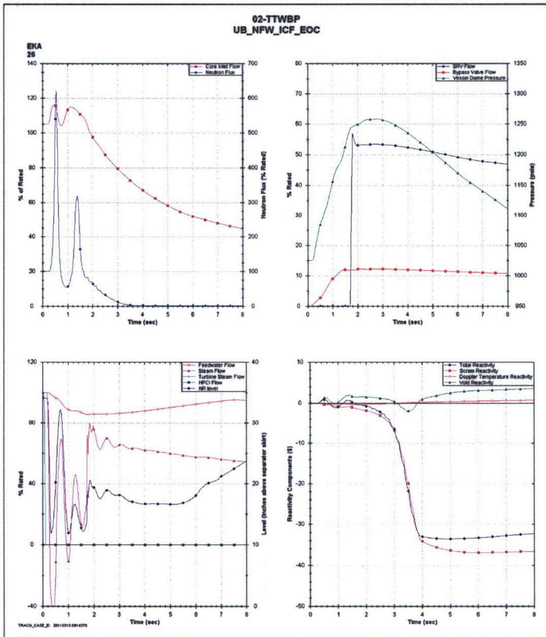
**Figure 3 Plant Response to Turbine Trip with Bypass
