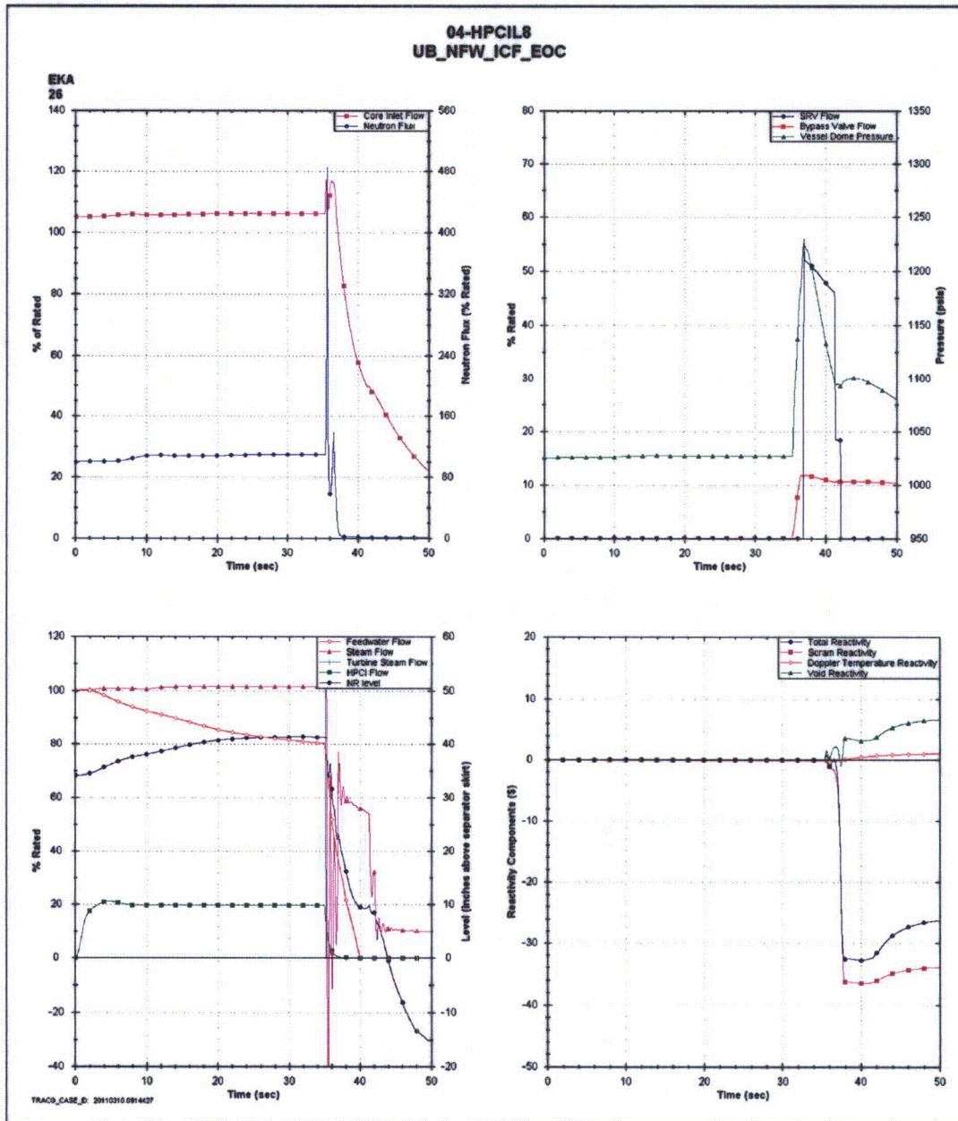
**Figure 6 Plant Response to Inadvertent HPCI /L8
