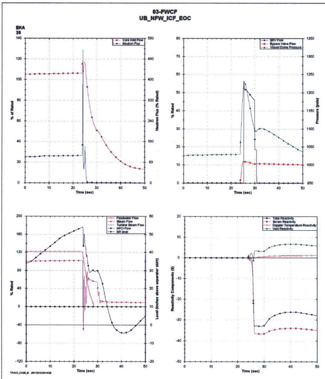
Figure 2 Plant Response to FW Controller Failure
