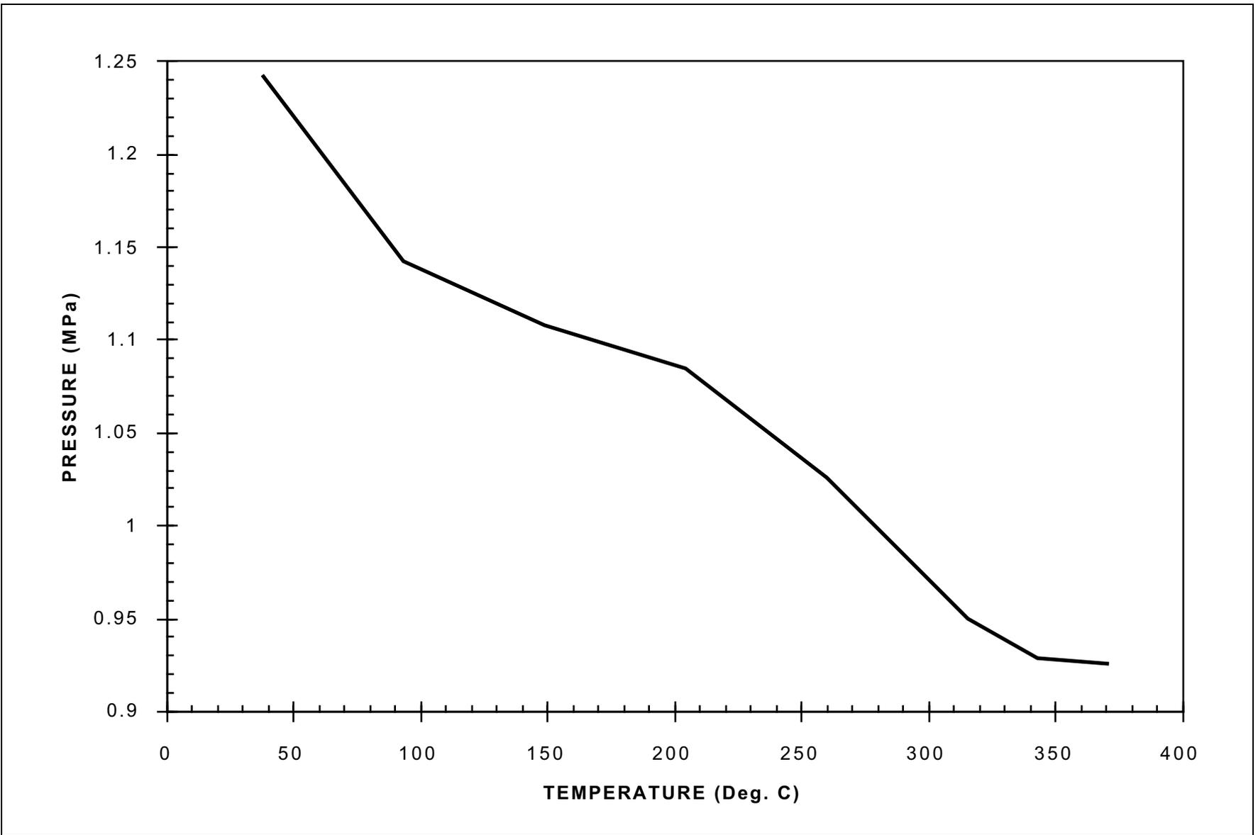
Figure 19F-5 Drywell Head Pressure Capability vs Temperature
