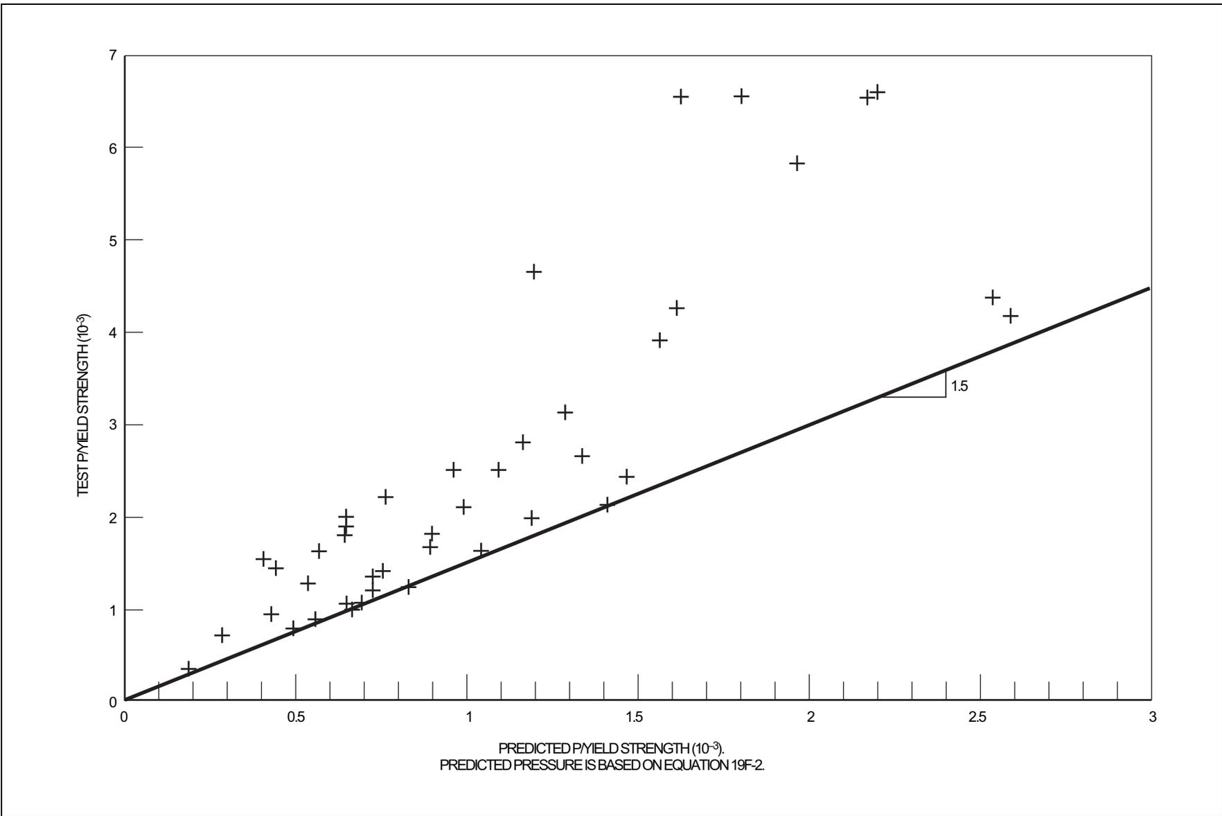
Figure 19F-6 Torispherical Head Buckling Test Data
