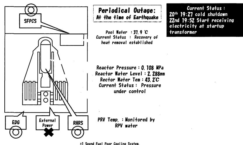
\*Z:Emergency Diesel Generator \*3:Residual Heat Removal System
