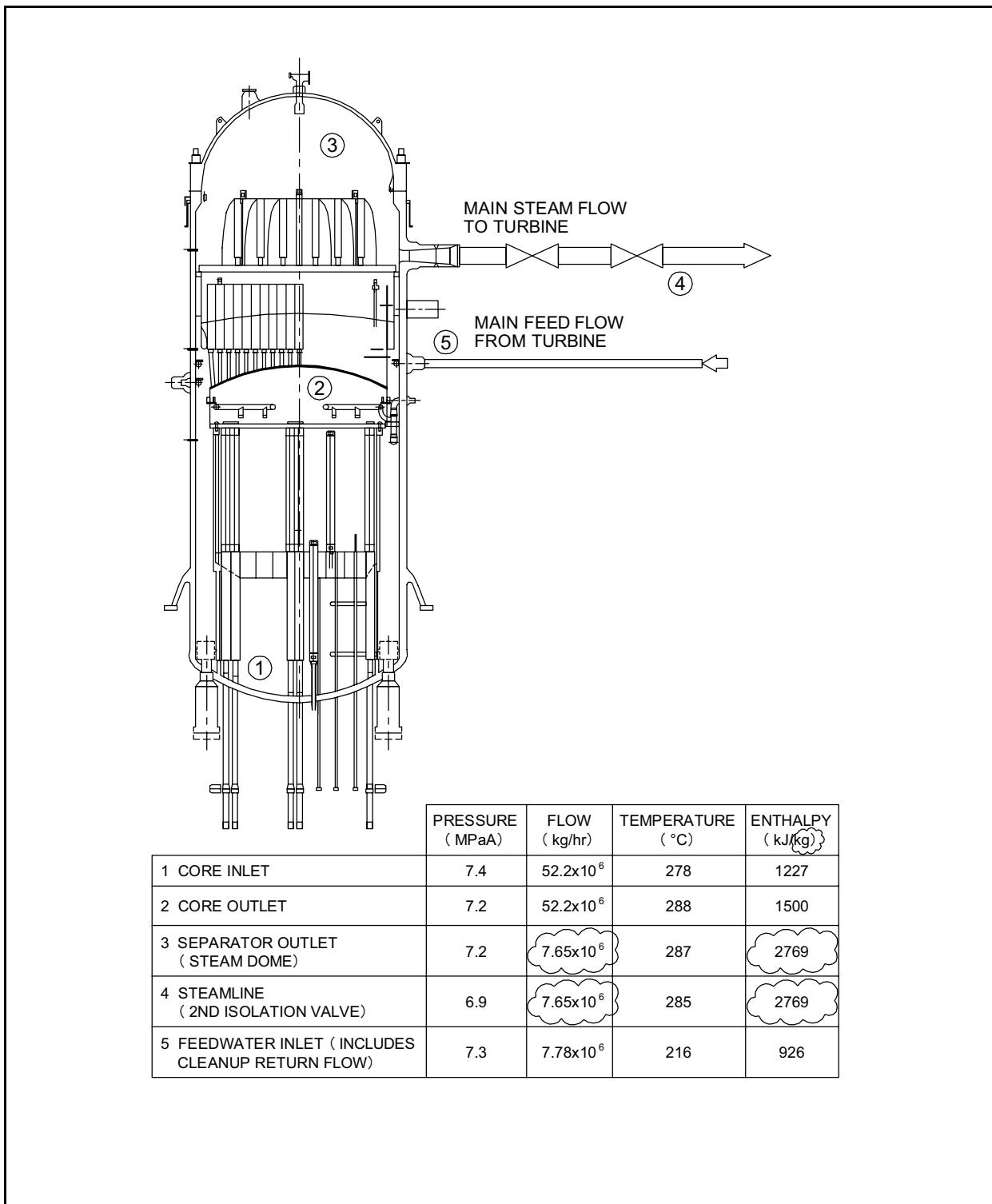
**Figure 5.1-1 Rated Operating Conditions of the ABWR**
