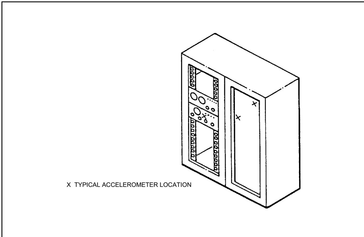
Figure 3.10-2 Instrument Panel
