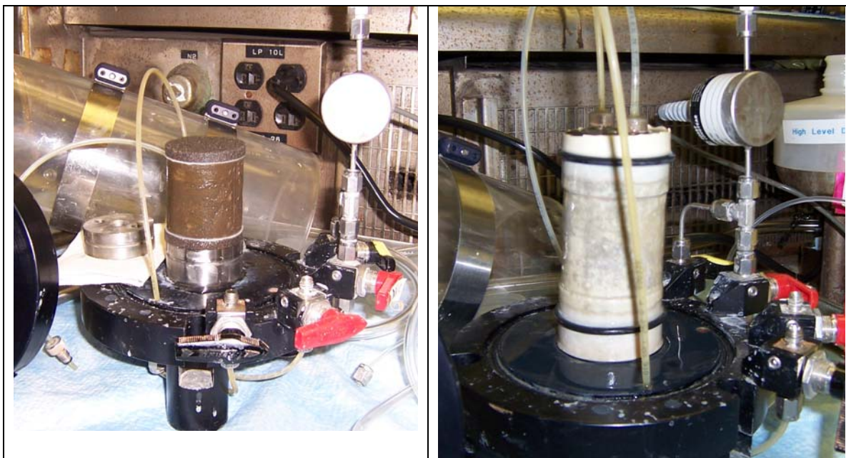
Figure 5 Saltstone sample in flexible wall permeameter.
