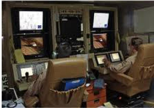
**Figure 5-1 Unmanned aircraft system (UAS) - Predator UAV and control station**
