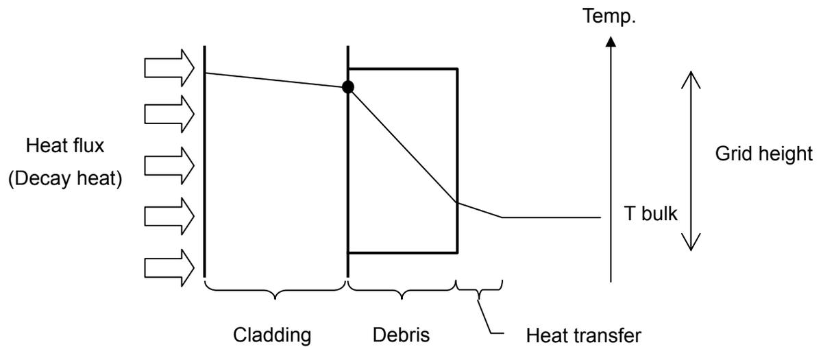
**Figure 4.2.1-2 Schematic Drawing of the Analysis Model**
