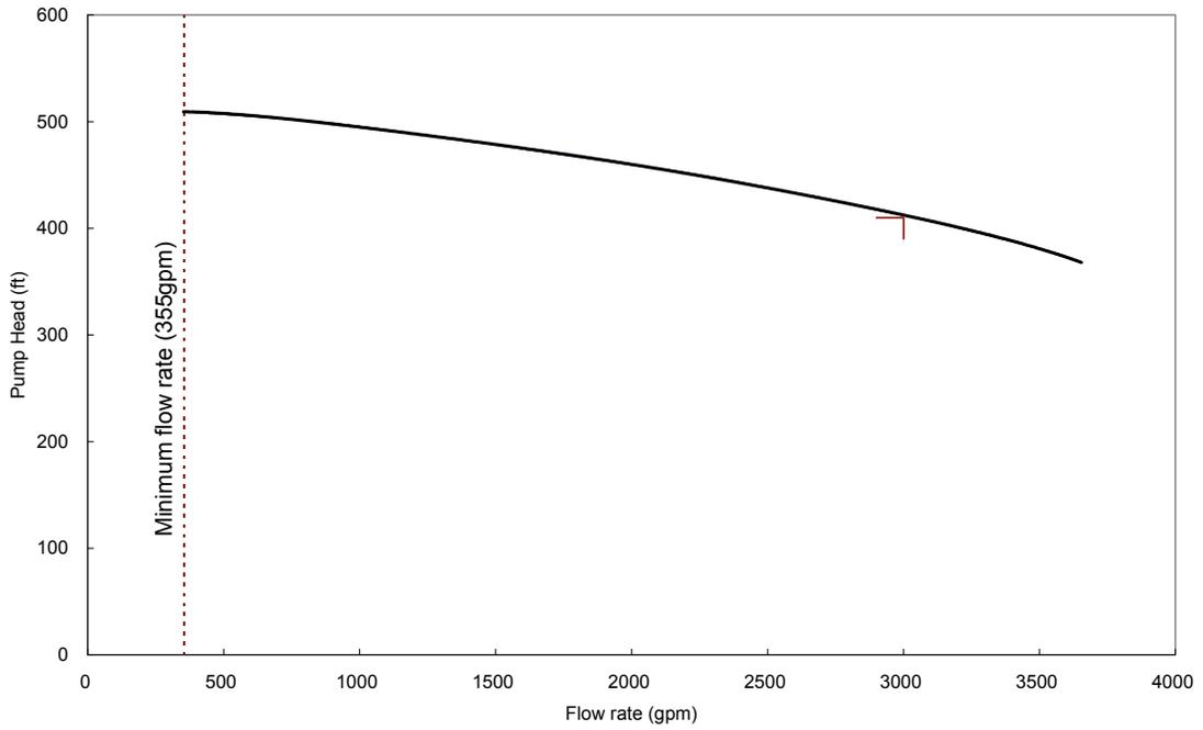
**Figure B-1 CS/RHR Pump Characteristic Curve**
