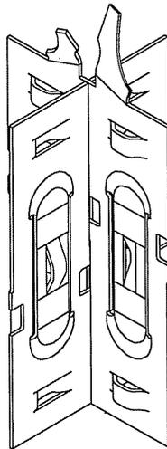
**Figure 4.2.1-1 Mitsubishi Grid Spacer (Z3 Type) Schematic View**
