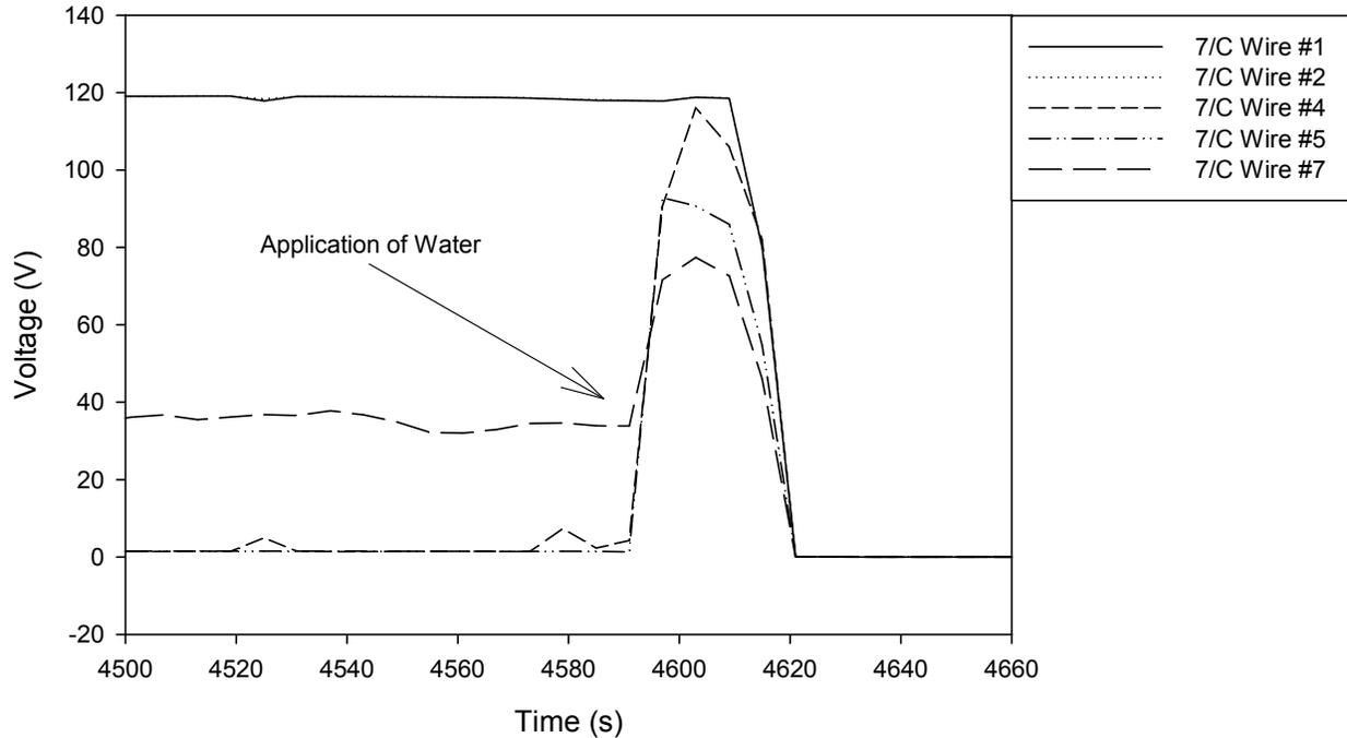
**Figure 2-30. EPRI/NEI Test 3 voltage plot - water spray**
