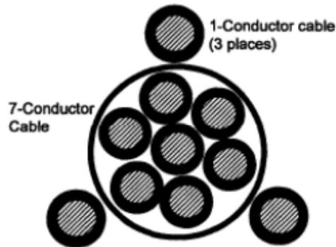
**Figure 3-3. EPRI/NEI cable configuration**
