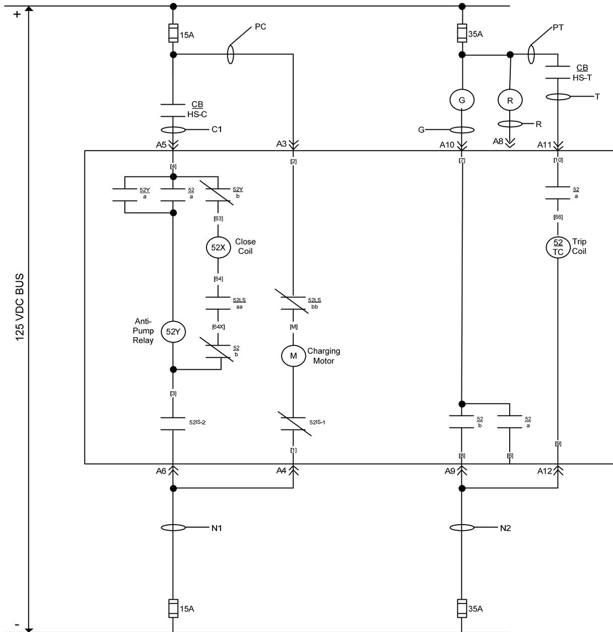
Figure 4-5. Line drawing for dc SWGR 1 circuit
