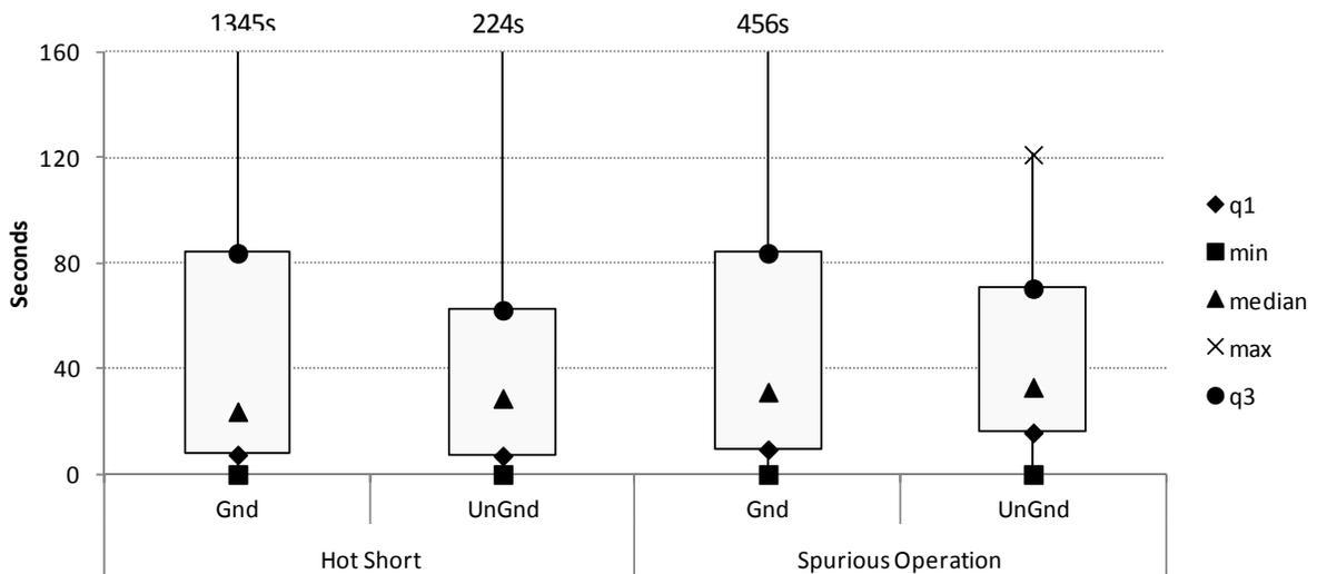
**Figure 2-25. Circuit grounding box plot, duration, ac tests**
