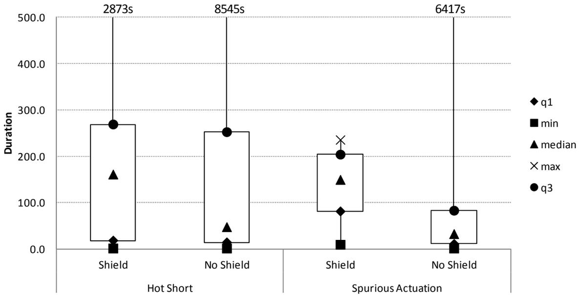
**Figure 4-34. Cable Shielding box plot, duration, dc tests**
