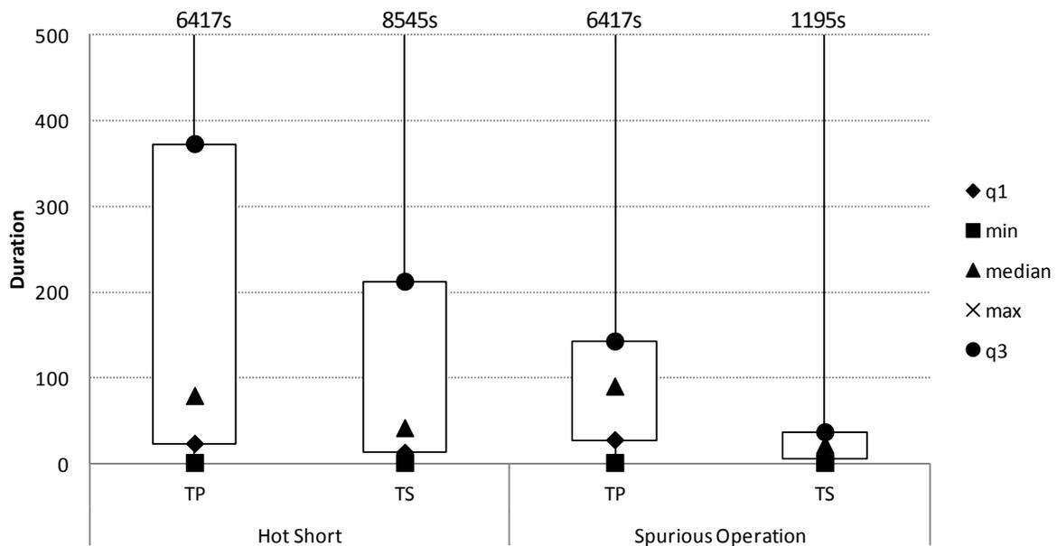
**Figure 4-20. Insulation type box plot, duration, dc tests**
