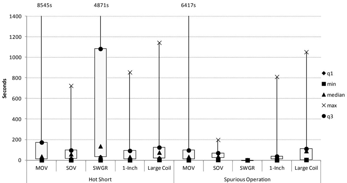
**Figure 4-30. Circuit type box plot, duration, dc tests**
