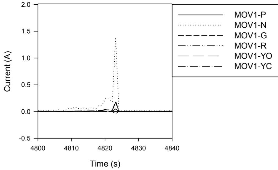
**Figure A-20. Penlight MOV-1 Test #49 current plot**
