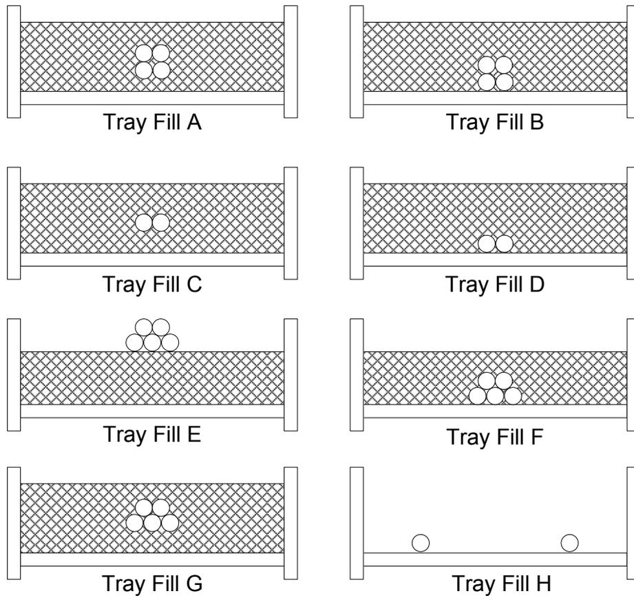
**Figure 4-14. Circuit cable orientation for filled trays**
