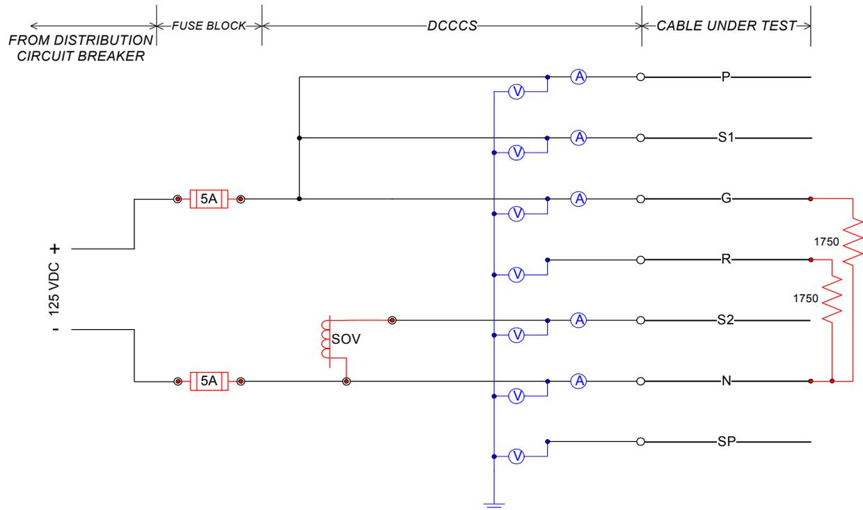
Figure 4-4. Line drawing for dc SOV circuit
