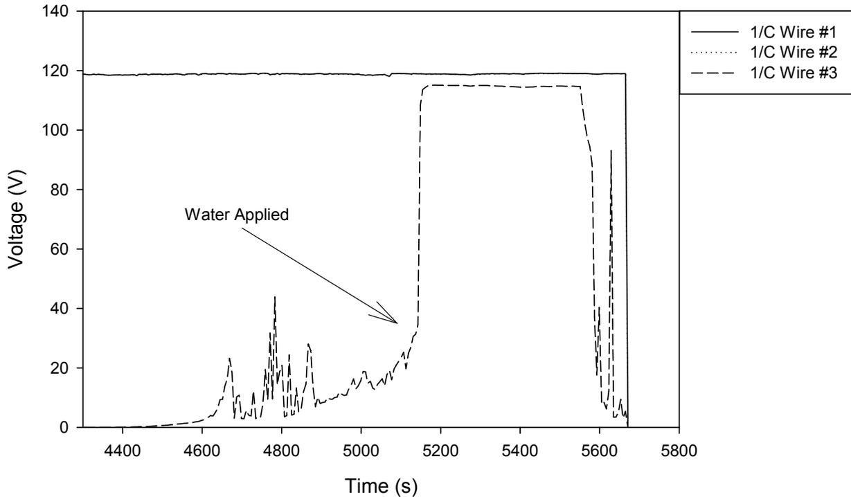
**Figure 2-31. EPRI/NEI Test 10 voltage response following water spray**
