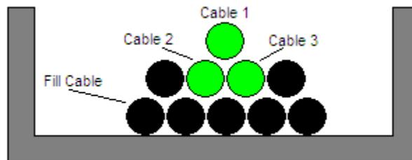
**Figure 3-1. EPRI/NEI inter-cable test tray fill**
