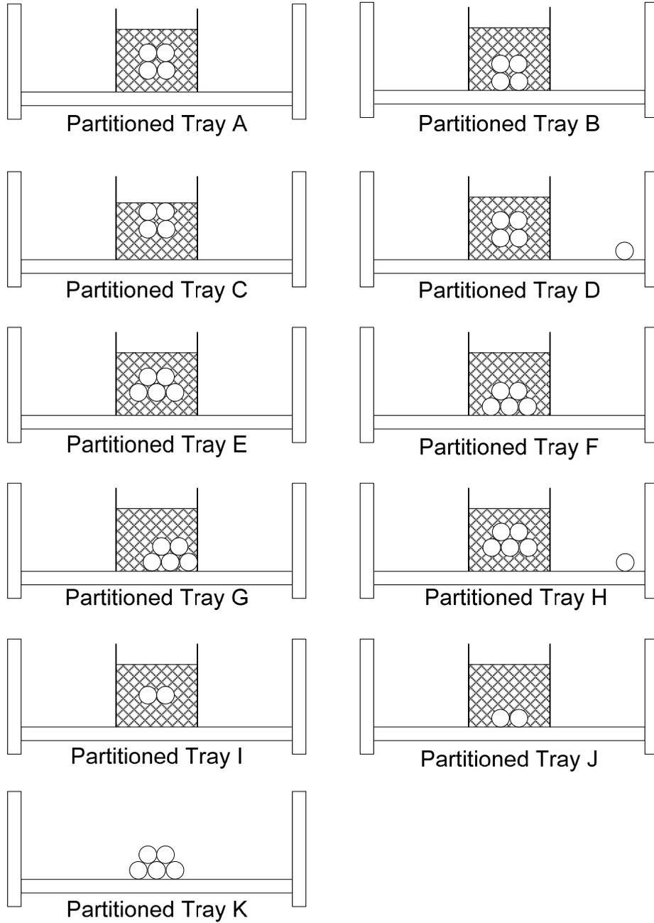
**Figure 4-15. Circuit cable orientation for partitioned trays**
