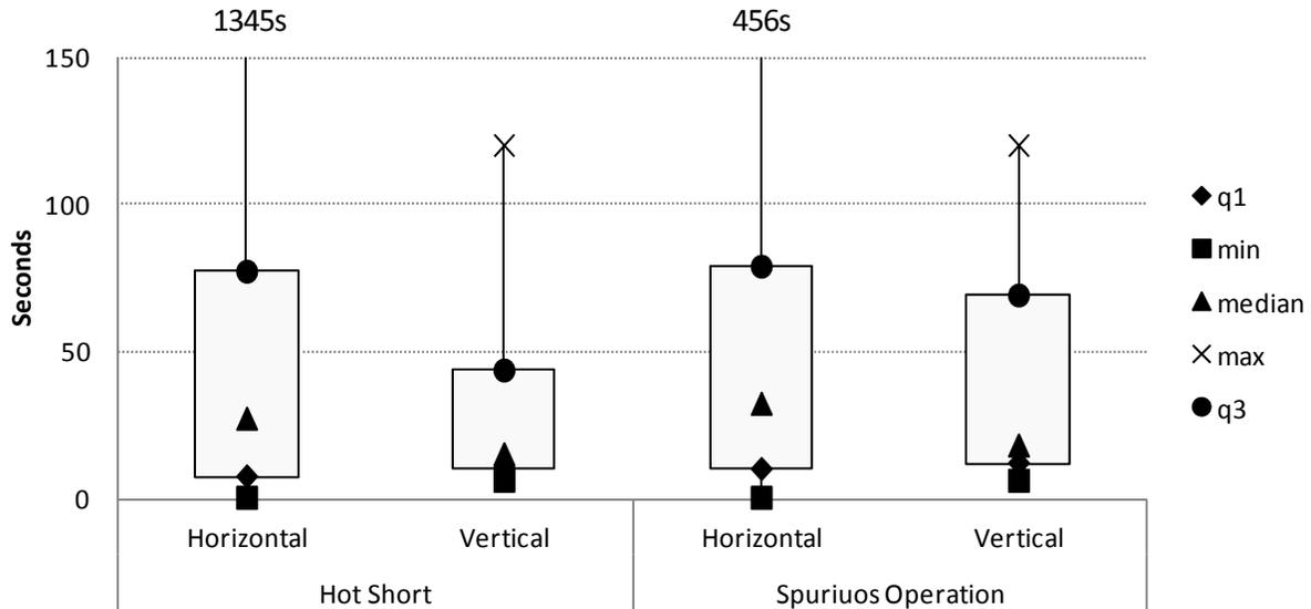
**Figure 2-8. Cable orientation box plot, duration, ac tests**
