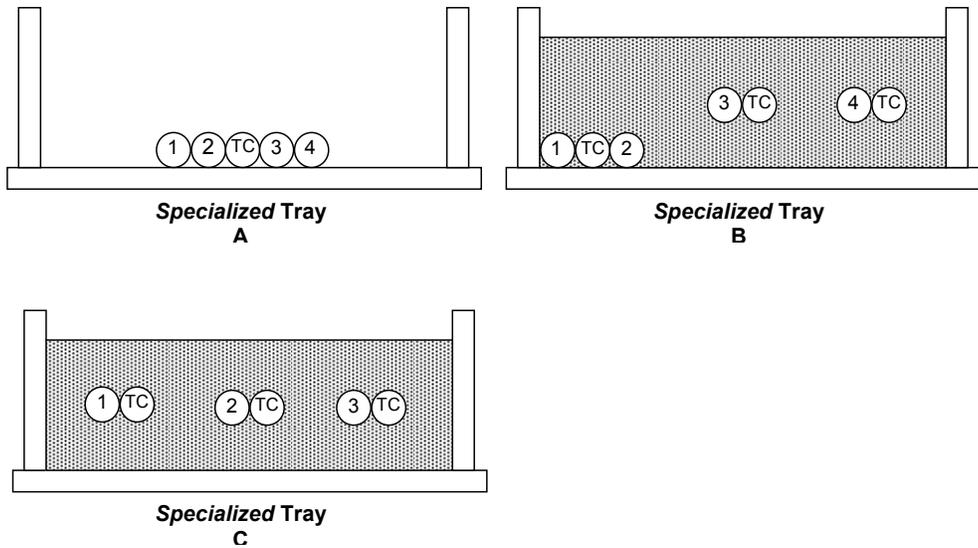
**Figure 4-16. Circuit cable orientation for specialized trays**
