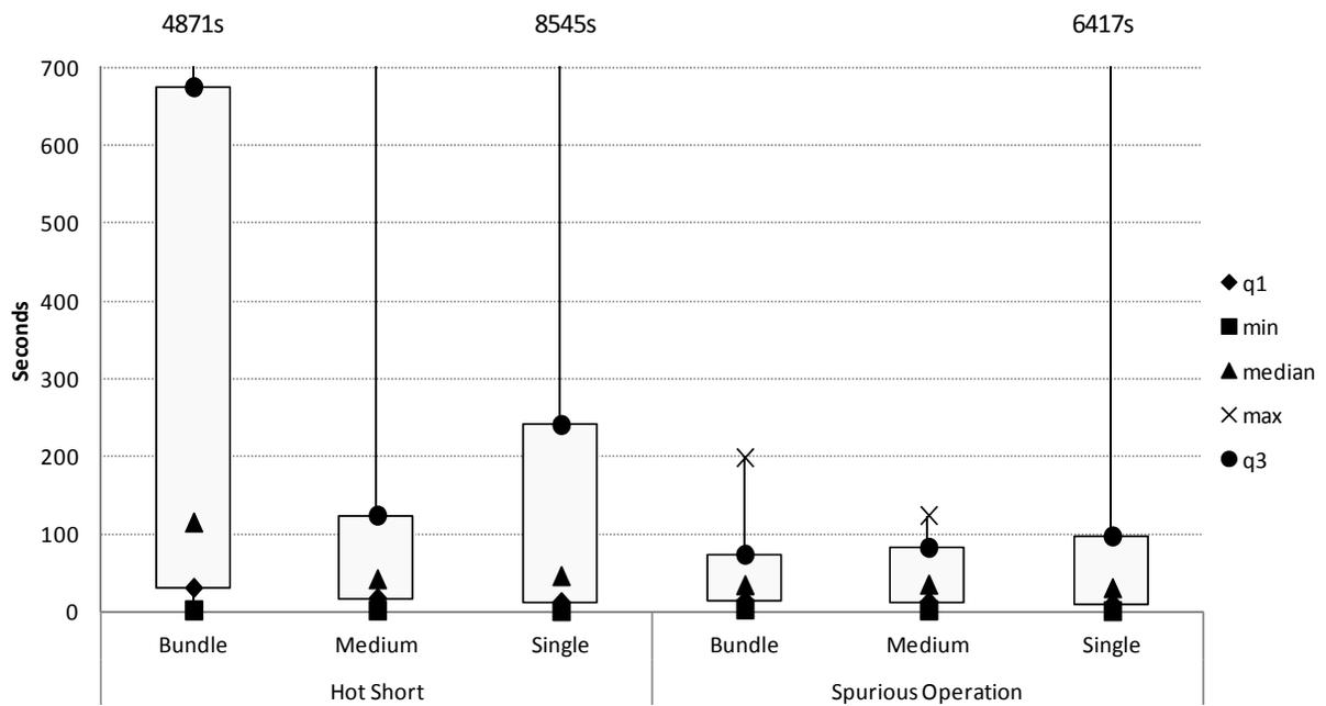
**Figure 4-18. Raceway fill box plot, duration, dc tests**
