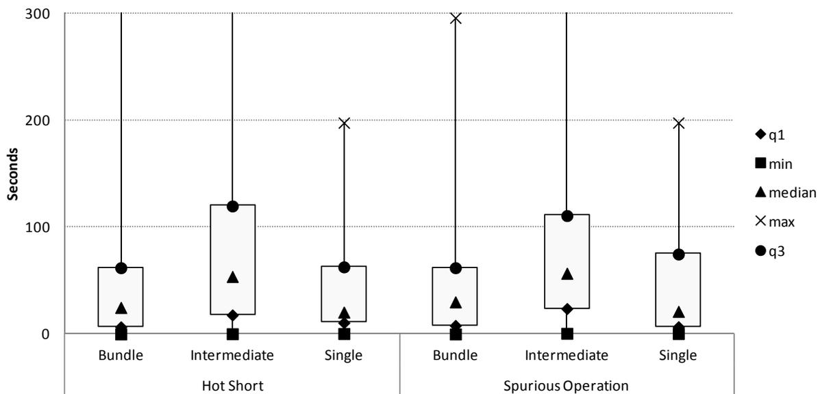
**Figure 2-15. Raceway fill box plot, duration, ac tests**
