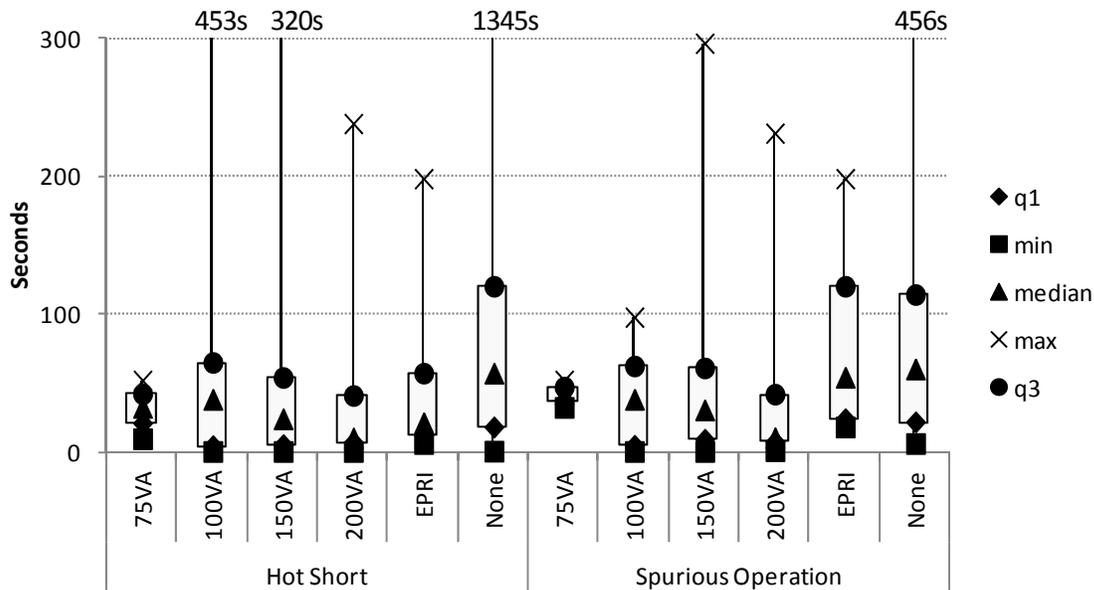
**Figure 2-23. CPT size box plot, duration, ac tests**
