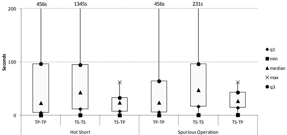
**Figure 2-21. Insulation-Jacket type box plot, duration, ac tests**
