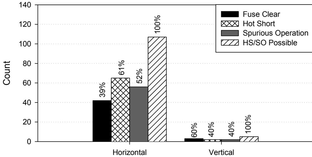
**Figure 2-7. Cable orientation, global approach, ac tests**
