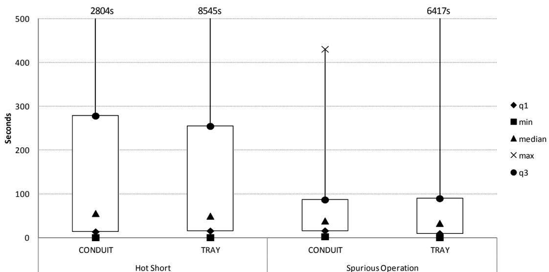
**Figure 4-12. Raceway routing box plot, duration, dc tests**
