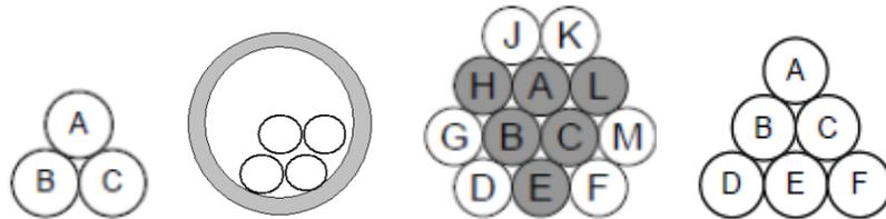
Figure 2-11. Cable bundle arrangements (3-, 4-, 6-, & 12-cable bundles)
