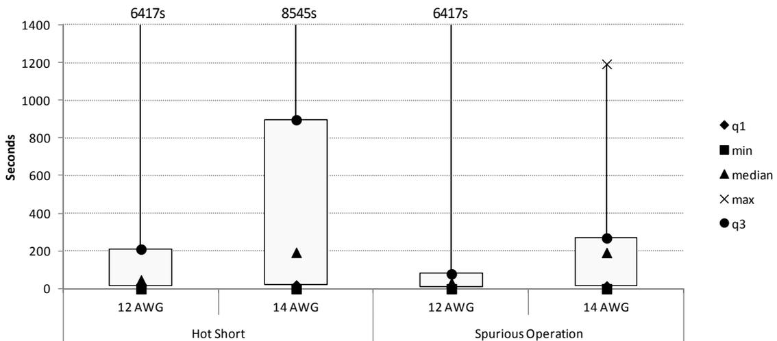
**Figure 4-28. Conductor size box plot, duration, dc tests**
