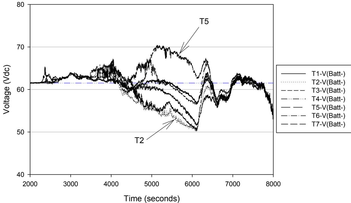
**Figure 5-2. DESIREE-FIRE inter-cable test results penlight #47**
