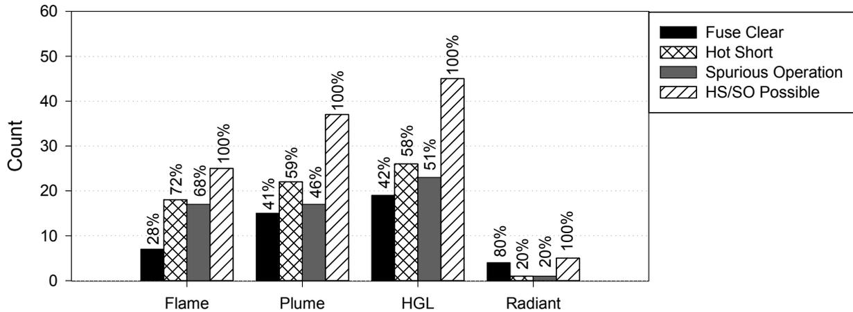
**Figure 2-5. Thermal exposure conditions, global approach, ac tests**
