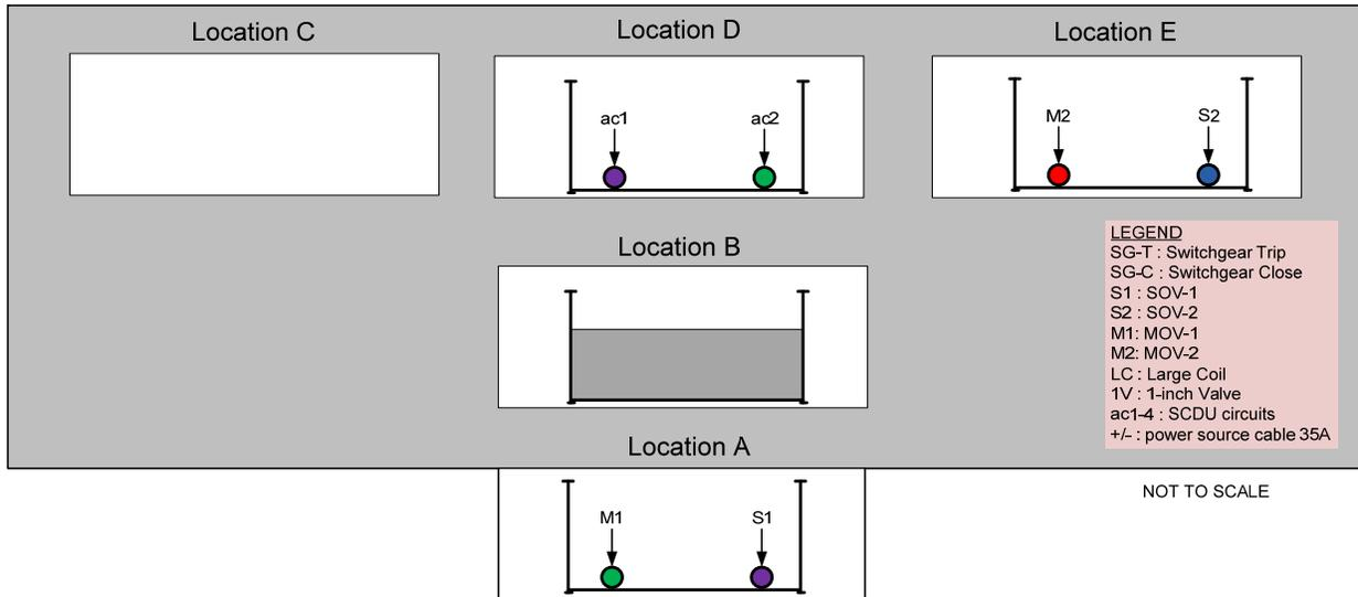
Figure 5-6. Intermediate-scale test preliminary 2 cable loading configuration
