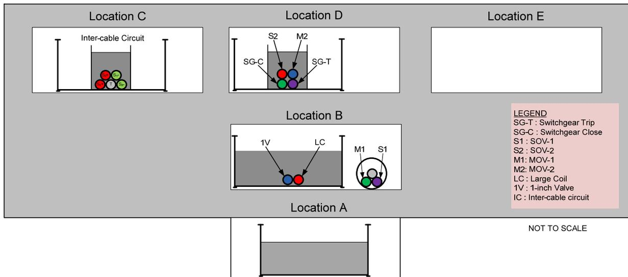
Figure 5-8. Intermediate-scale test 1 cable loading configuration
