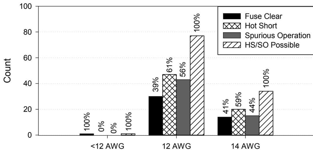
**Figure 2-28. Conductor size, global approach, ac tests**
