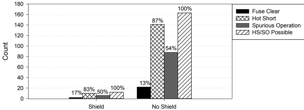
**Figure 4-33. Cable shielding, global approach, dc tests**
