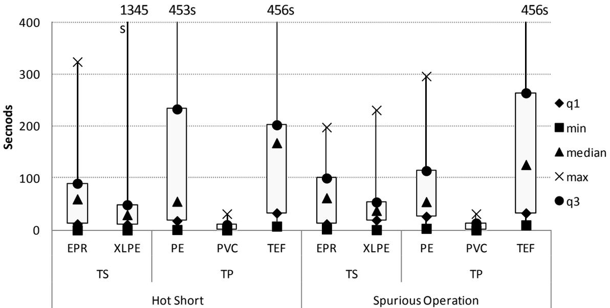
**Figure 2-19. Insulation material box plot, duration, ac tests**
