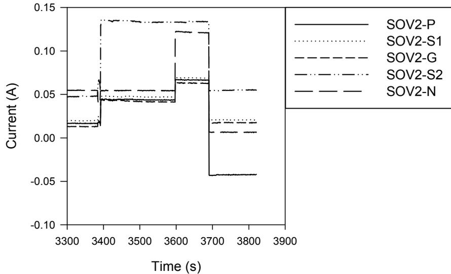
**Figure A-33. Penlight SOV-2 Test #28 current plot**
