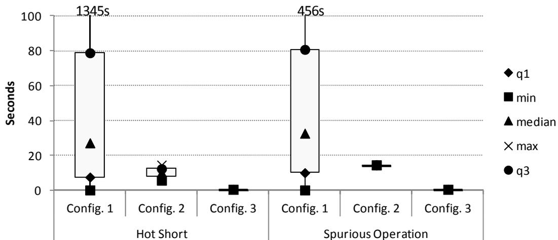
**Figure 2-27. Wiring configuration box plot, duration, ac tests**
