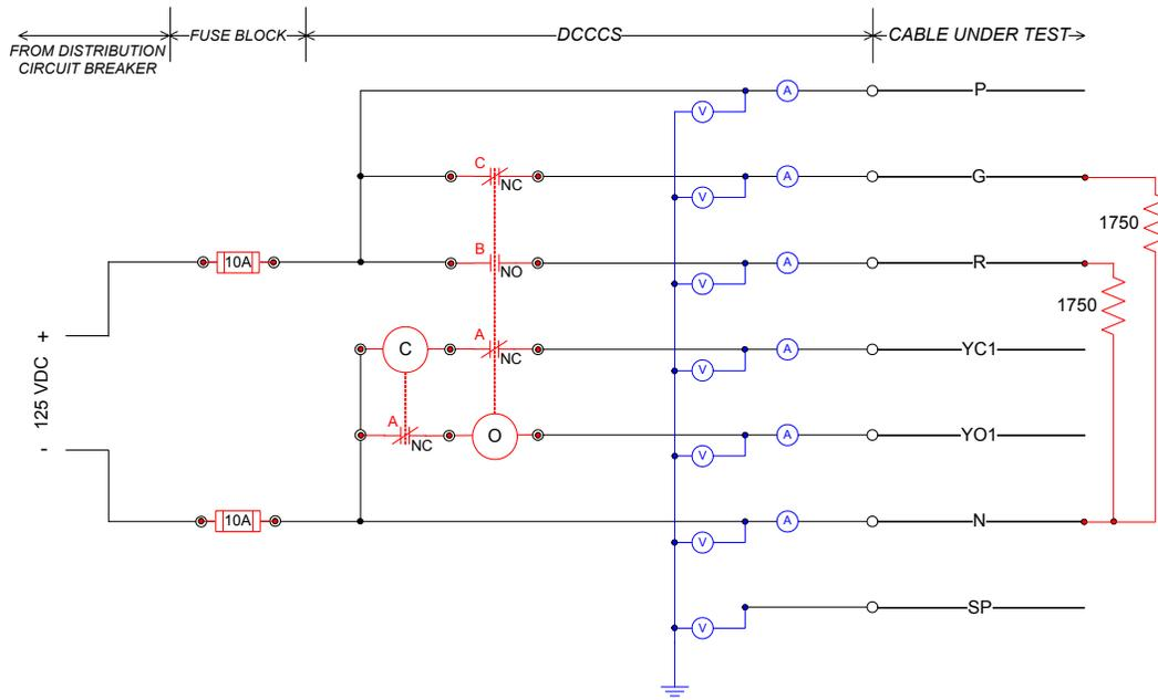
Figure 4-3. Line drawing for dc MOV circuit
