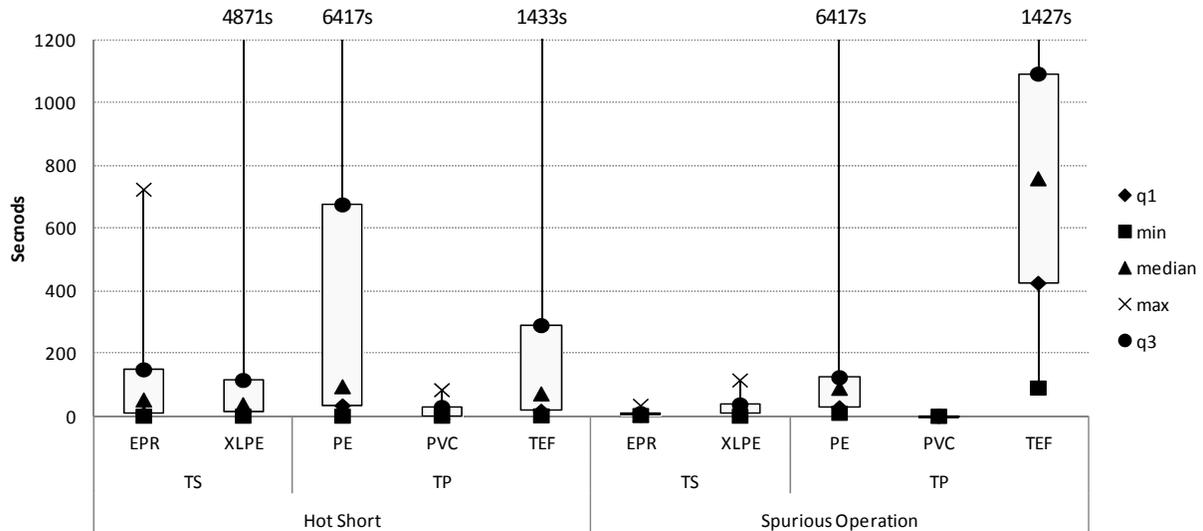
**Figure 4-22. Insulation material box plot, duration, dc tests**
