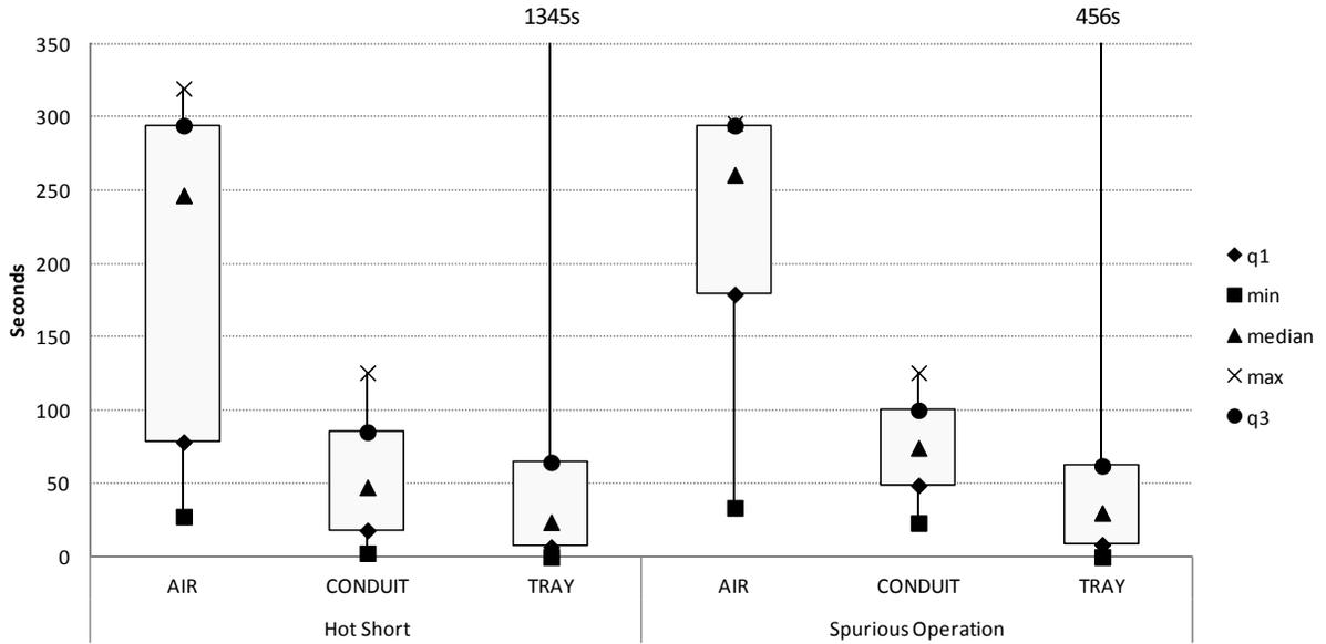
Figure 2-10. Raceway routing box plot, duration, ac tests
