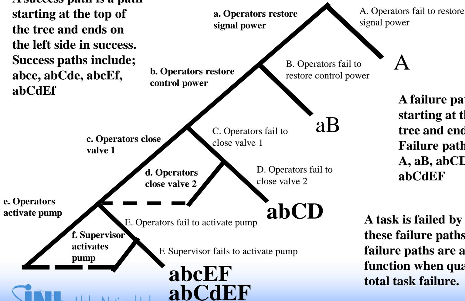
A failure path is a path starting at the top of the tree and ends in failure. Failure paths include; A, aB, abCD, abcEF, abCdeF
