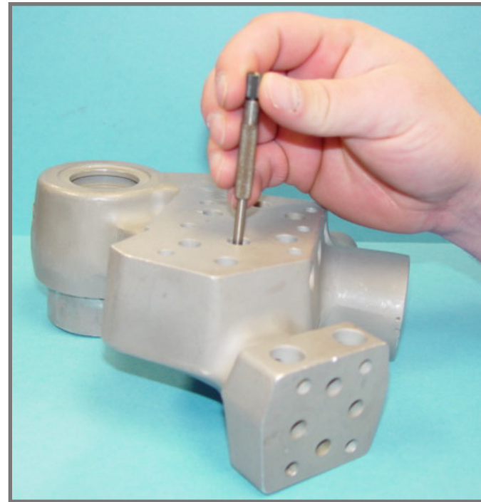
Small hole gauge used in determining hole diameter
