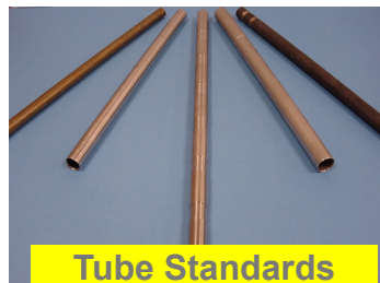
EDM Notches (Crack Simulation)
