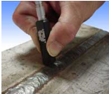
Conventional Probe and Crack Indication
