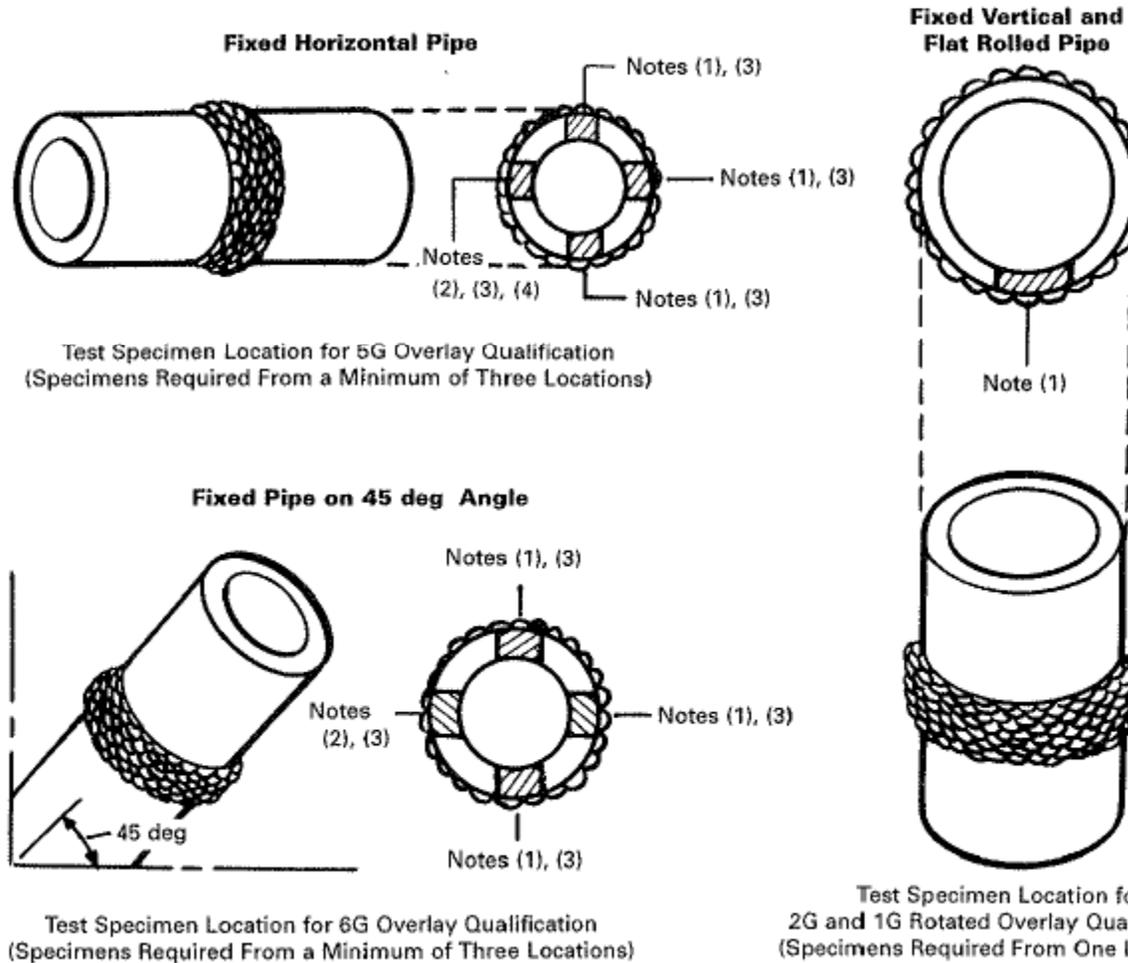
Test Specimen Location for 5G Overlay Qualification (Specimens Required From a Minimum of Three Locations)
