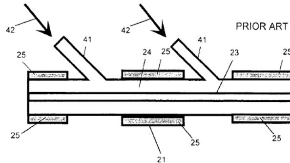
**Multiple 1kW single mode fibers interfaced to a larger multi-mode fiber by a patented technique**
