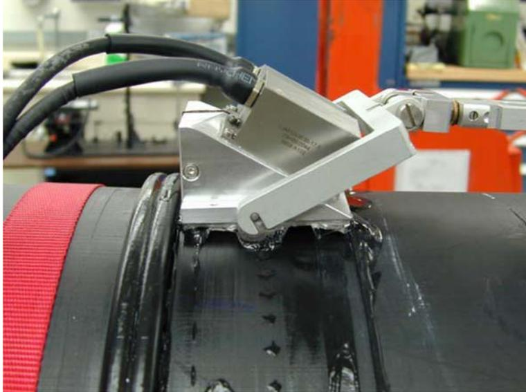
**Figure 3.20 Gel Wedge in an Aluminum Frame for the 1.5-MHz PA Probe**
