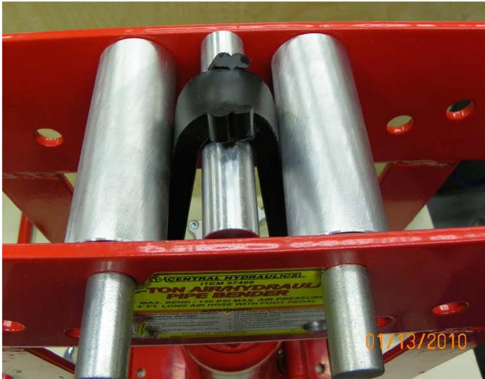
Figure 4.21 Side-Bend Test Apparatus (top) with an HDPE Test Specimen from Pipe 1224 Undergoing Testing (bottom) – Example of a Dark Green SBT Result
