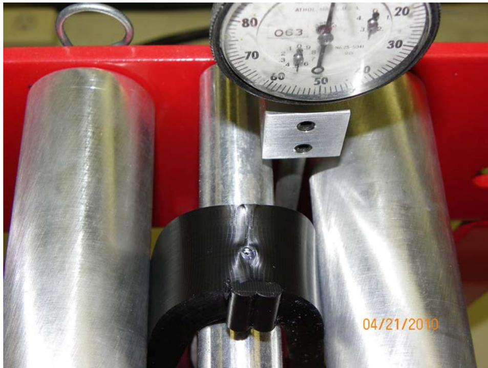
**Figure 4.22 Another HDPE Specimen Undergoing Side-Bend Testing Showing the Dial Indicator Used to Track Travel of the Ram Which, in This Case, is Showing the Maximum Travel of 2.5 Inches (63.5 mm) as Shown by the Upper Right and Lower Left Dials. This is an example of a light green SBT result.**
