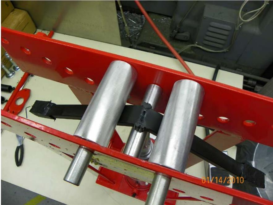
**Figure 4.23 Specimen from Pipe 126 Part Way Through the Side-Bend Test Showing the Early Stages of Failure**
