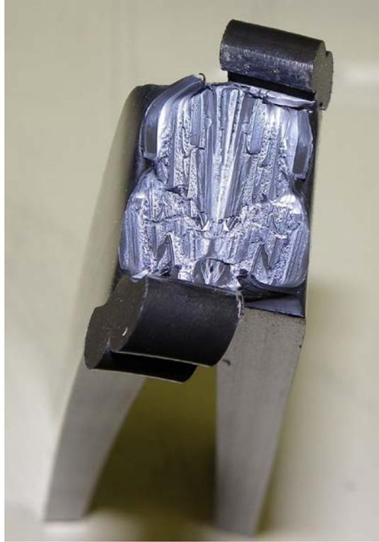
**Figure 4.25 Sample from Pipe 1224 Failed the SBT and Was Removed Adjacent to the Specimen Shown in Figure 4.21, Which Did Not Fail – Example of a Red SBT Result**
