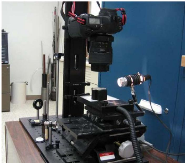
**Figure 4.3 Setup for Photographing the Bulk Specimen**
