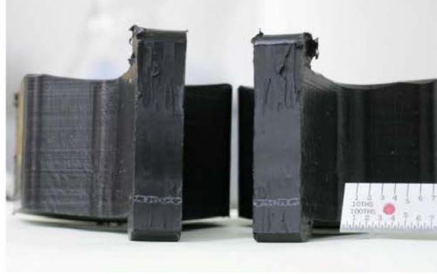
**Figure 4.17** Coupon 4 from Pipe 126 Quadrant 4, Fused with Fusion Pressure During the Heat Cycle and a 20-sec Open/Close Time. The failure mode is brittle but shows some tearing at the top (ID) in the right figure. PNNL called this area good and the Fluor call was on the edge of a good-to-bad region.
