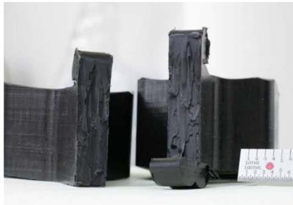
**Figure 4.18** Coupon 5 from Pipe 1224 Quadrant 2, Fused with Procedure F2620 and Expected to be Good. The failure mode was brittle at the joint but shows some ductility. Both PNNL and Fluor called this area good.
