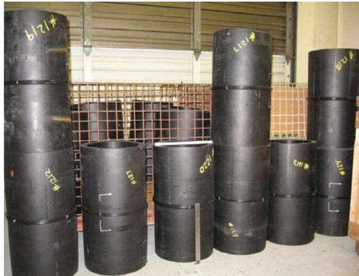
**Figure 2.1** Several of the Butt Welded 3408 Pipes are shown with 12-in. (30.5-cm) Scales on the Center Pipe, One in the Horizontal Direction and One in the Vertical. The pipe assemblies are approximately 2 ft (61 cm) long.
