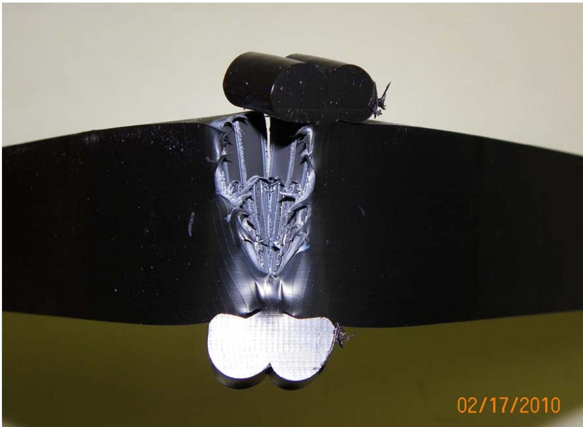
**Figure 4.26 Example Where Only One Ligament Remained at Location +12 on Pipe 1224 – Example of a Yellow SBT Result**
