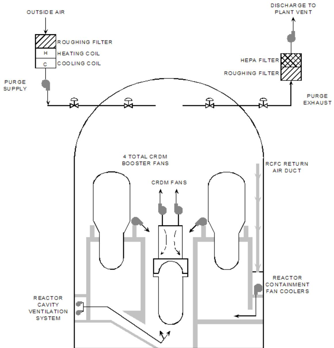
Figure 1.7-1 PWR Containment Ventilation System
