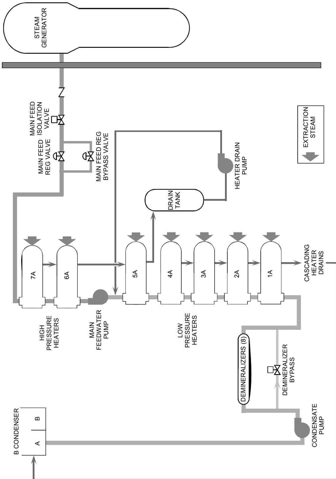
Figure 1.8-1 PWR Condensate and Feedwater System
