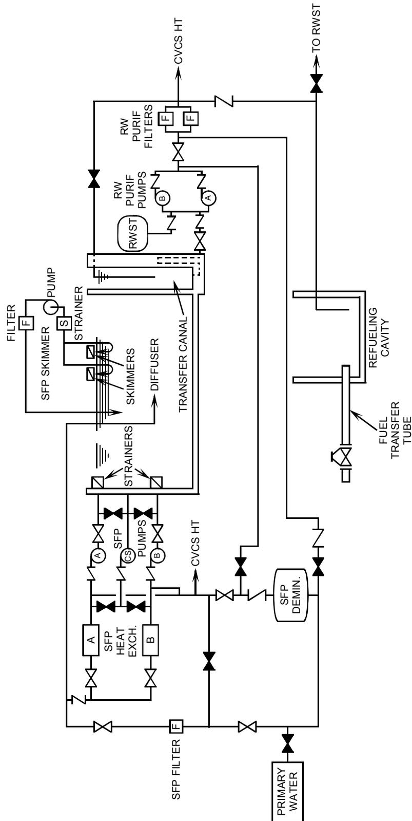
Figure 1.8-2 PWR Spent Fuel Pool Cooling System
