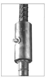
• By means of an exothermic process, molten filler solidifies around the deformations on the bar and internal grooves of the sleeve, creating a mechanical interlock; good also in tension
