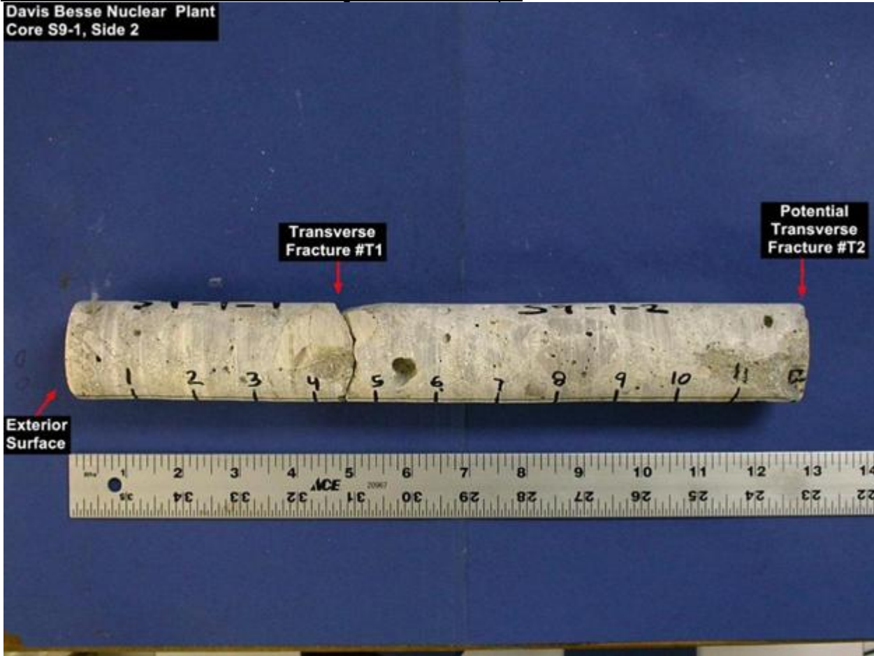
Picture No. 8 -Davis-Besse Shield Building - Core Bore Sample
