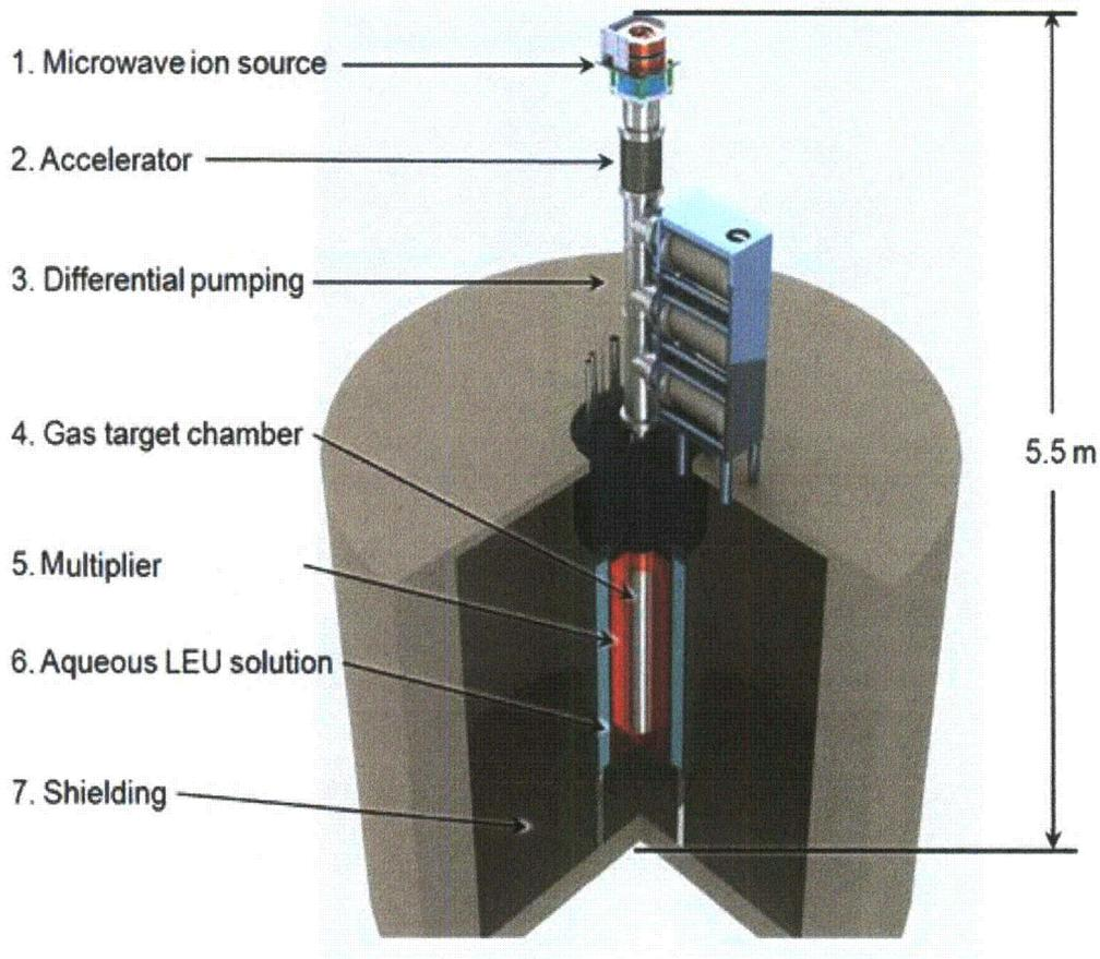
Figure 2 provides the process flow diagram for the SHINE production system.
