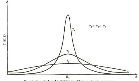
Doppler-broadening of a resonance with increasing temperature.
