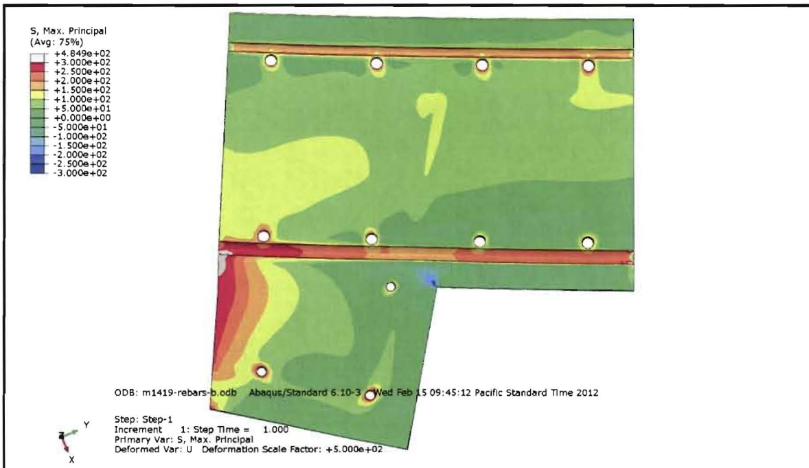
Figure 46: Max Principal Stress (psi) in the [redacted] laced in the Shoulder 10 Location
