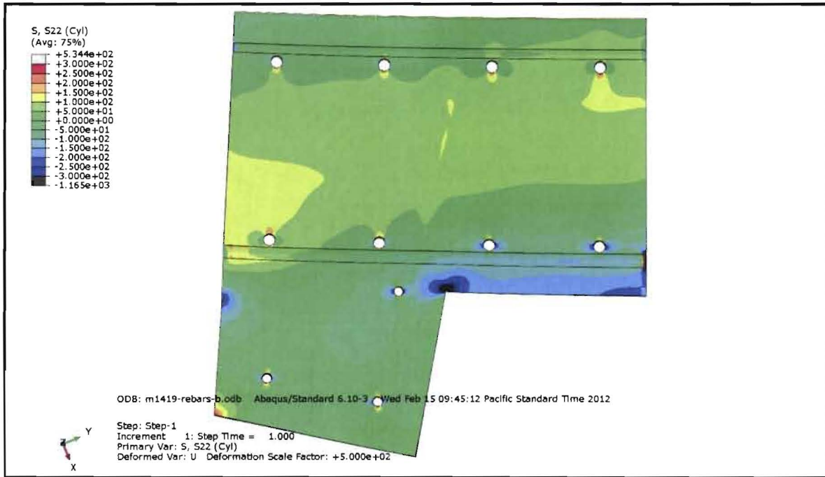
Figure 48: Hoop Stress (psi) in the [REDACTED] placed in the Shoulder 10 Location
