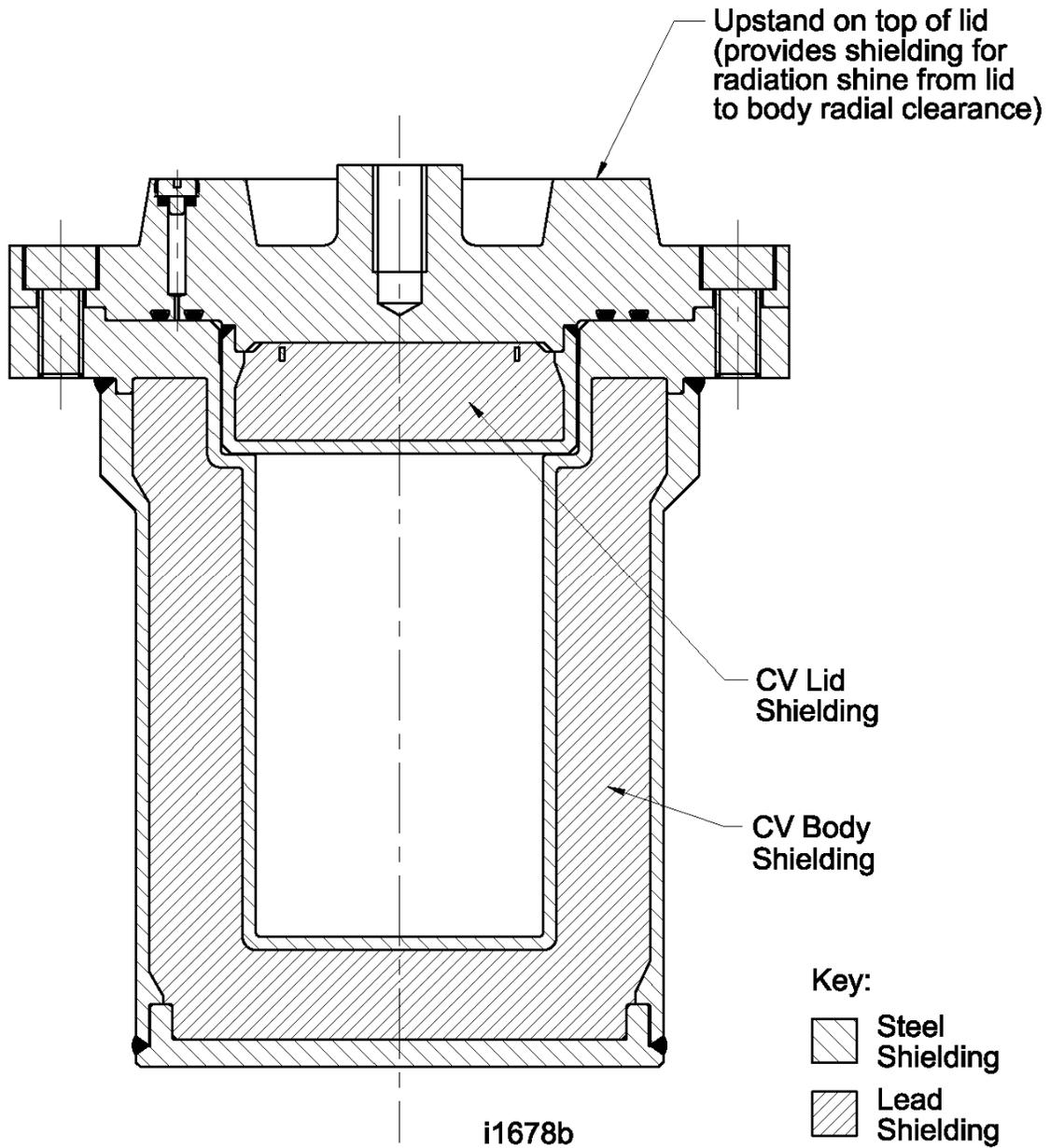
Figure 5-1 Gamma shielding present in the 3979A package
