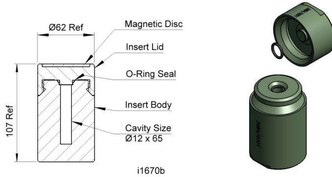
**Figure 1-5a Shielding insert LS-12x65-Tu – Design # 3984**
