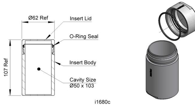
**Figure 1-5c Shielding insert LS-50x103-SS – Design # 3986**
