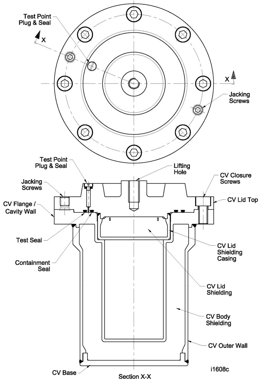
Figure 1-2a 3980 CV – Top and Section View and Nomenclature
