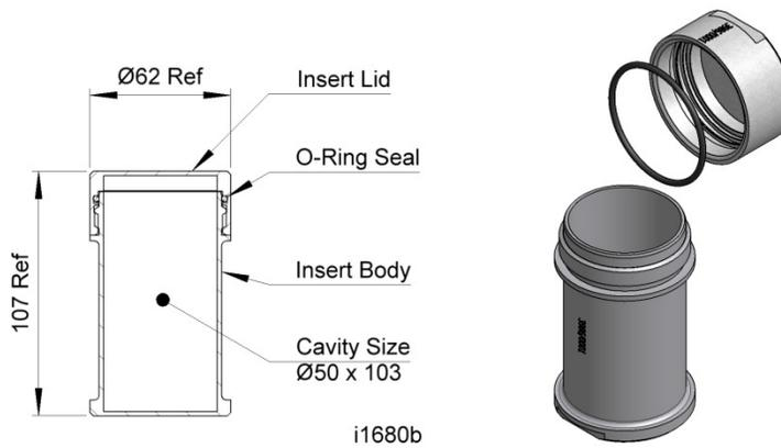
**Figure 5-2c Shielding insert LS-50x103-SS – Design # 3986**
