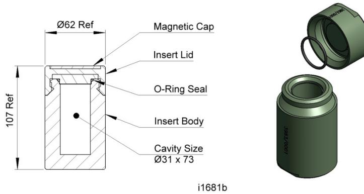
**Figure 1-5b Shielding insert LS-31x73-Tu – Design # 3983**
