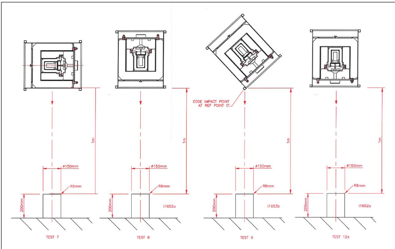
Figure 2-4 Puncture Tests Impact Orientations
