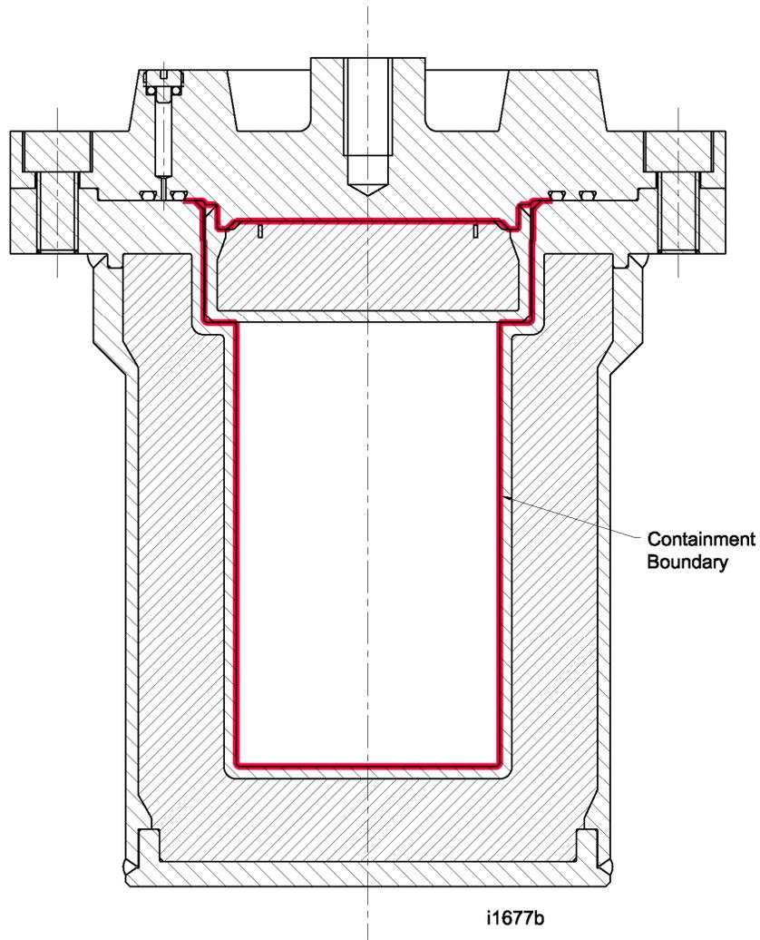
Figure 1-3 Containment boundary of the Safkeg-LS 3979A package
