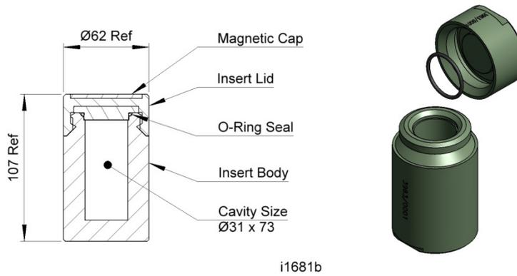
**Figure 5-2b Shielding insert LS-31x73-Tu – Design # 3983**
