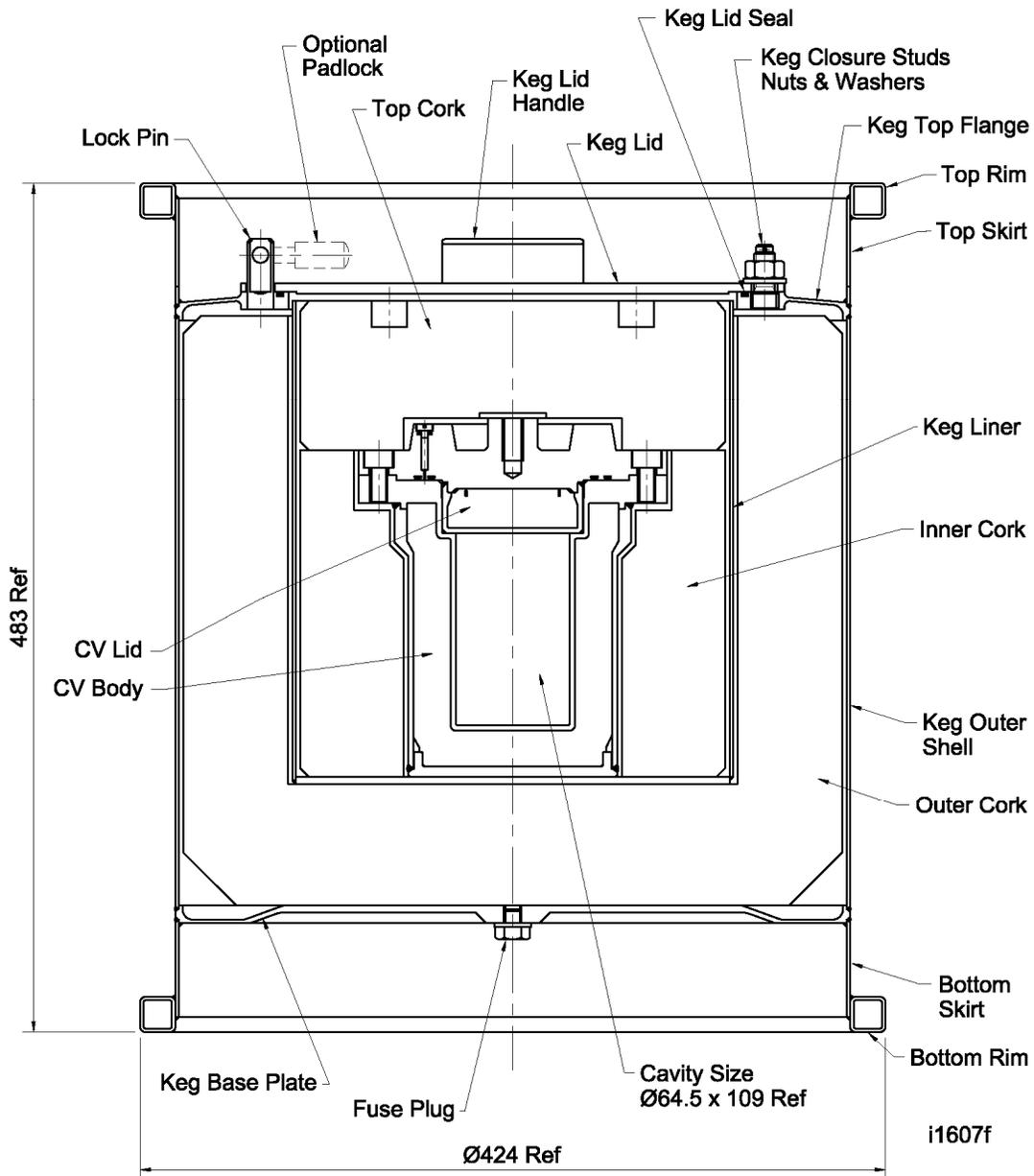
Figure 1-1a Safkeg-LS 3979A package – Section View and Nomenclature
