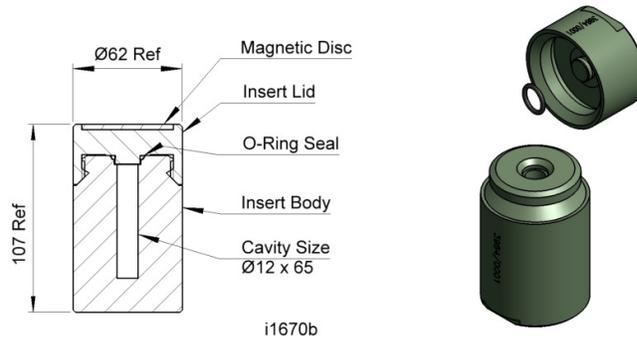
**Figure 5-2a Shielding insert LS-12x65-Tu – Design # 3984**
