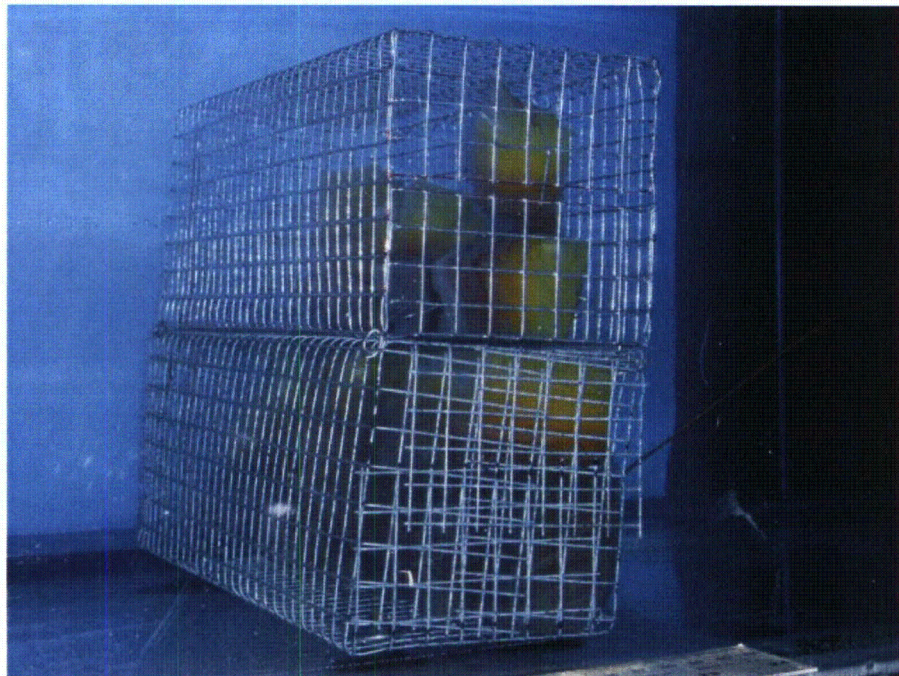
Figure 3e.1.5.1-4: Fiber Samples in Baskets in the Flume During a Test
