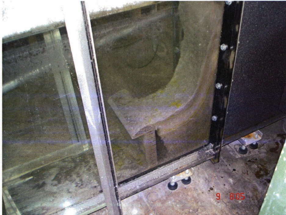
Figure 3f.4.2.3.4-2: Test 5 Non-Chemical Debris Bed on Front of Strainer
