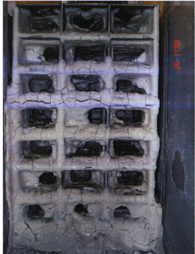
Figure 3f.4.2.3.5-5: Test 6 Debris Bed After All Chemical Portions During Draindown
