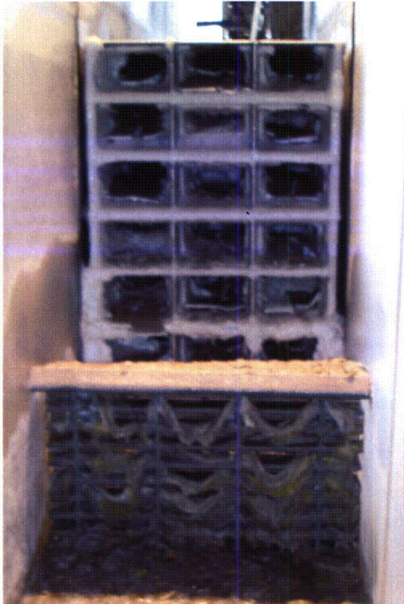
Figure 3f.4.2.3.5-4: Test 6 Debris Bed After All Chemical Portions During Draindown
