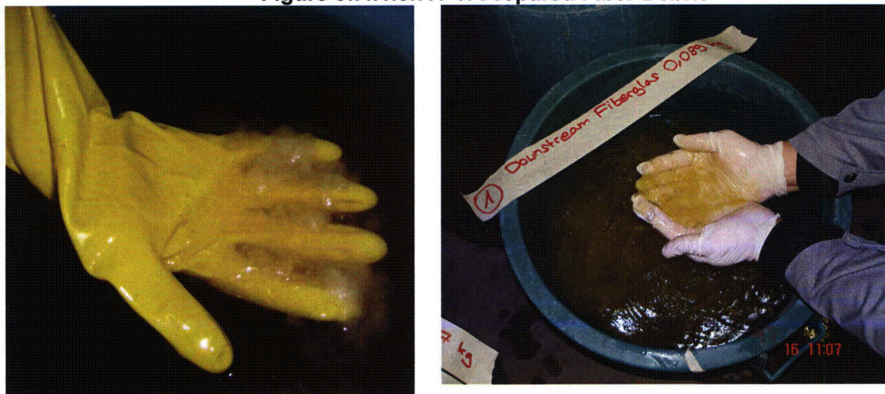
Figure 3f.4.1.5.7.1-1: Prepared Fiber Debris
