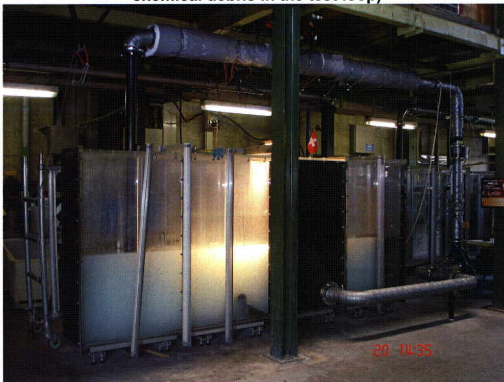
Figure 3f.4.1.5.1-1: Picture of CCI MFTL with the 2-Sided Test Module (with chemical debris in the test loop)
