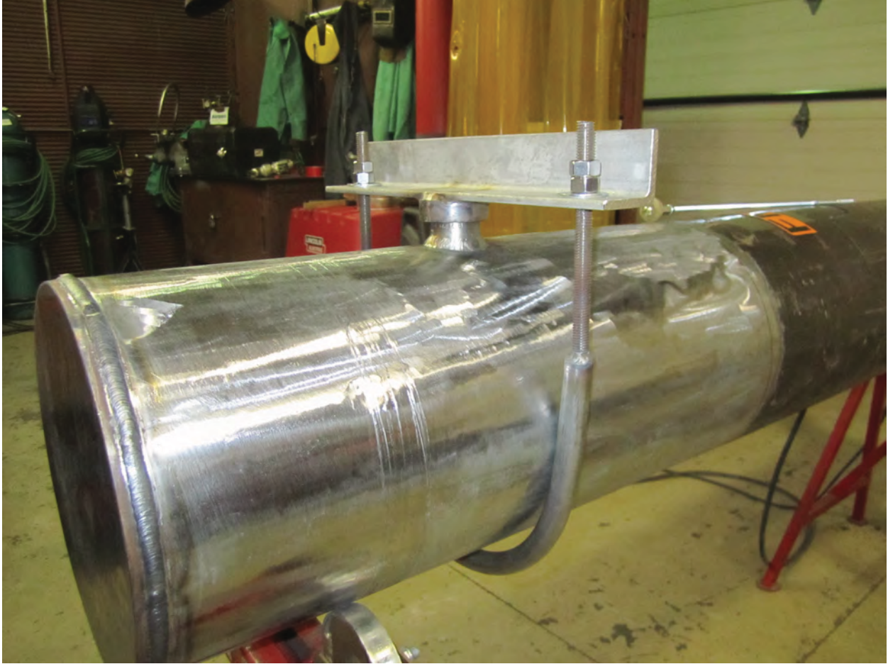
Figure 1: Temporary Plugging Device installed on fabrication shop mockup
