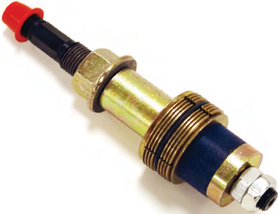
Figure 3: Example Alternate Temporary Plugging Device. Procured plugging device has solid shaft and stainless steel construction for wetted parts.
