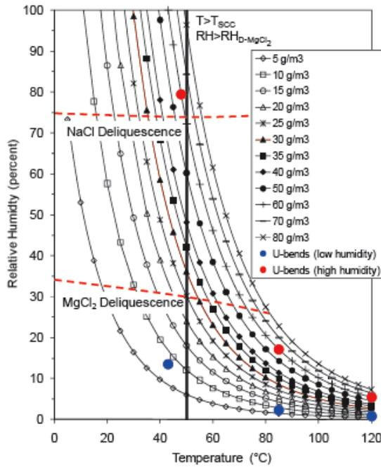
**Figure 43** Evolution of the Relative Humidity as a Function of Temperature Computed for Various Absolute Humidity Values. The Region Between the Red (Maximum Humidity) and Blue (Minimum Humidity) Symbols Indicate the Expected Environmental Conditions Near the U-Bend Surface in the Salt Fog Test
