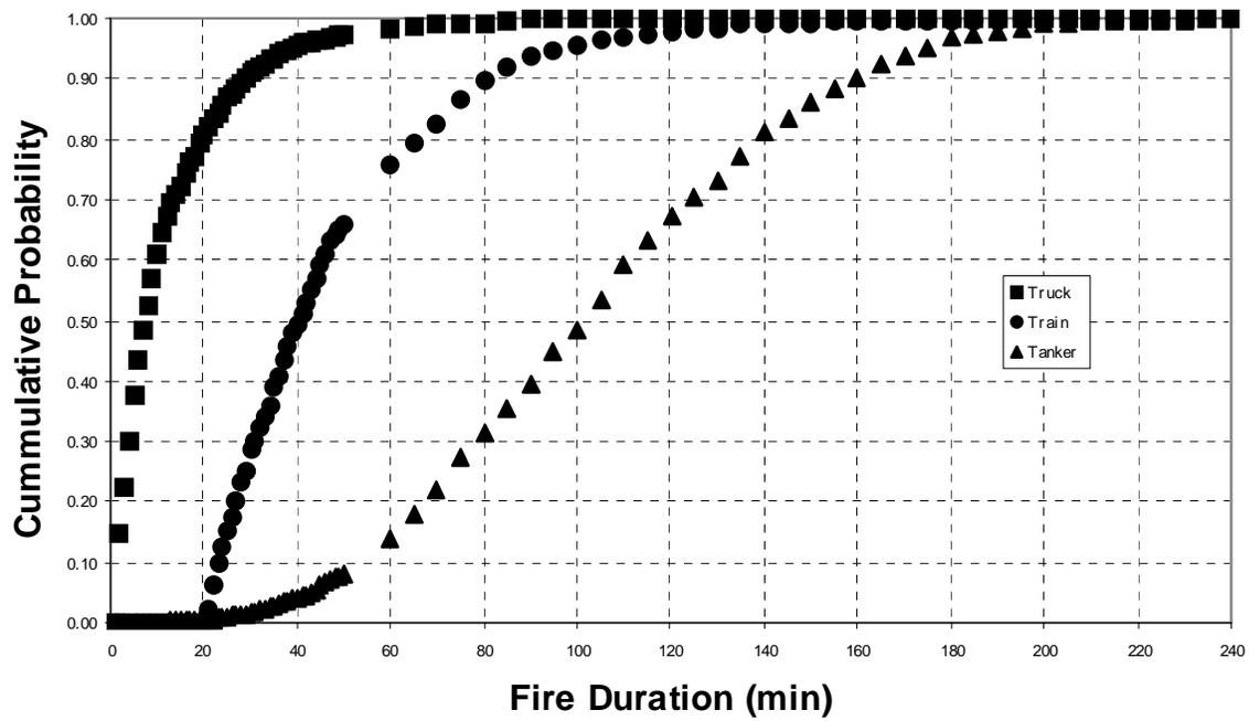
**Figure 8: Cumulative Fire Duration Distributions for Truck/Truck, Truck/Train, and Truck/Tanker Truck Fire Accidents**
