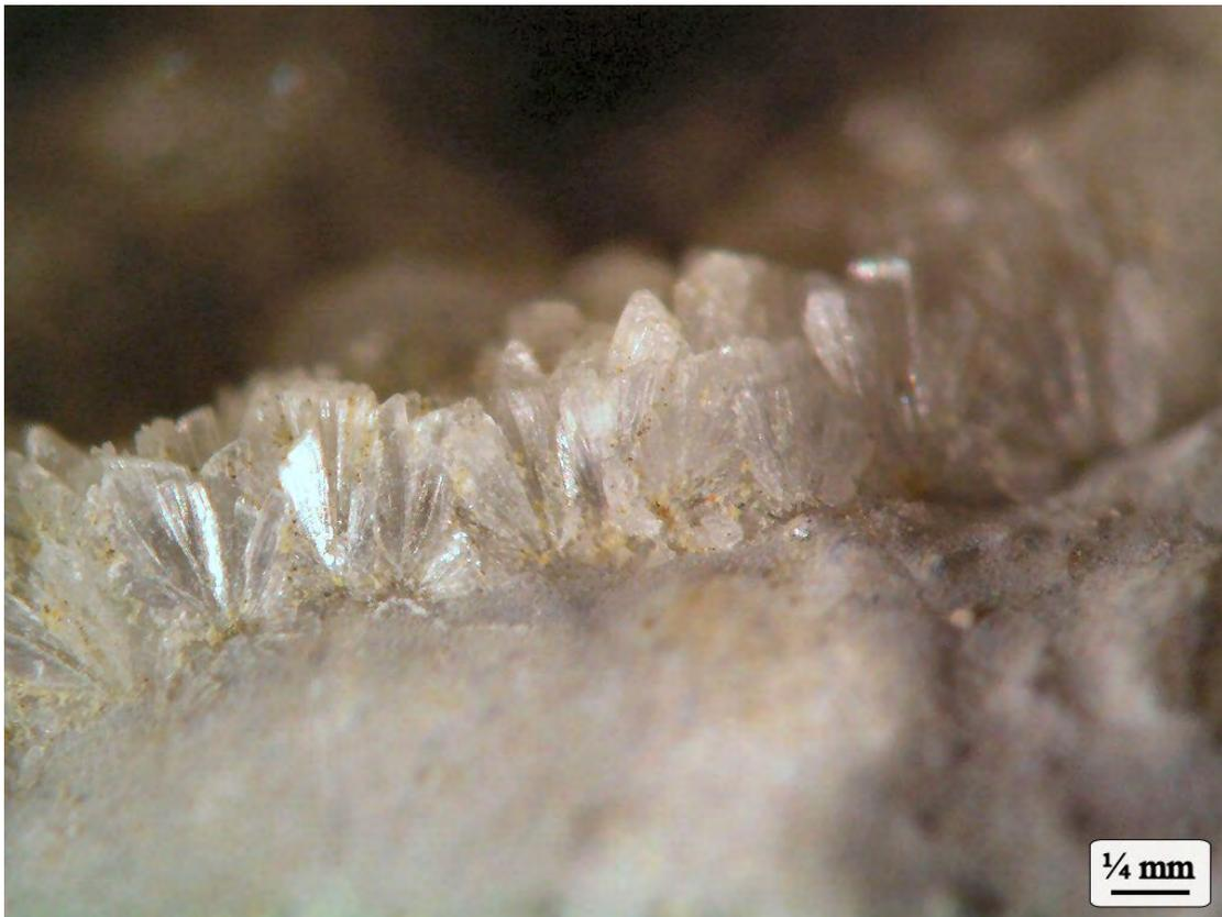
**Figure 10. Surface photographs taken under the microscope showing the boric acid crystals present within a surface void of Specimen No. 31.**
