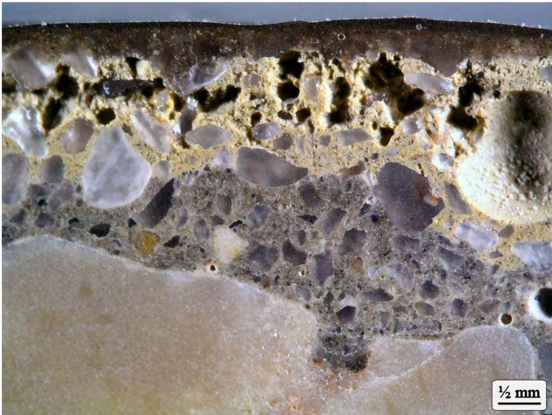
**Figure 2. Cross-section photographs taken under the microscope showing the acid attacked cement paste of Specimen No. 18. The upper dark portion of the cement paste has been penetrated by the epoxy coating.**
