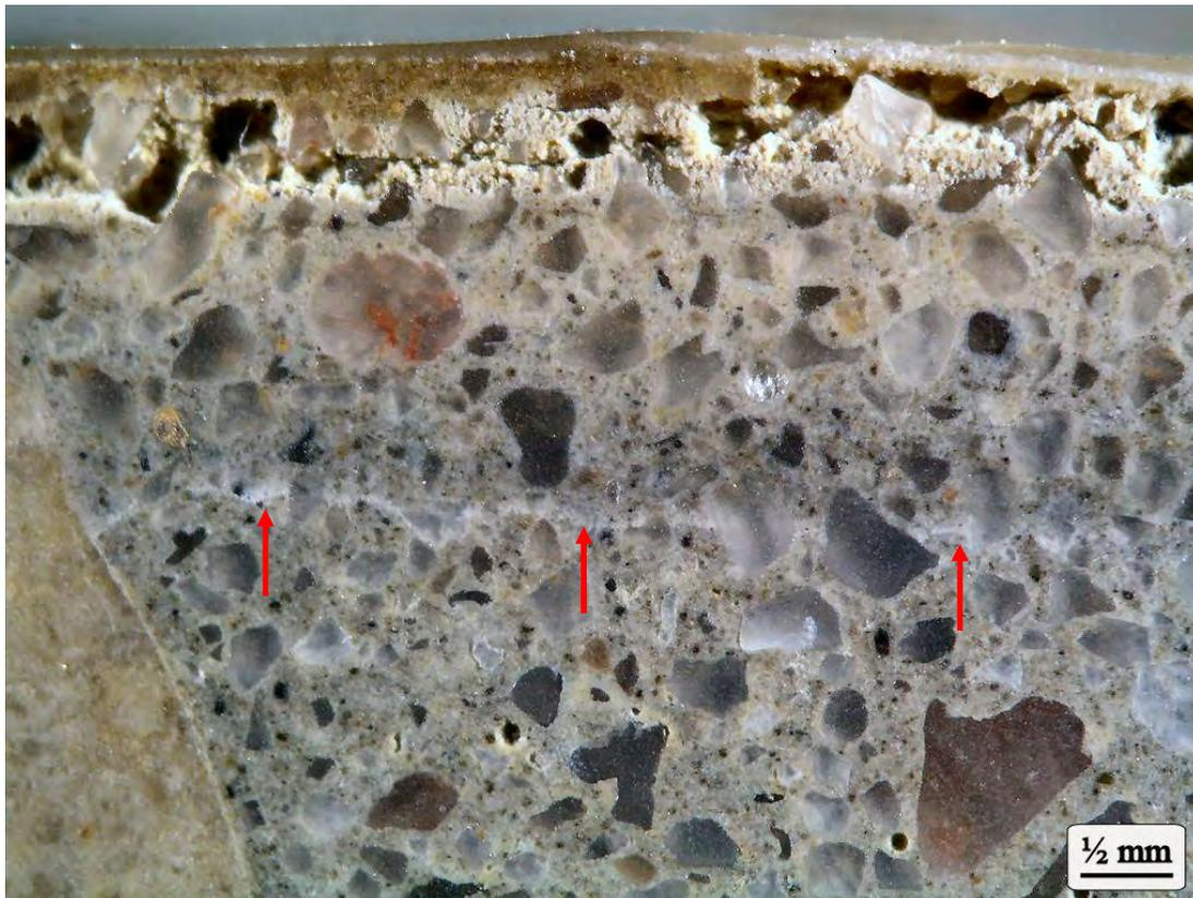
**Figure 4. Cross-section photographs taken under the microscope showing the acid attacked cement paste of Specimen No. 36. The upper dark portion of the cement paste has been penetrated by the epoxy coating. The thin white layer of cement paste is shown by the arrows.**
