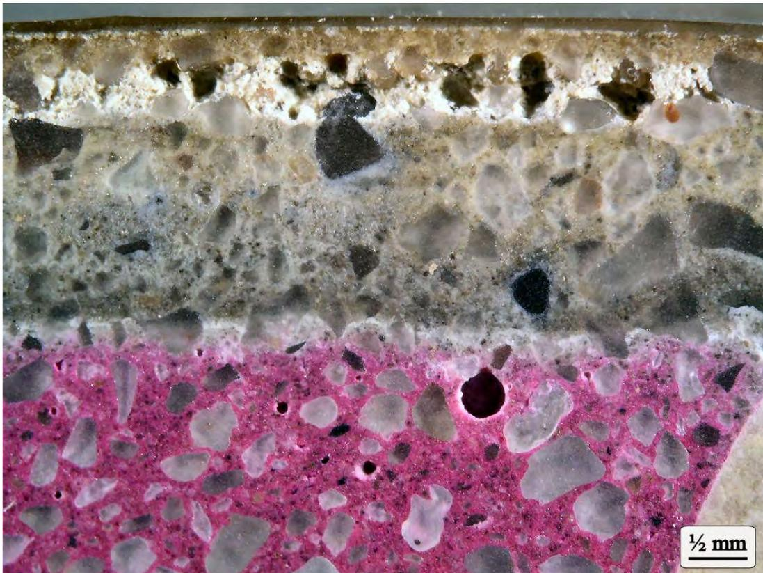
**Figure 6.** Cross-section photographs of Specimen No. 36 following the exposure to phenolphthalein solution. The depth to which the pH has been lowered by the acid exposure is represented by the uncolored cement paste.
