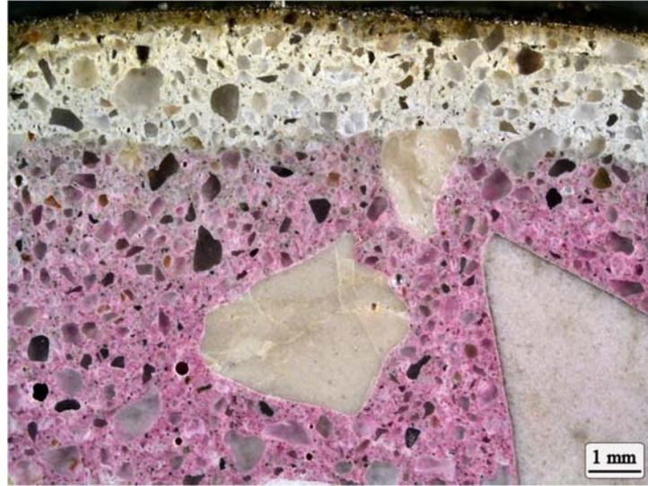
**Figure 5-5. Cross Section Photomicrograph of Saw-Cut, Lapped Concrete Specimen After Exposure to Phenolphthalein Solution. The Depth to Which the pH Has Been Lowered by Acid Exposure Is Represented by the Uncolored Cement Paste. [1 mm = 0.039 in]**
