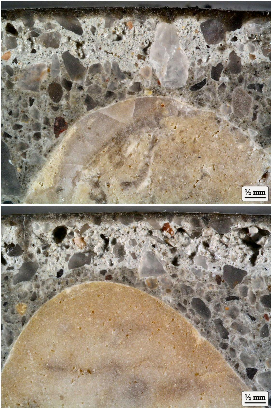
**Figure 2. Cross-section photographs taken under the microscope showing the acid attacked cement paste of Specimen No. 16. The layer of penetrated epoxy can be seen in both photographs.**
