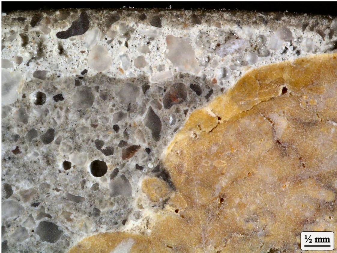
**Figure 3. Cross-section photographs taken under the microscope showing the acid attacked cement paste of Specimen No. 20. The layer of penetrated epoxy can be seen in both photographs.**
