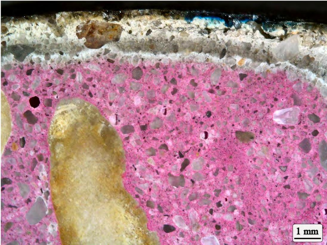
**Figure 8.** Cross-section photographs of Specimen No. 31 following the exposure to phenolphthalein solution. The depth to which the pH has been lowered by the acid exposure is represented by the uncolored cement paste.
