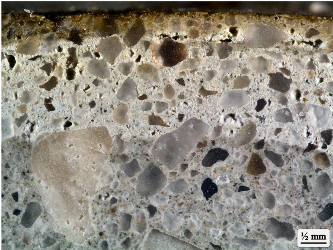
**Figure 4.** Cross-section photographs taken under the microscope showing the acid attacked cement paste of Specimen No. 34. The layer of penetrated epoxy can be seen in both photographs.
