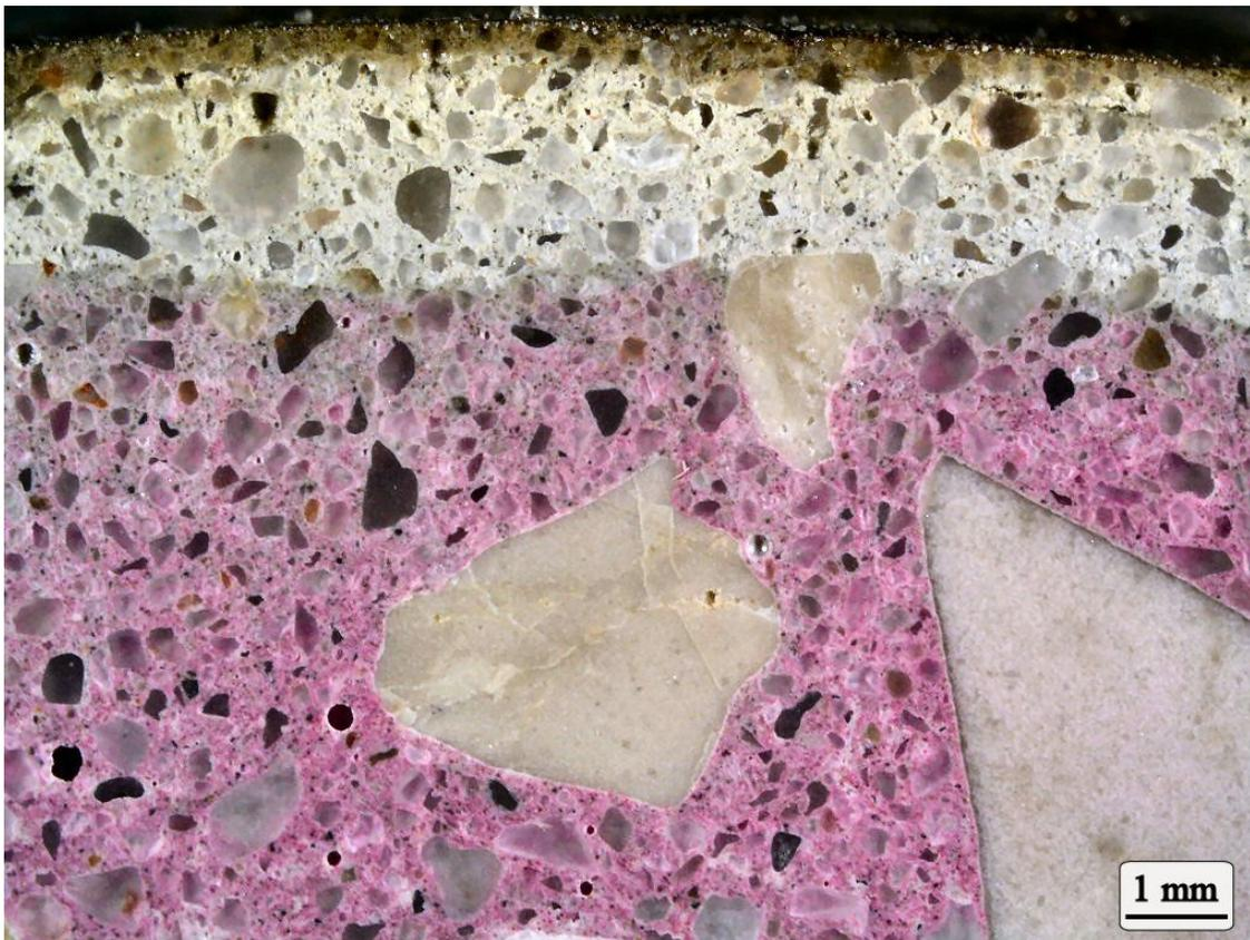
**Figure 6.** Cross-section photographs of Specimen No. 34 following the exposure to phenolphthalein solution. The depth to which the pH has been lowered by the acid exposure is represented by the uncolored cement paste.
