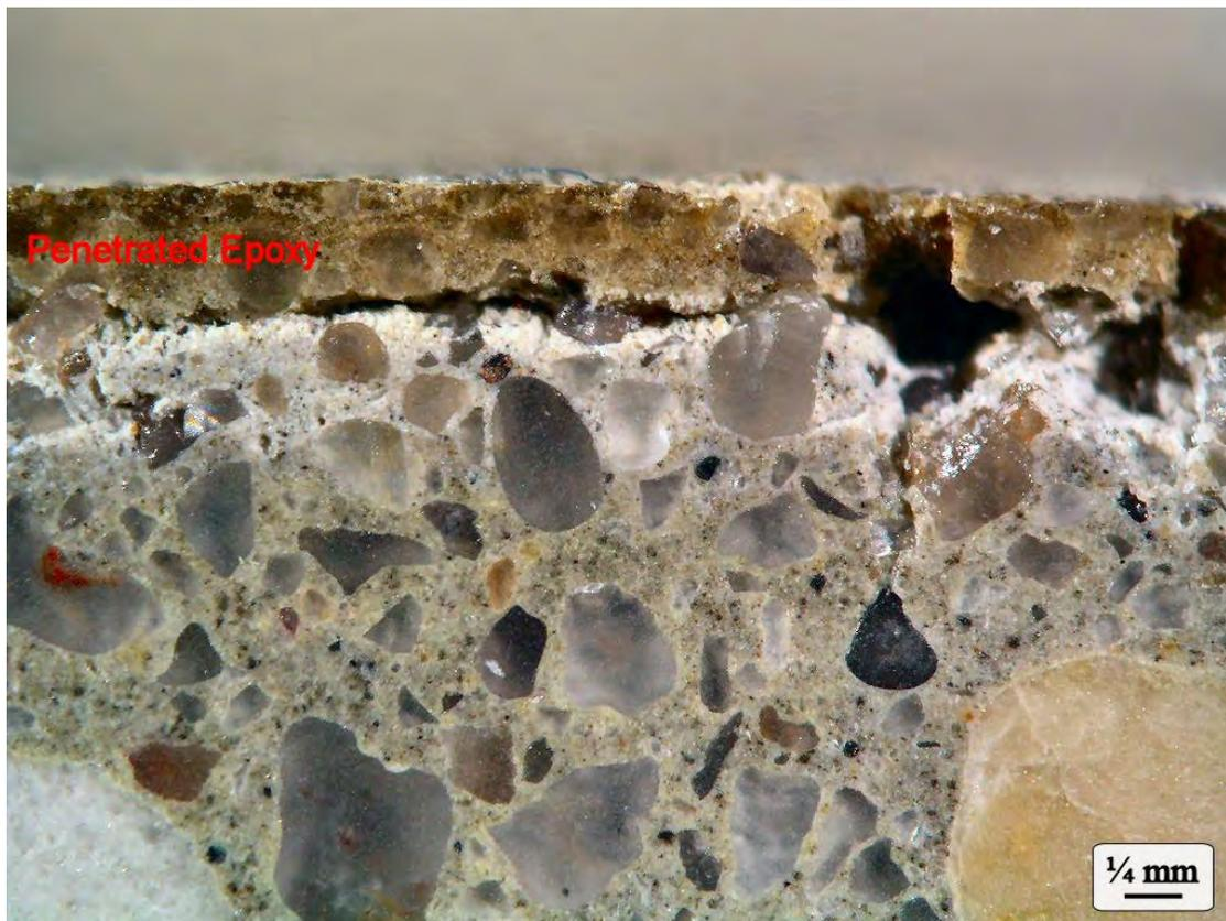
Figure 6. Cross-section photographs taken under the microscope showing the acid attacked cement paste of Specimen No. 31.
