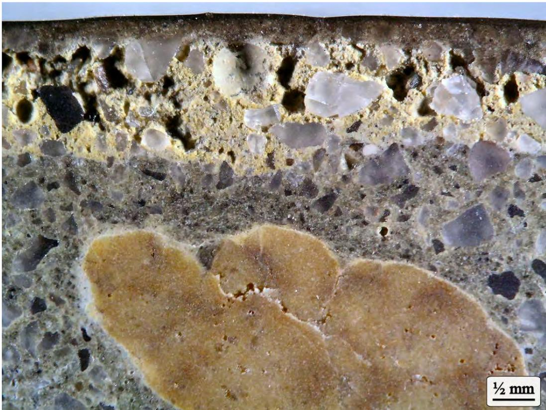
**Figure 3. Cross-section photographs taken under the microscope showing the acid attacked cement paste of Specimen No. 24. The upper dark portion of the cement paste has been penetrated by the epoxy coating.**
