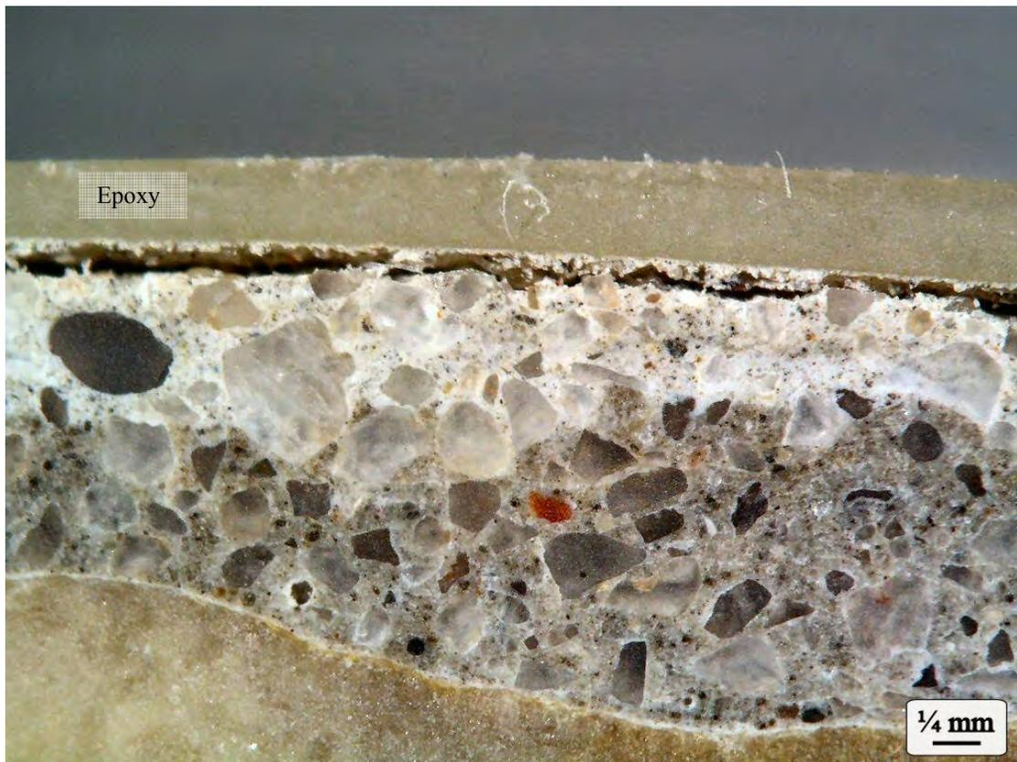
**Figure 4.** Cross-section photographs taken under the microscope showing the acid attacked cement paste of Specimen No. 13. In the lower photograph, the epoxy has pulled away a portion of the attacked cement paste.
