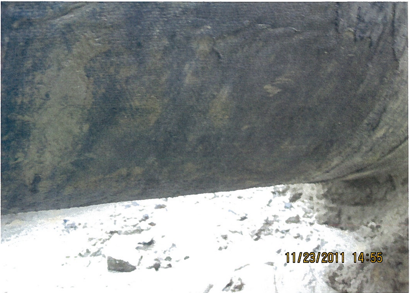
FINE CRACKS IN TOP LAYER OF WRAP ↓
