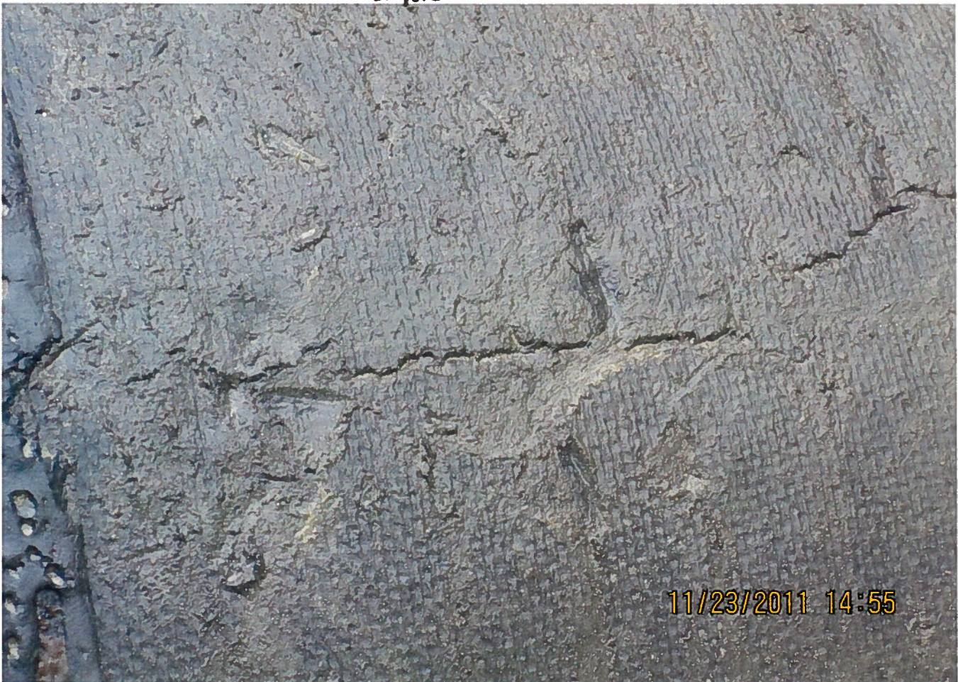
FINE CRACKS IN TOP LAYER OF WRAP ↓
