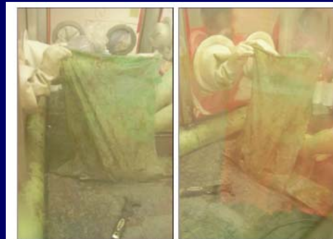
Figure 5. Removal of cured Decon Gel 1101 as a strippable film from cast steel glove-box floor.
