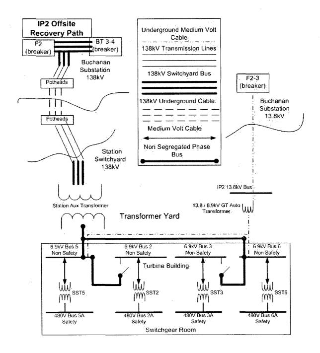
Figure 2.5-2 IP2 Offsite Power Scoping Diagram
