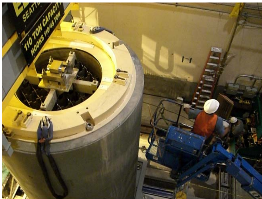
Shielded canisters like these are designed for safe dry storage and older spent nuclear fuel assemblies.
