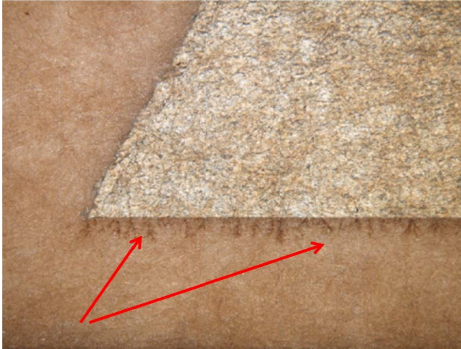
Fig. 30: Electrical treeing observed in “C” phase bushing only at electrically-stressed edge
