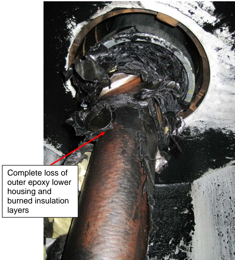
Fig. 12: Failure of the “B” phase bushing insulating material
