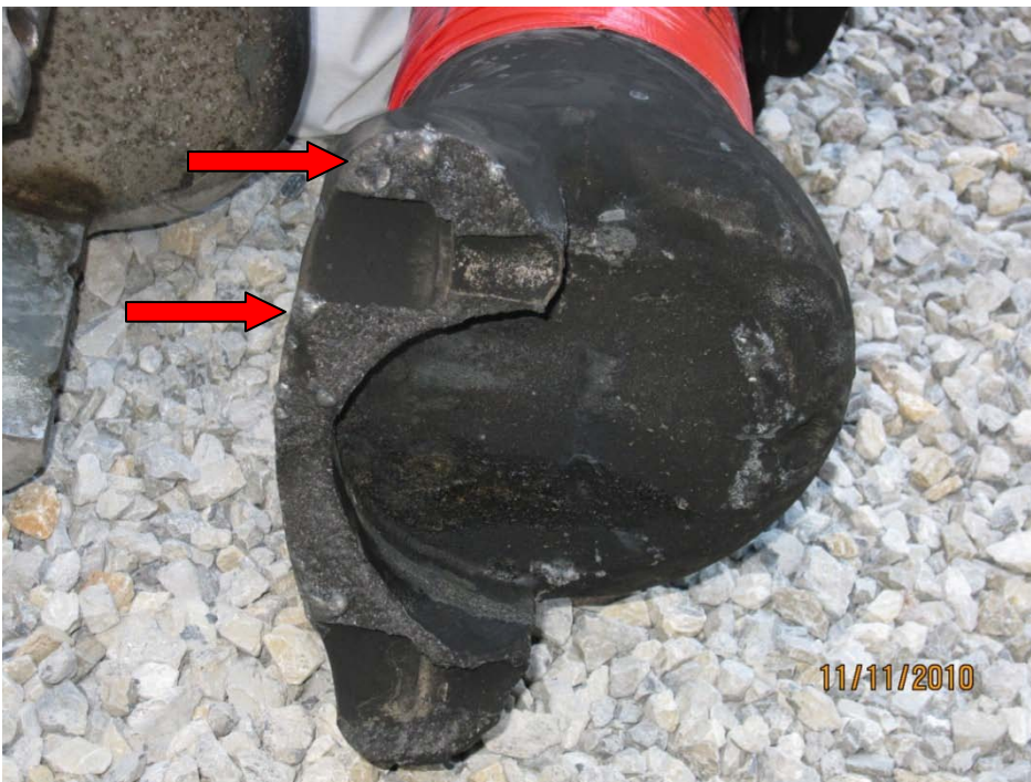
Fig. 8: Fracture surface of “B” phase HV feeder bus section showing localized melting
