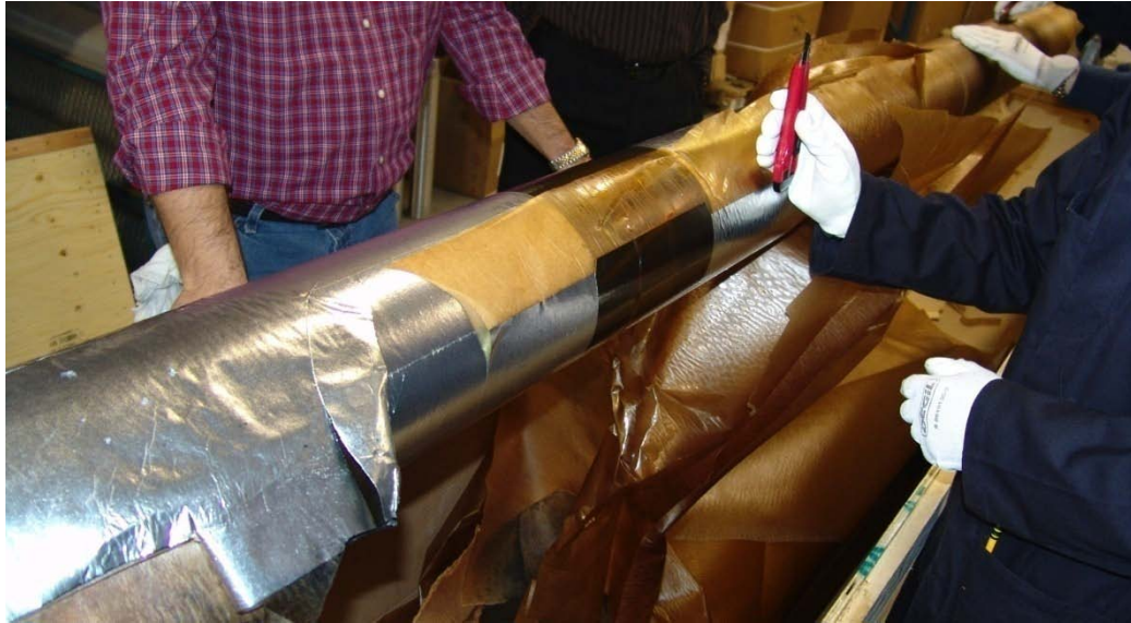
Fig. 15: Overview photo of bushing's capacitor structure as witnessed upon teardown
