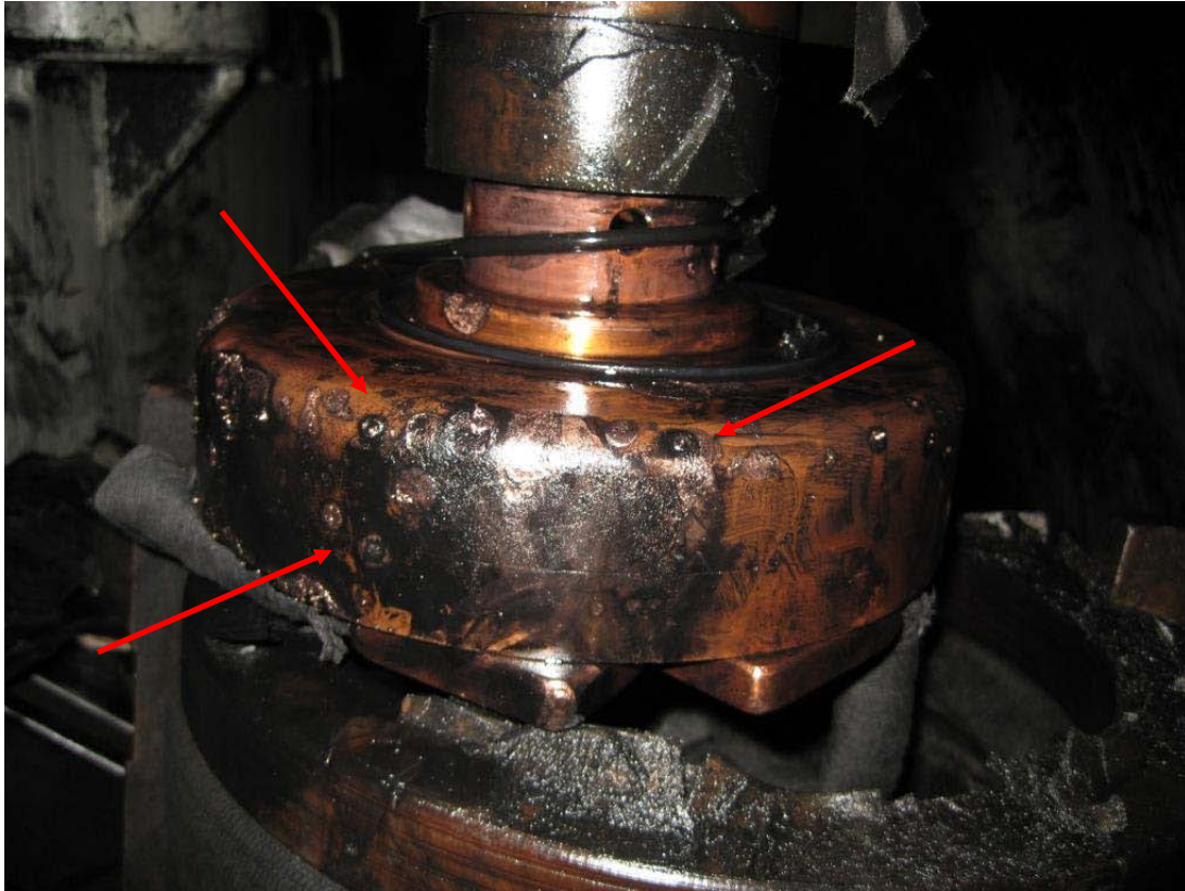
Fig. 11: Numerous arc strikes observed at the bottom terminal of the "B" phase bushing
