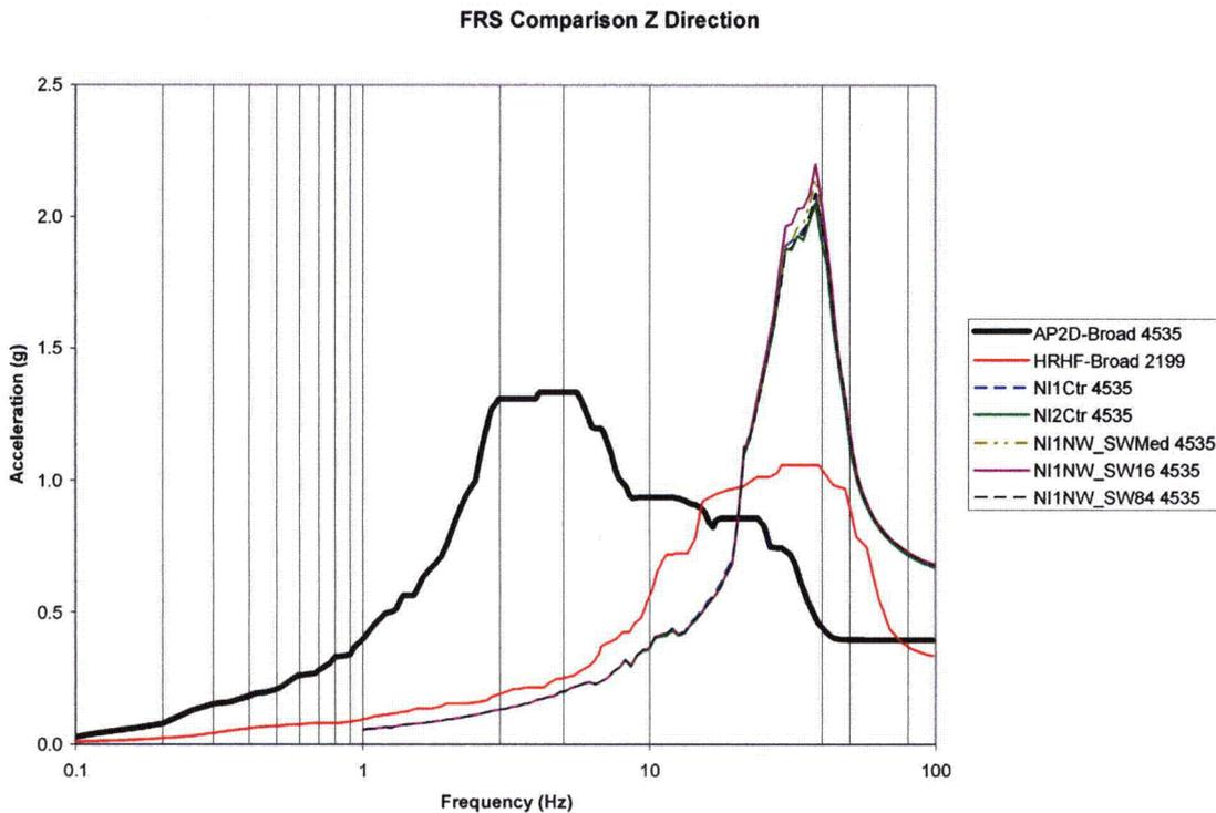
**Figure C-12: 2D SW Backfill Parametric FRS Comparison of Node 4535 in Z-Direction**
