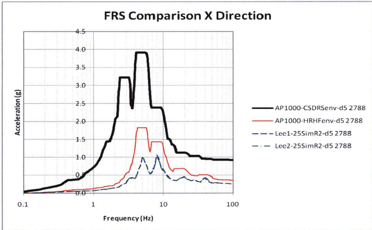
Figure 7-13: 3D FRS and AP1000 Envelope Comparison of Node 2788 in X-Direction
