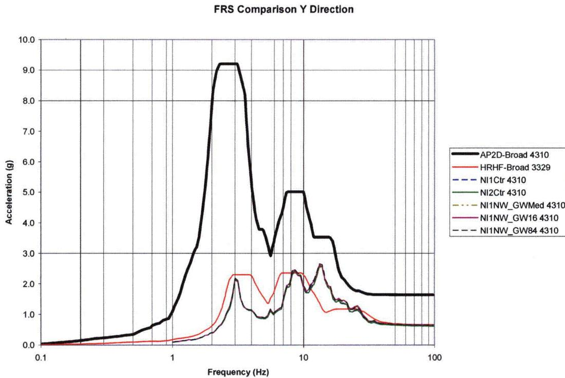
**Figure B-7: 2D GW Backfill Parametric FRS Comparison of Node 4310 in Y-Direction**
