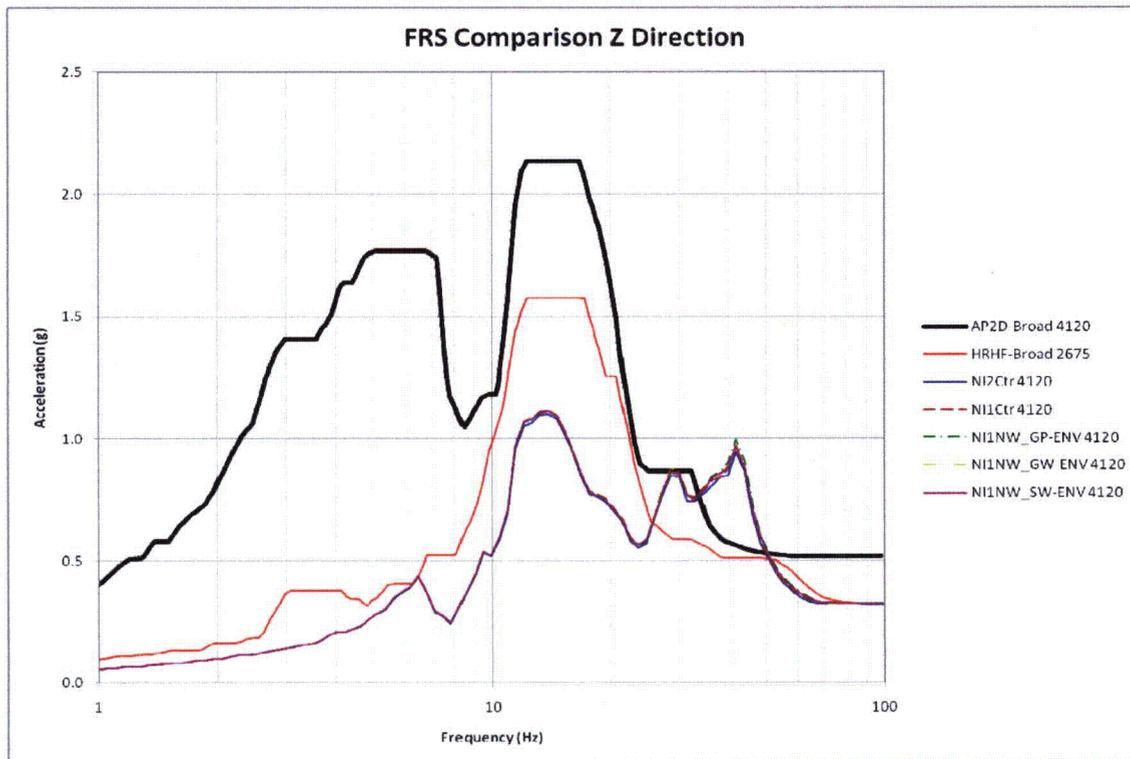
Figure 5-6: 2D Parametric FRS Comparison of Node 4120 in Z-Direction
