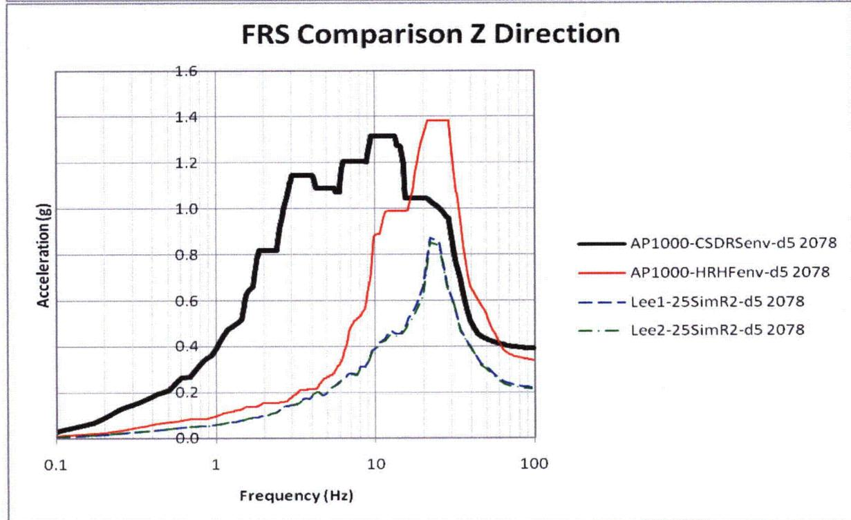
**Figure 3.7-208a Comparison of 3D FRS and AP1000 Envelope (Z-Direction, Nodes 1761 and 2078)**
