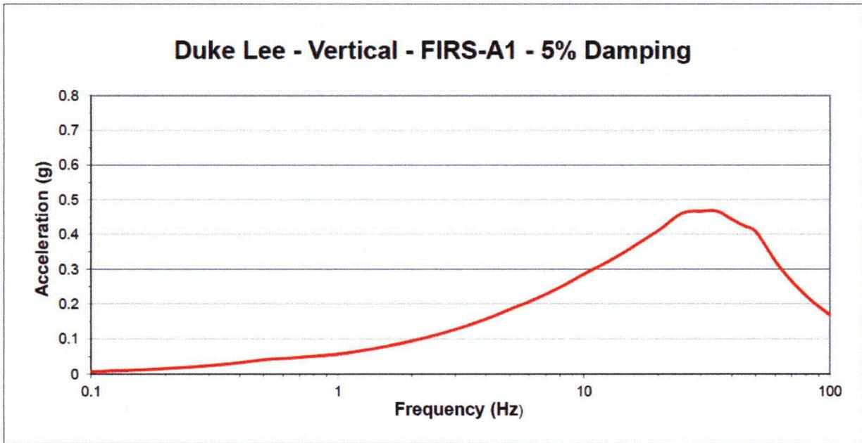
Figure 3-4: Duke Lee Vertical Foundation Input Response Spectra at 5% Damping
