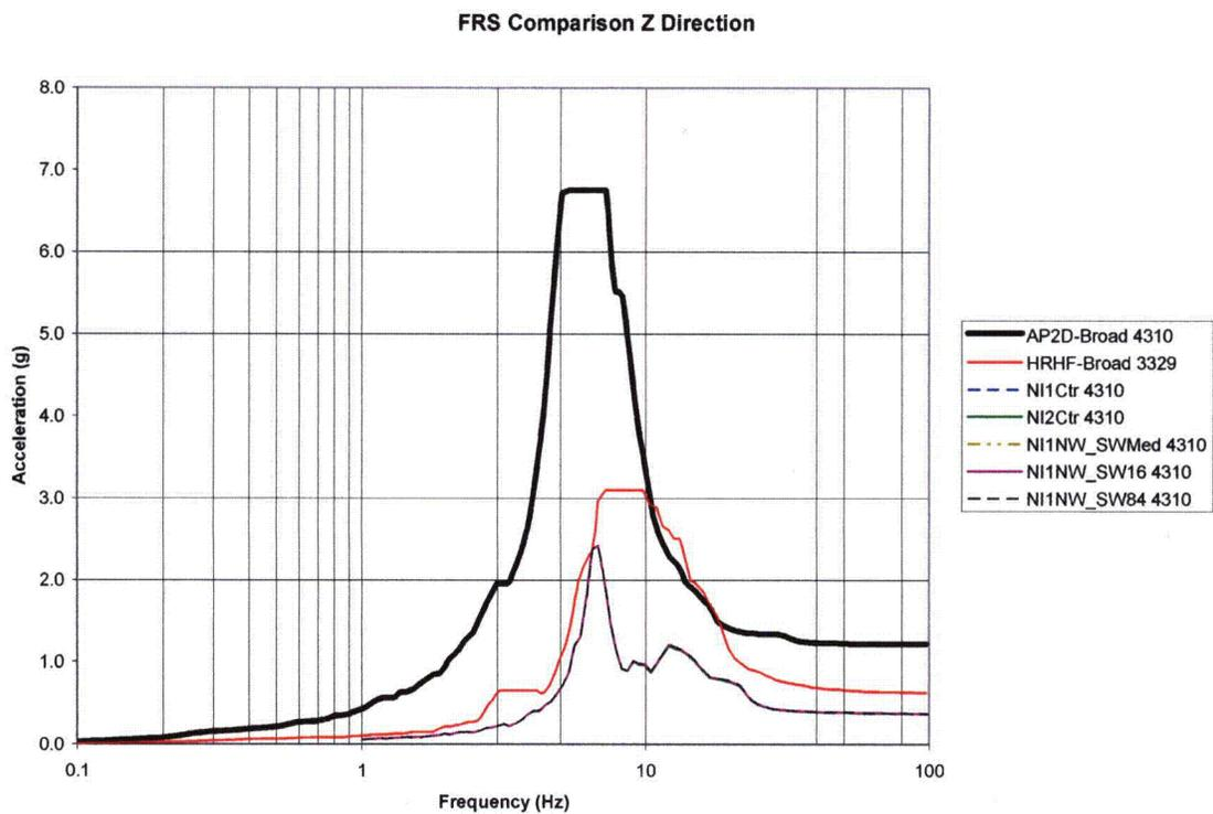
**Figure C-8: 2D SW Backfill Parametric FRS Comparison of Node 4310 in Z-Direction**
