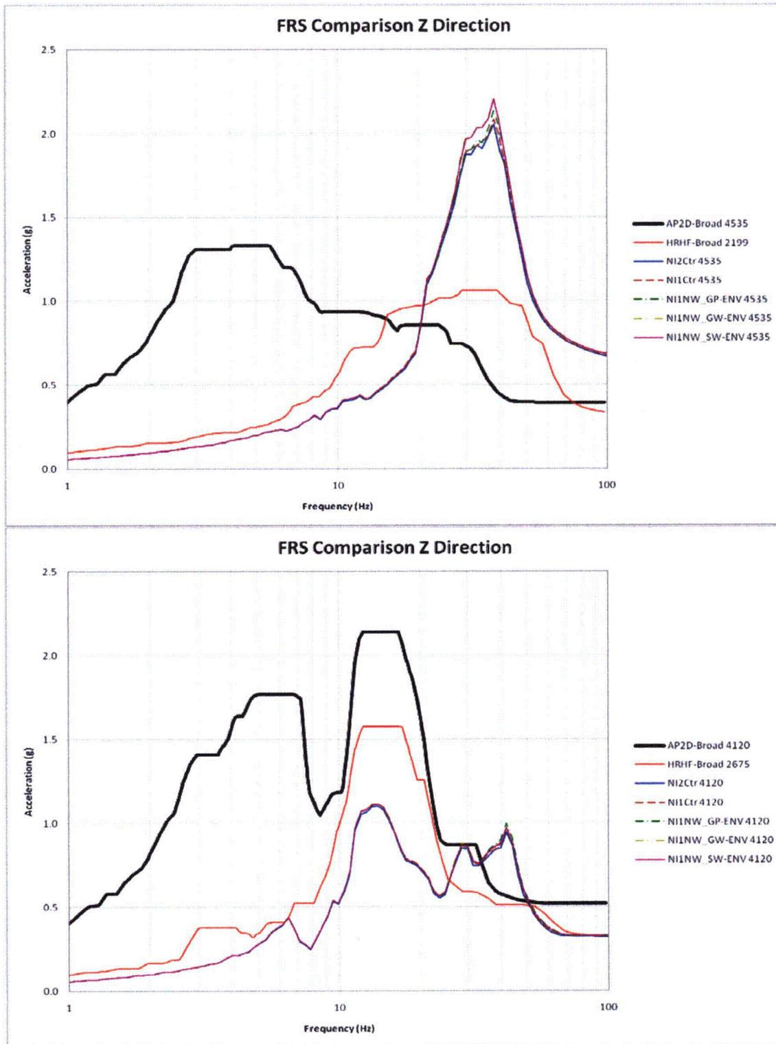
**Figure 3.7-205b Comparison of 2D FRS and AP1000 Envelope (Z-Direction, Nodes 4535 and 4120)**
