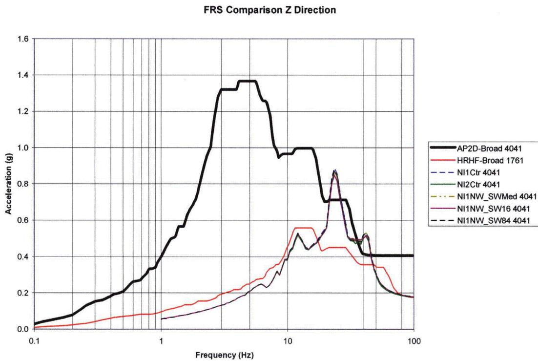
Figure C-2: 2D SW Backfill Parametric FRS Comparison of Node 4041 in Z-Direction
