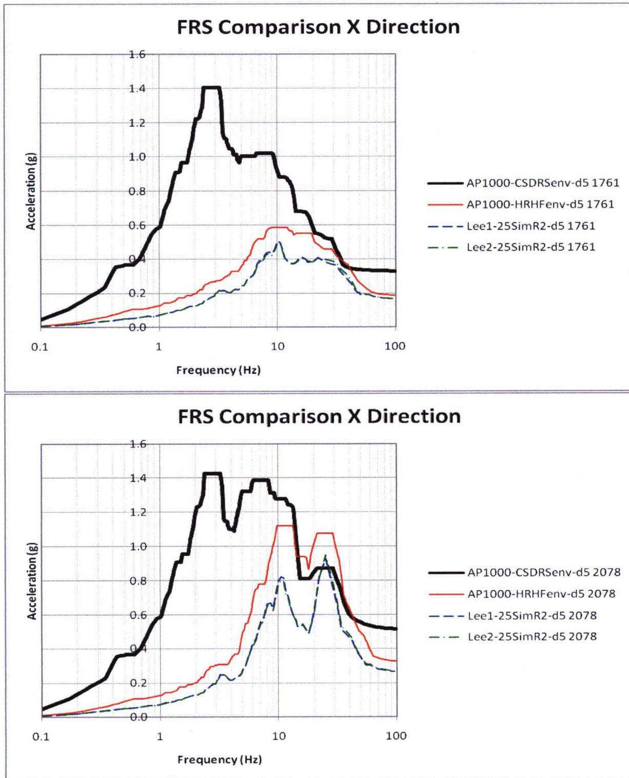
**Figure 3.7-206a Comparison of 3D FRS and AP1000 Envelope (X-Direction, Nodes 1761 and 2078)**
