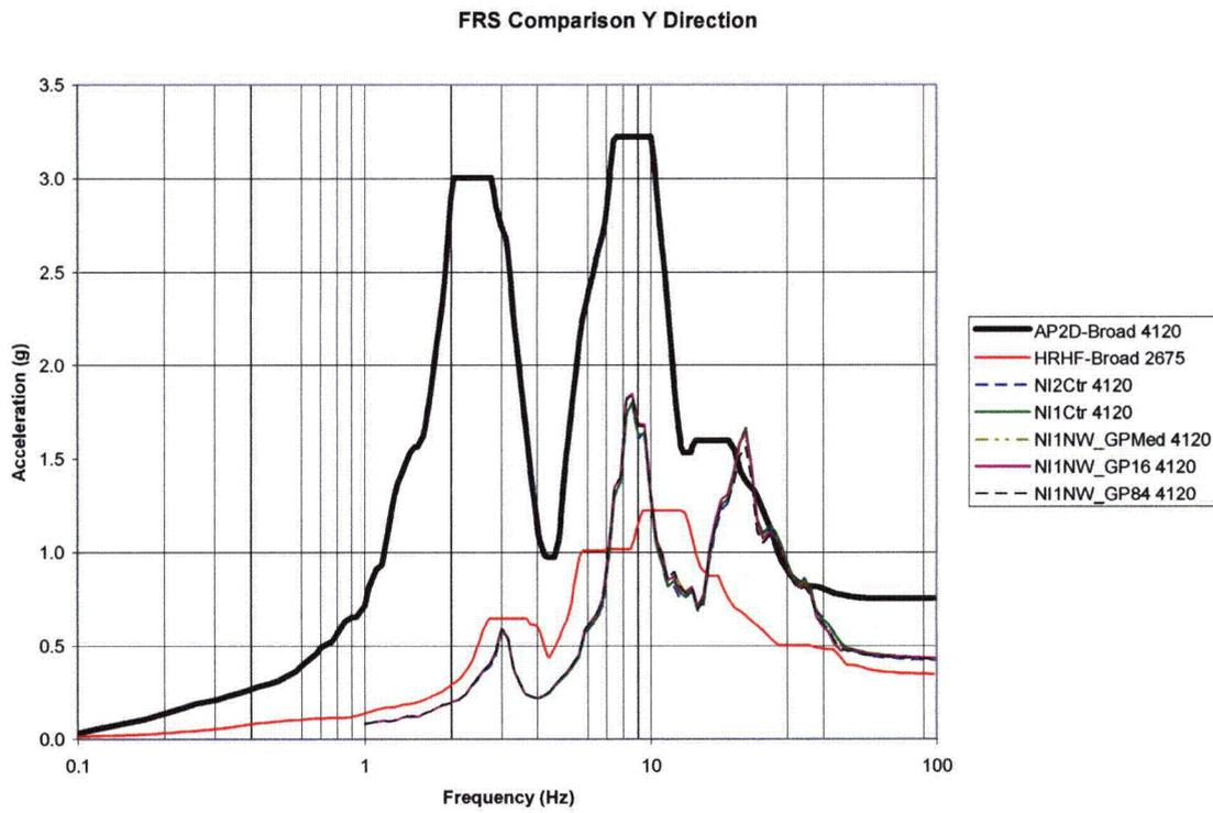
Figure A-5: 2D GP Backfill Parametric FRS Comparison of Node 4120 in Y-Direction
