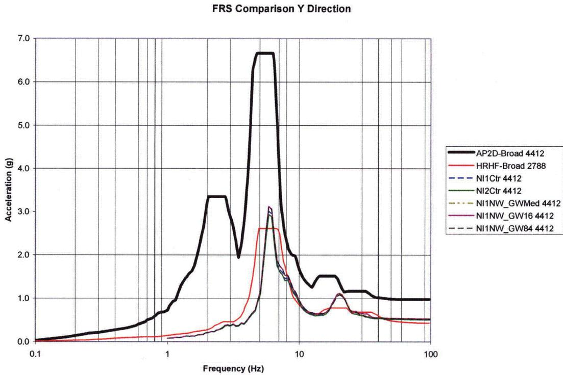
Figure B-9: 2D GW Backfill Parametric FRS Comparison of Node 4412 in Y-Direction
