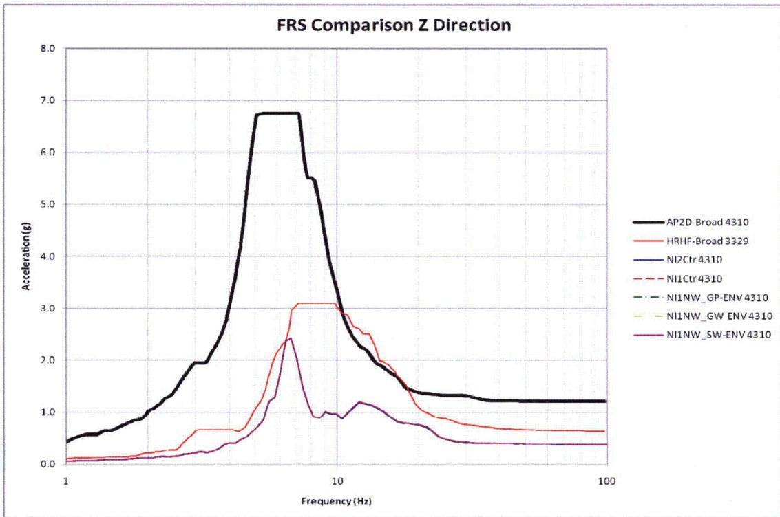
Figure 5-8: 2D Parametric FRS Comparison of Node 4310 in Z-Direction
