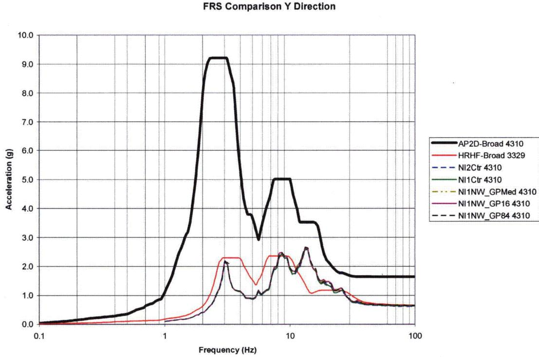
Figure A-7: 2D GP Backfill Parametric FRS Comparison of Node 4310 in Y-Direction
