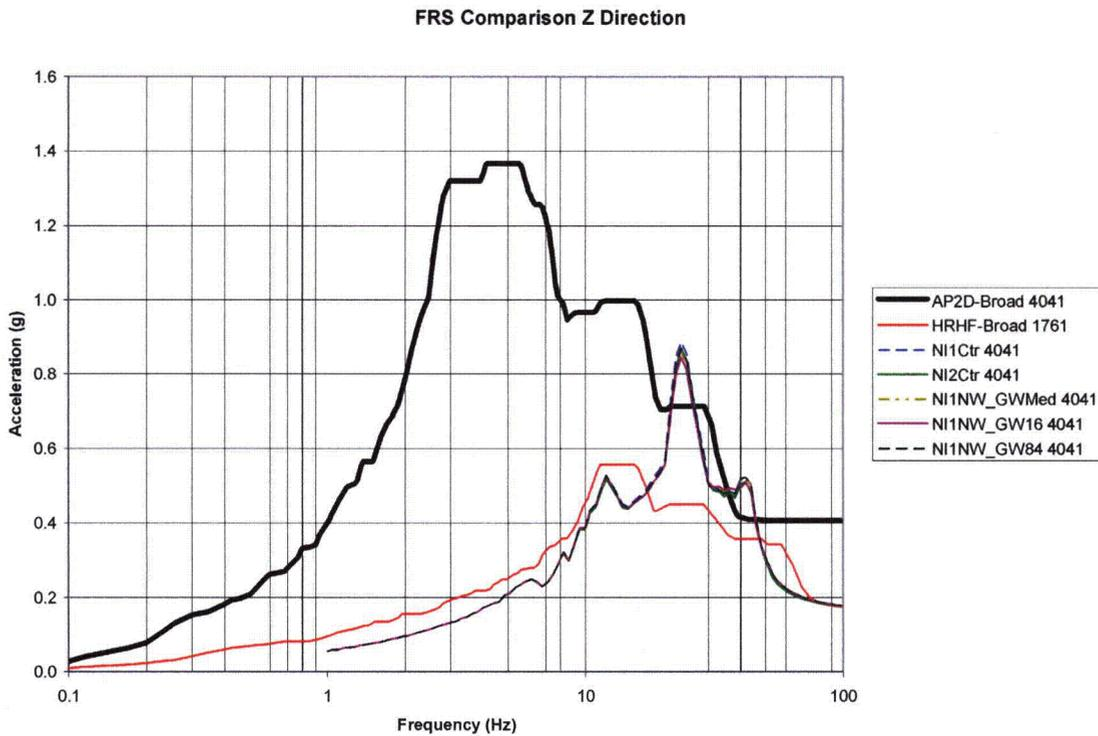
Figure B-2: 2D GW Backfill Parametric FRS Comparison of Node 4041 in Z-Direction
