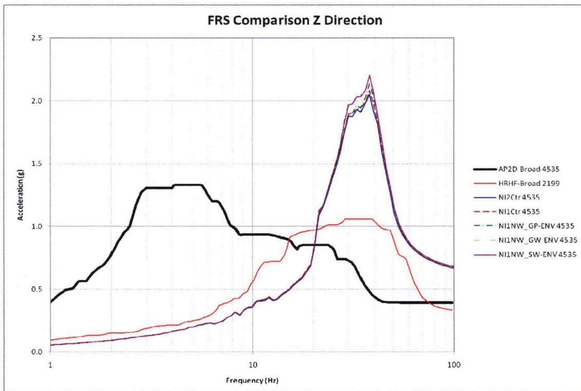
Figure 5-12: 2D Parametric FRS Comparison of Node 4535 in Z-Direction
