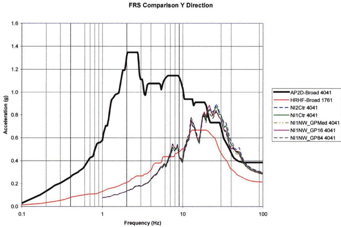
Figure A-1: 2D GP Backfill Parametric FRS Comparison of Node 4041 in Y-Direction
