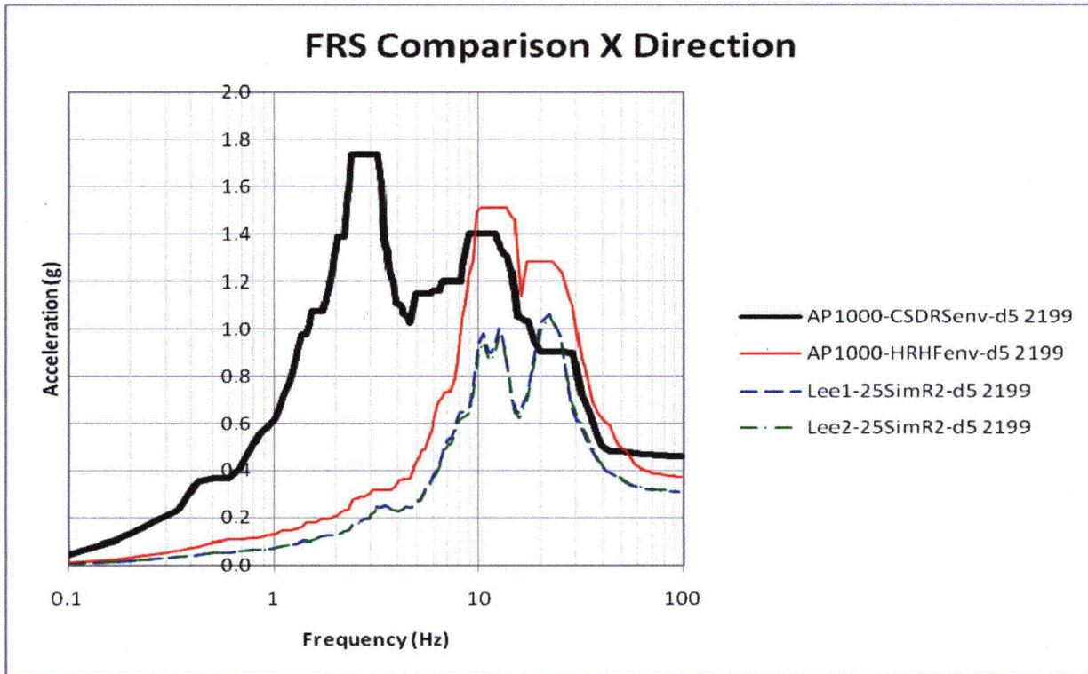
Figure 7-7: 3D FRS and AP1000 Envelope Comparison of Node 2199 in X-Direction
