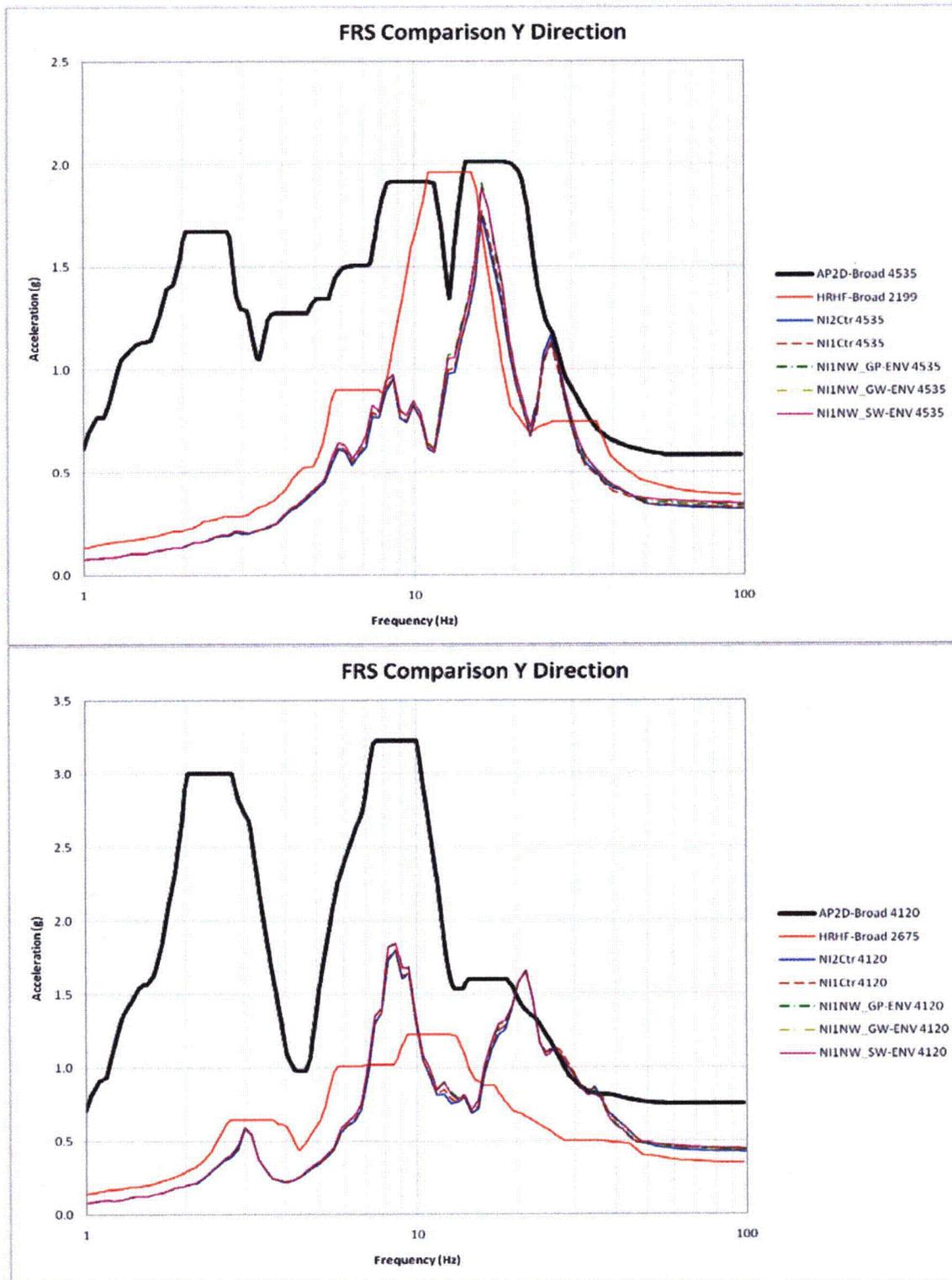
**Figure 3.7-204b Comparison of 2D FRS and AP1000 Envelope (Y-Direction, Nodes 4535 and 4120)**
