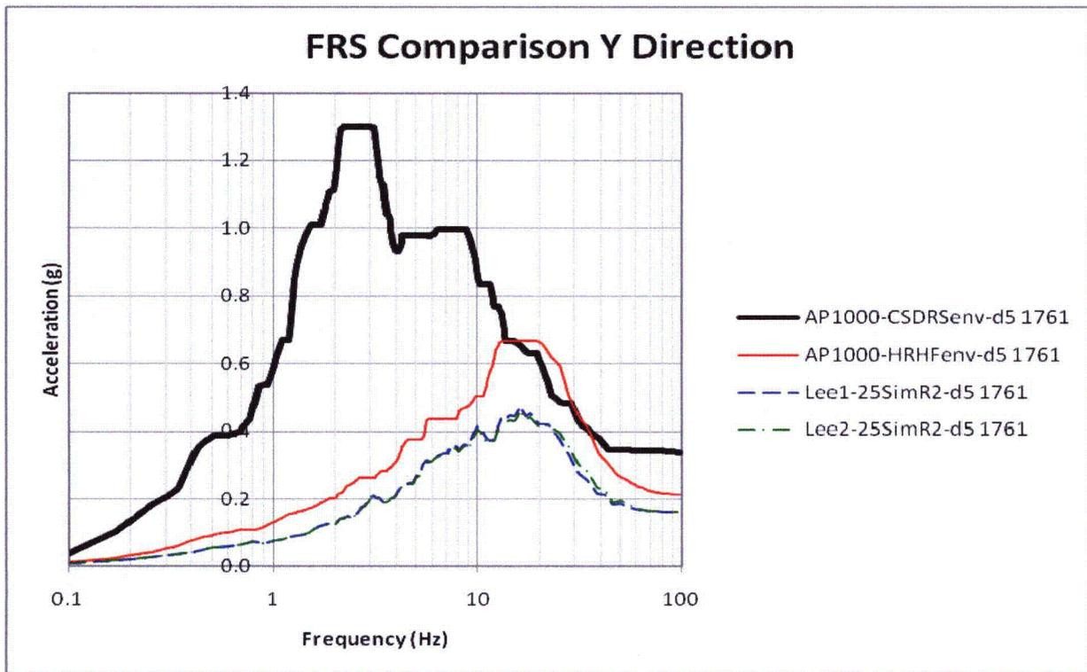
Figure 7-2: 3D FRS and AP1000 Envelope Comparison of Node 1761 in Y-Direction
