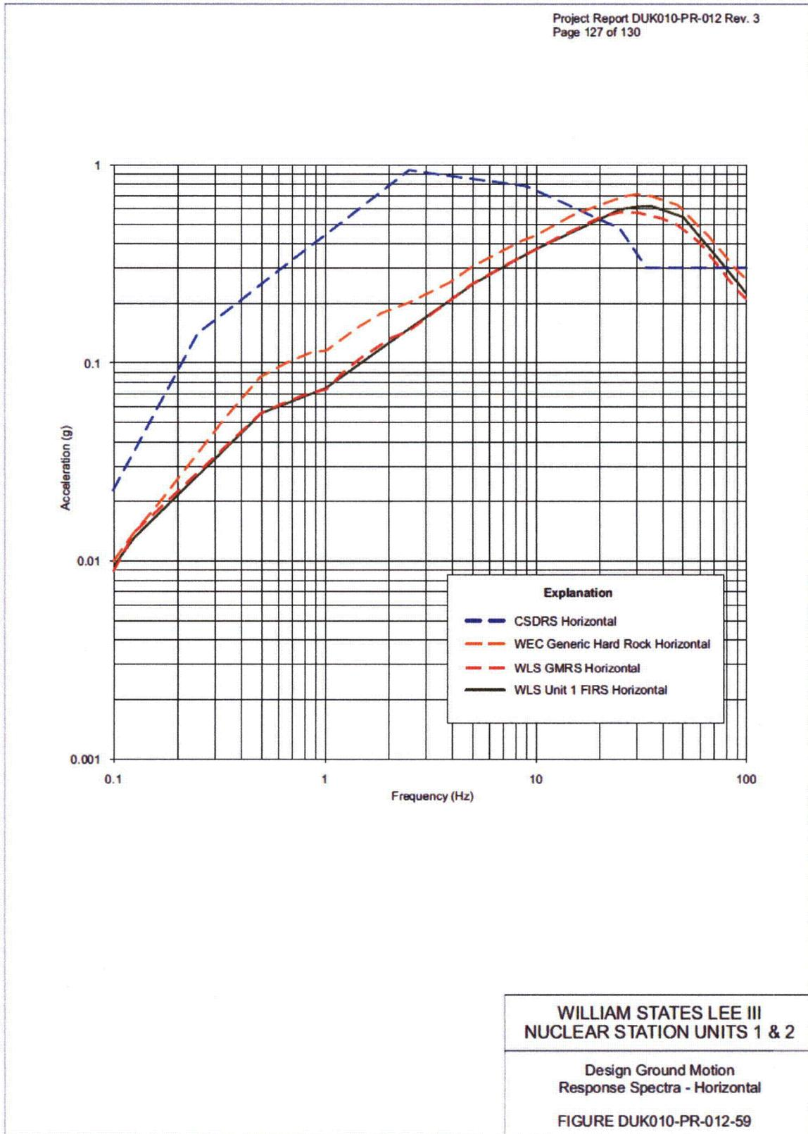
Figure 3-1: Duke Lee Units 1 and 2 Horizontal Ground Motion Response Spectra
