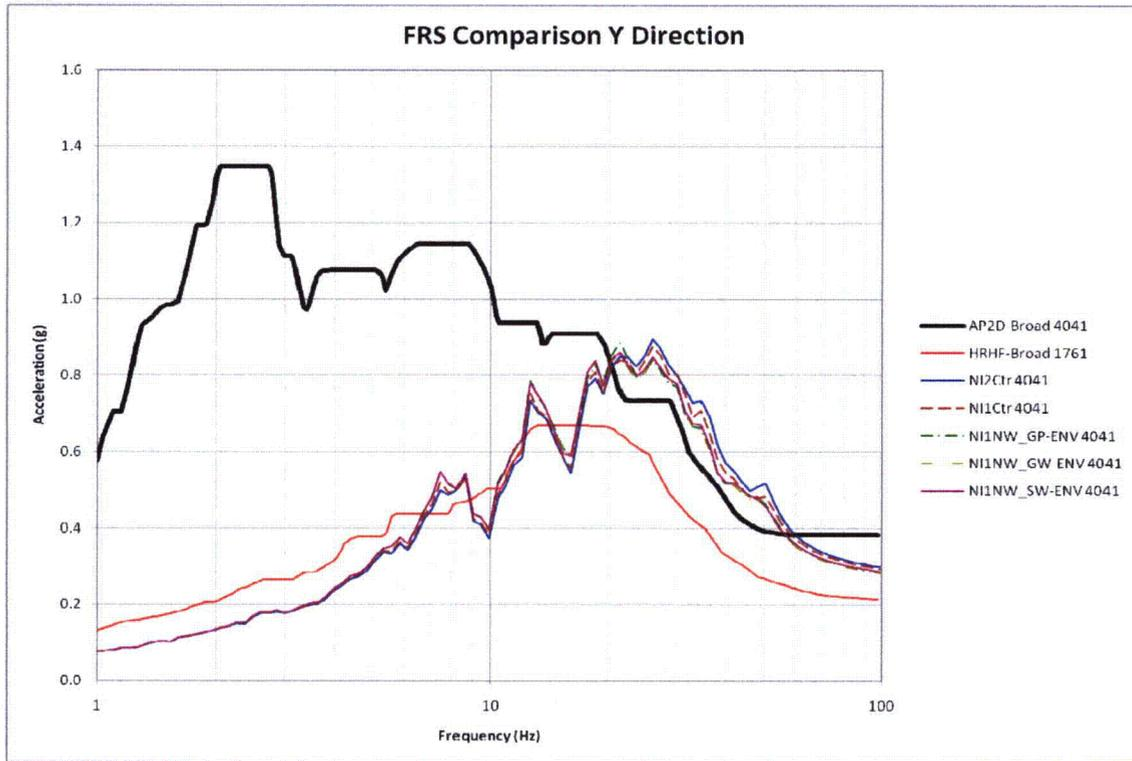
Figure 5-1: 2D Parametric FRS Comparison of Node 4041 in Y-Direction
