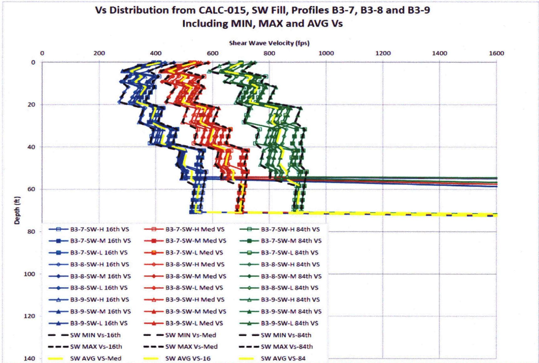
Figure 2.5-4: SW Engineered Fill Dynamic Profile
