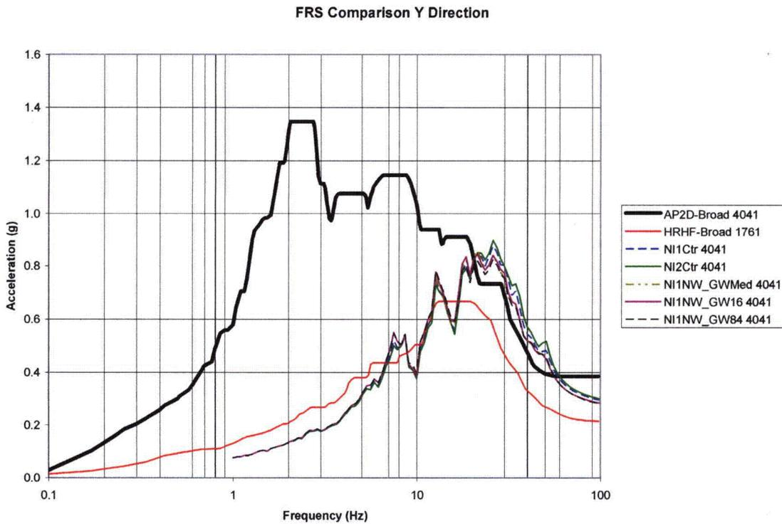
Figure B-1: 2D GW Backfill Parametric FRS Comparison of Node 4041 in Y-Direction
