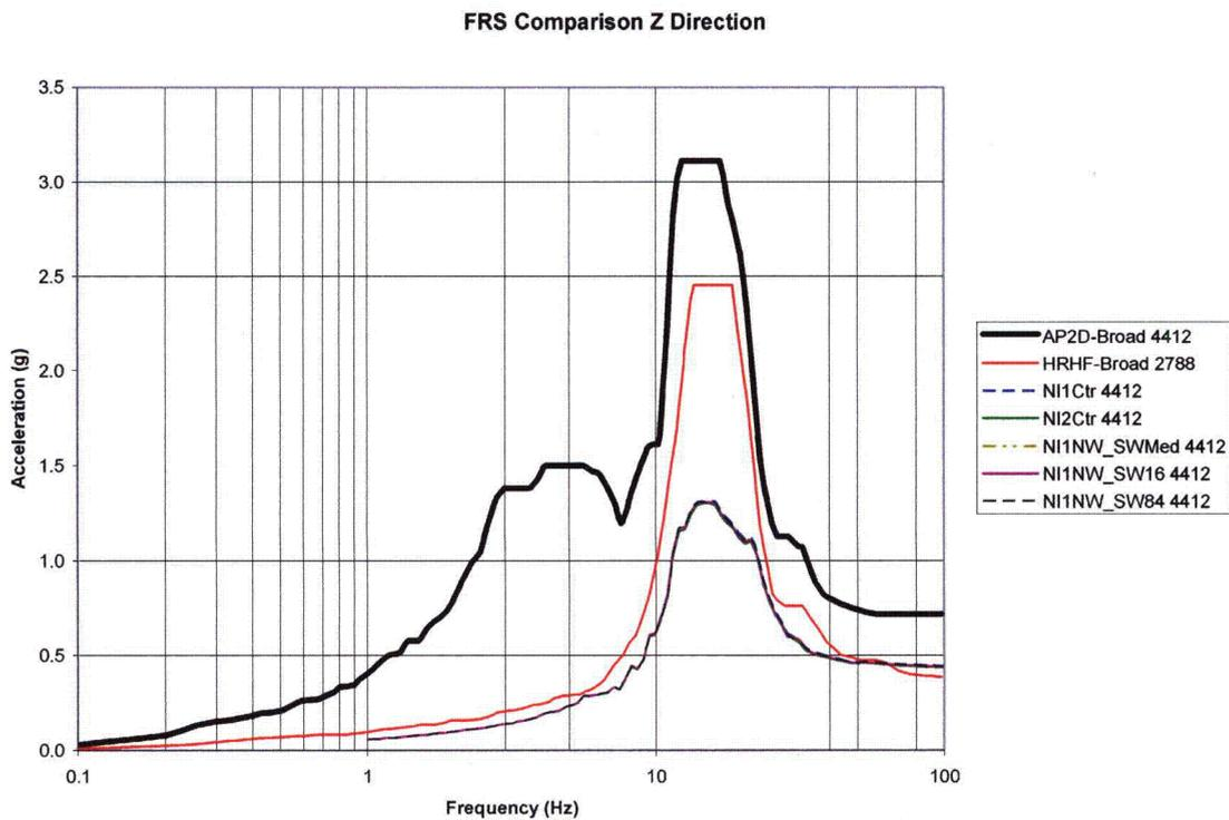
Figure C-10: 2D SW Backfill Parametric FRS Comparison of Node 4412 in Z-Direction
