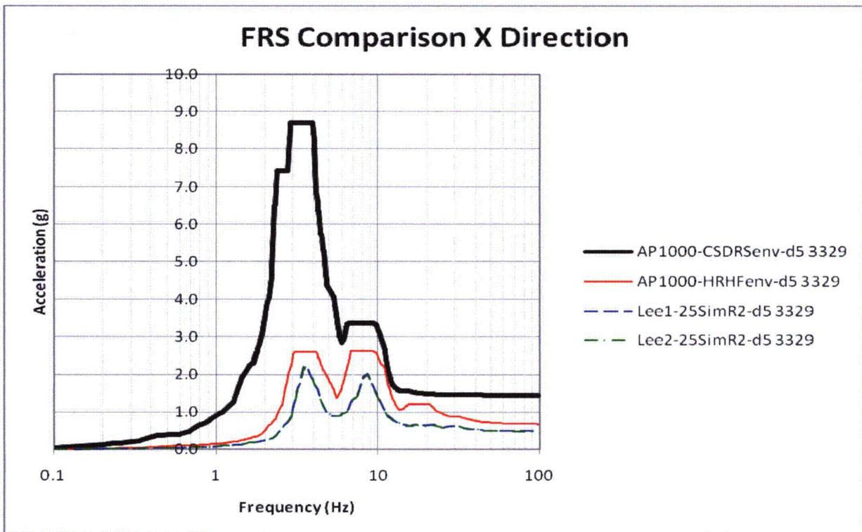
Figure 7-16: 3D FRS and AP1000 Envelope Comparison of Node 3329 in X-Direction
