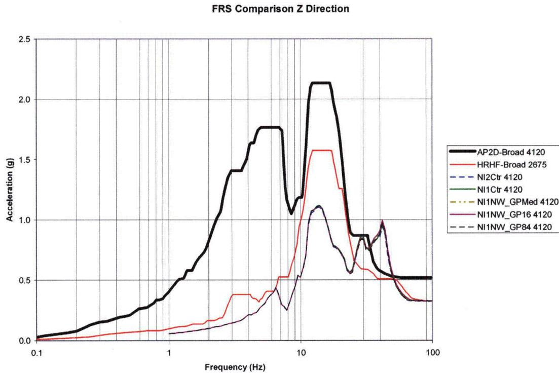
Figure A-6: 2D GP Backfill Parametric FRS Comparison of Node 4120 in Z-Direction
