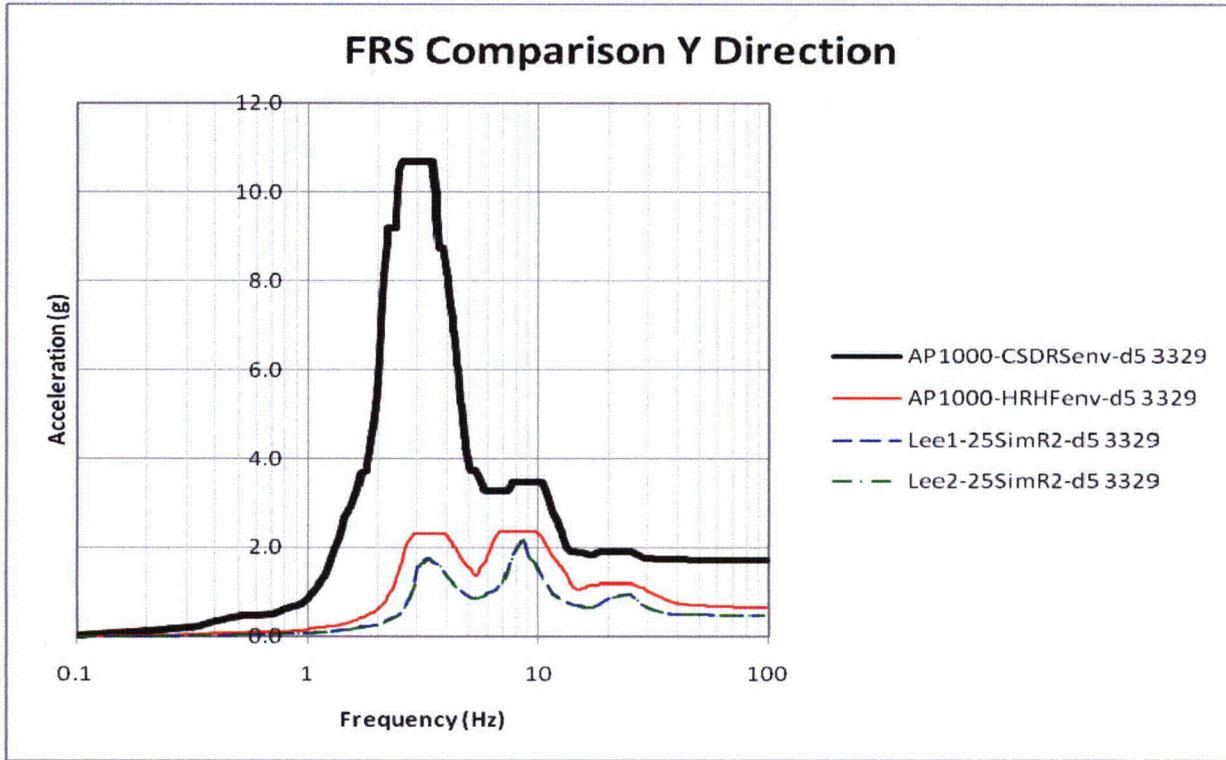
Figure 7-17: 3D FRS and AP1000 Envelope Comparison of Node 3329 in Y-Direction
