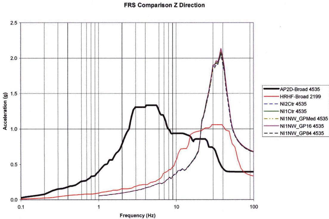
Figure A-12: 2D GP Backfill Parametric FRS Comparison of Node 4535 in Z-Direction
