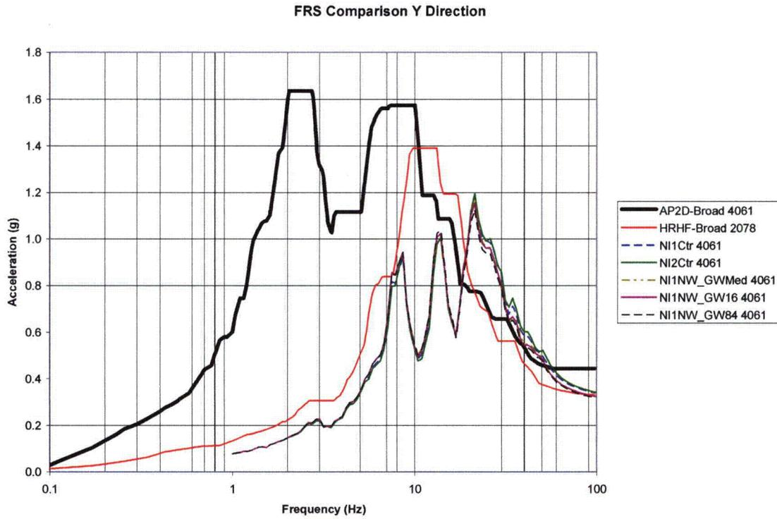
Figure B-3: 2D GW Backfill Parametric FRS Comparison of Node 4061 in Y-Direction
