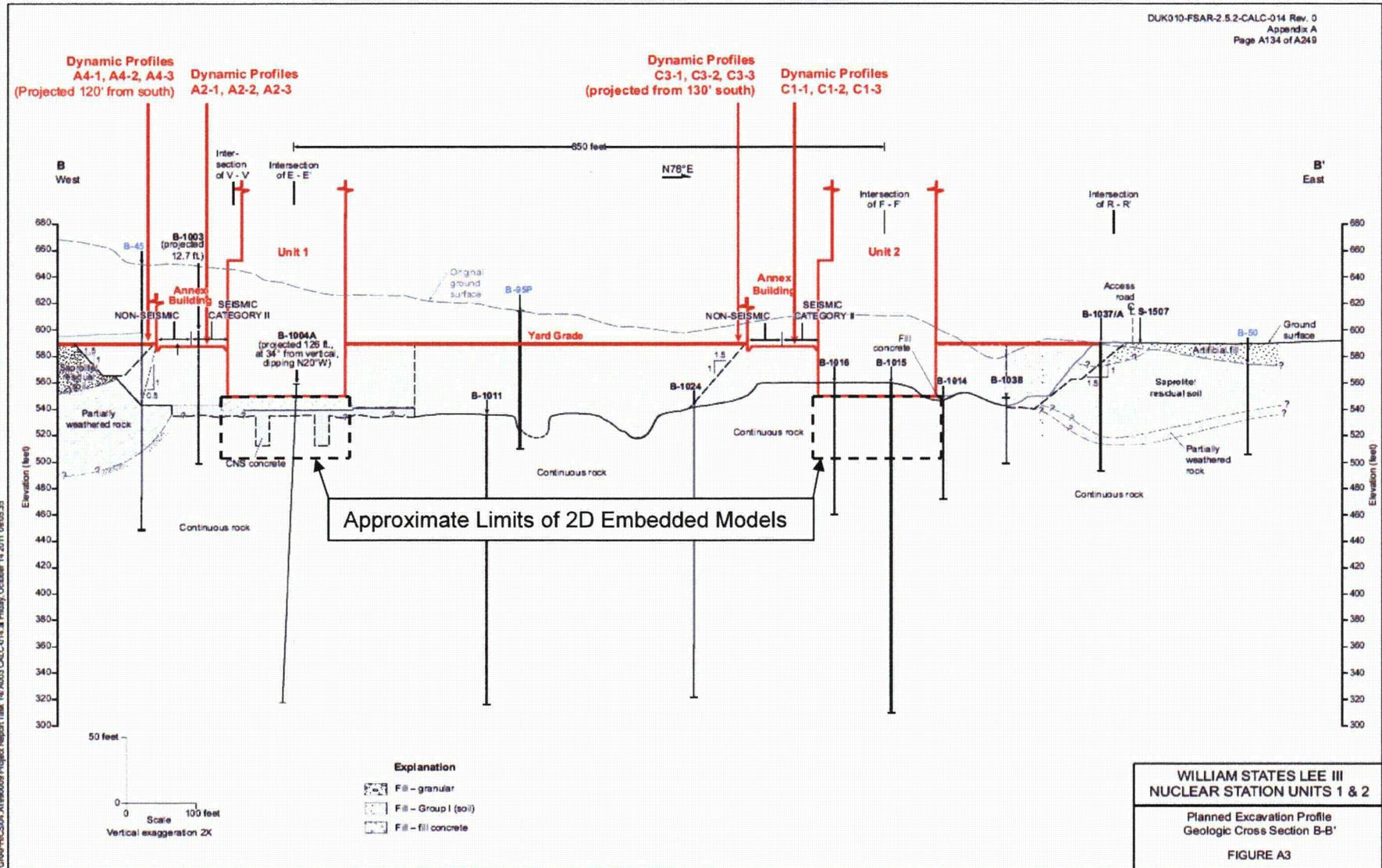
Figure 2.2-1: Cross-Section B-B
