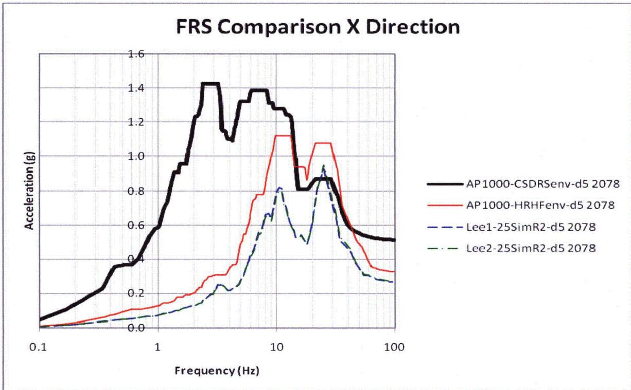
Figure 7-4: 3D FRS and AP1000 Envelope Comparison of Node 2078 in X-Direction
