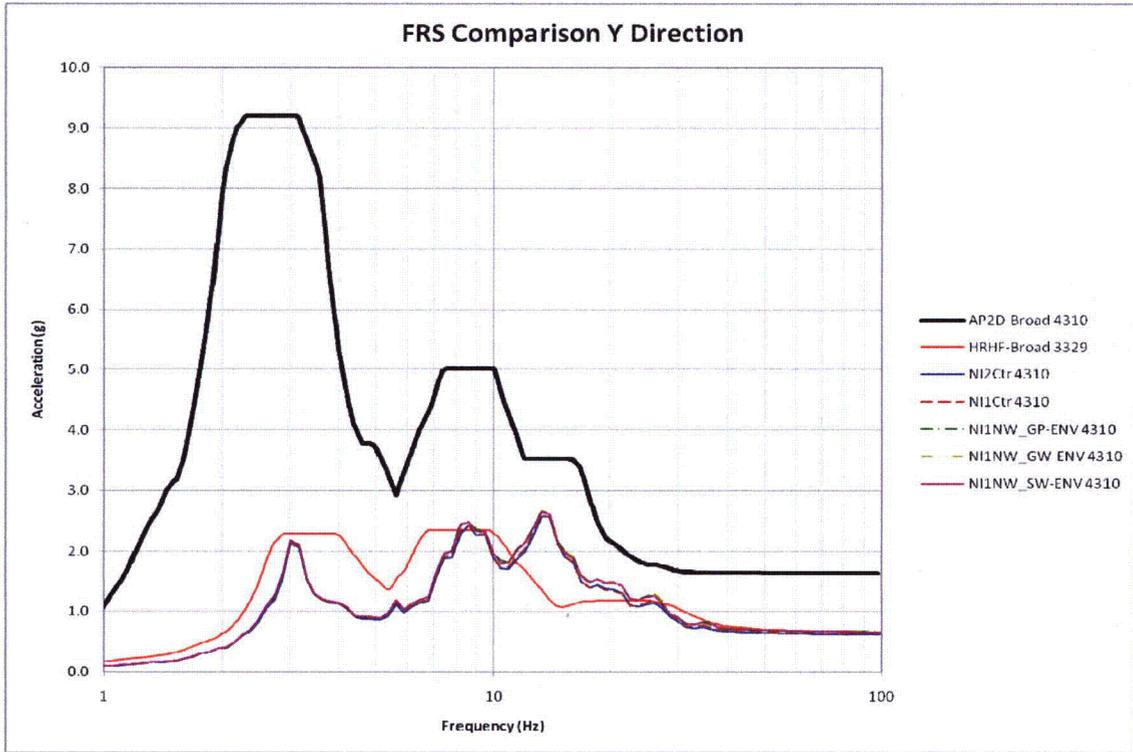
Figure 5-7: 2D Parametric FRS Comparison of Node 4310 in Y-Direction
