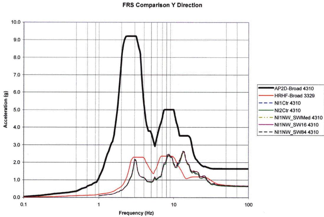
**Figure C-7: 2D SW Backfill Parametric FRS Comparison of Node 4310 in Y-Direction**
