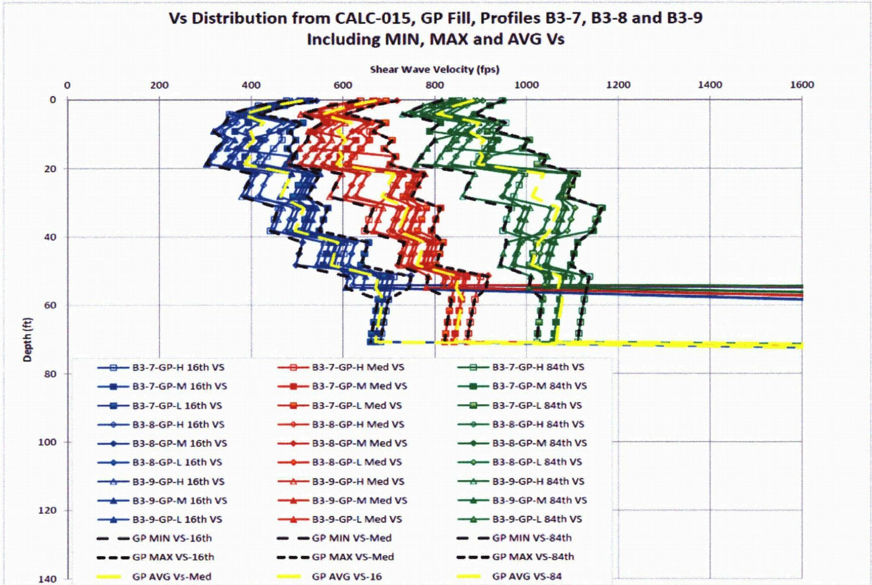
Figure 2.5-2: GP Engineered Fill Dynamic Profile
