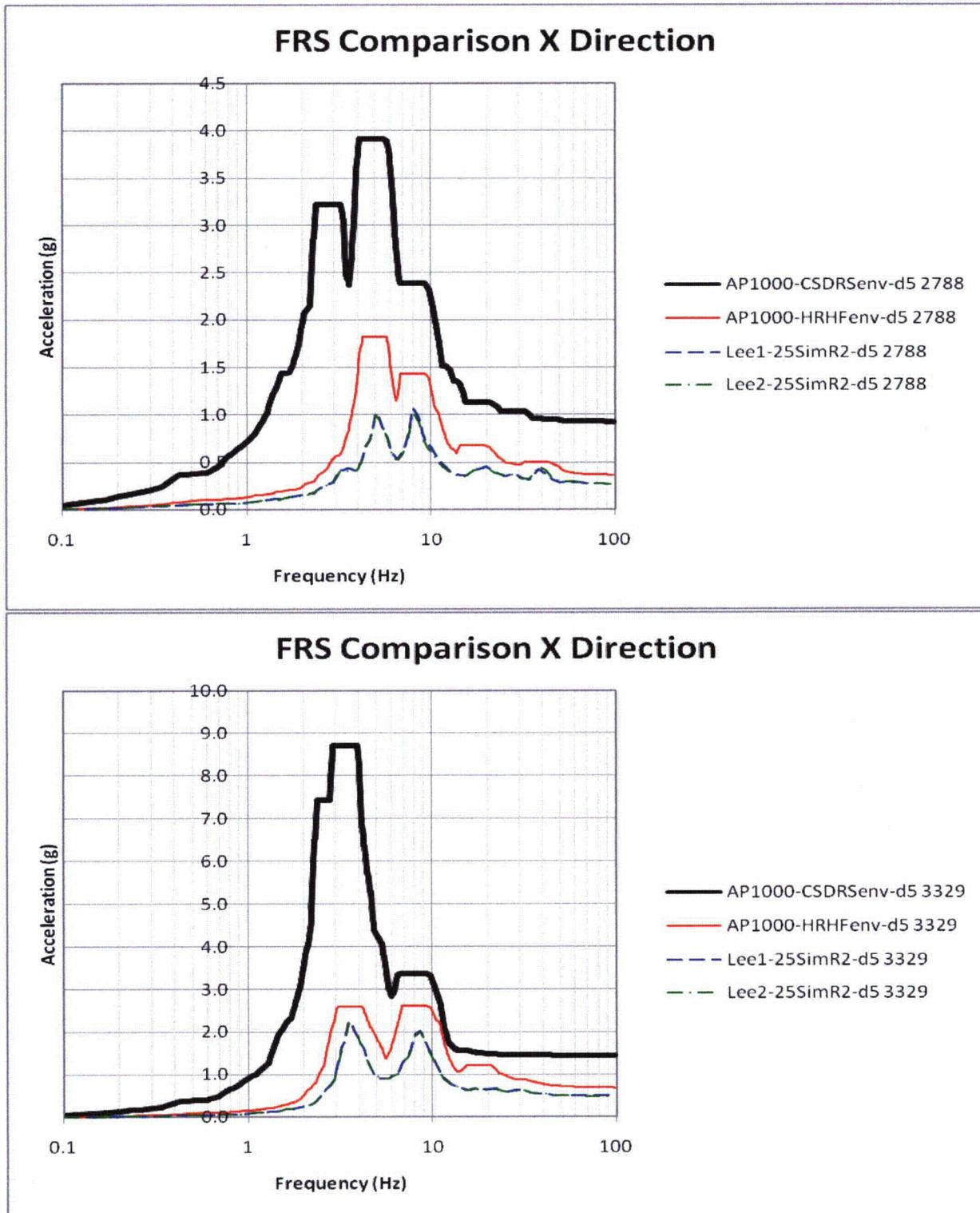
Figure 3.7-206c Comparison of 3D FRS and AP1000 Envelope (X-Direction, Nodes 2788 and 3329)
