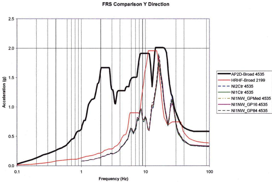
Figure A-11: 2D GP Backfill Parametric FRS Comparison of Node 4535 in Y-Direction
