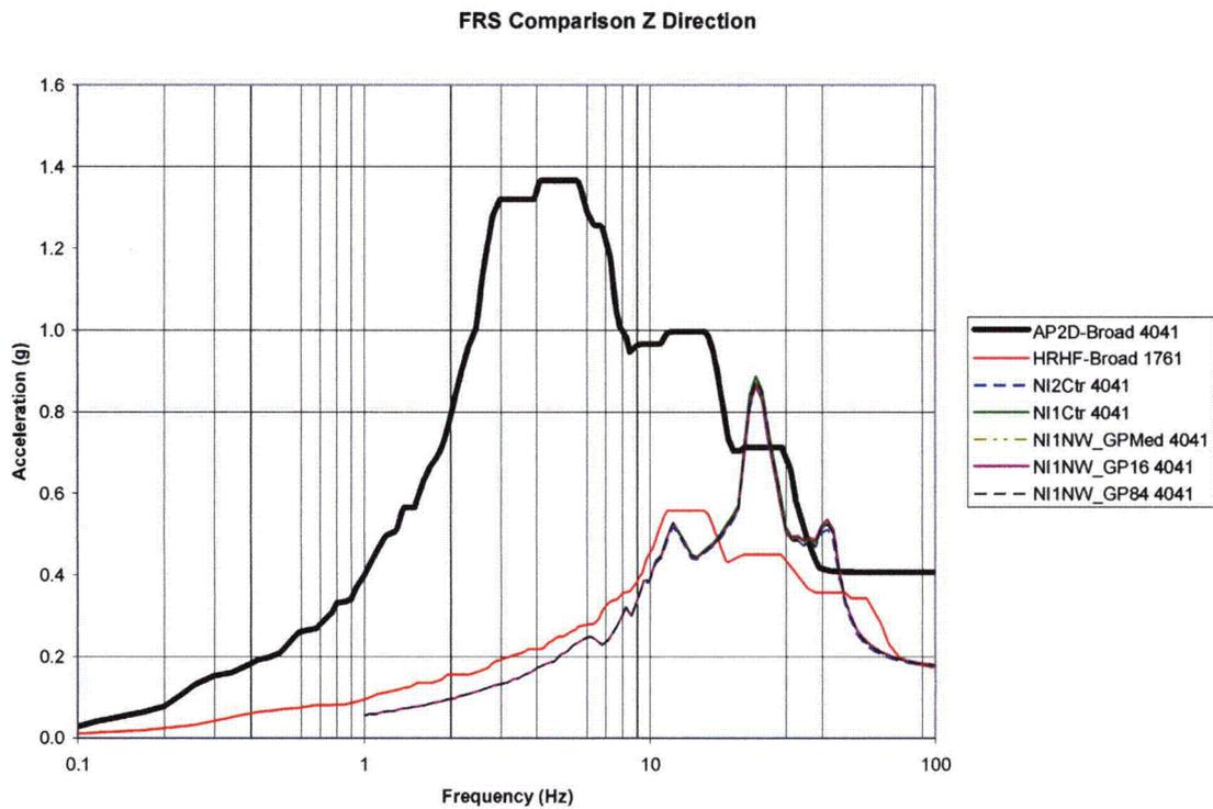
Figure A-2: 2D GP Backfill Parametric FRS Comparison of Node 4041 in Z-Direction
