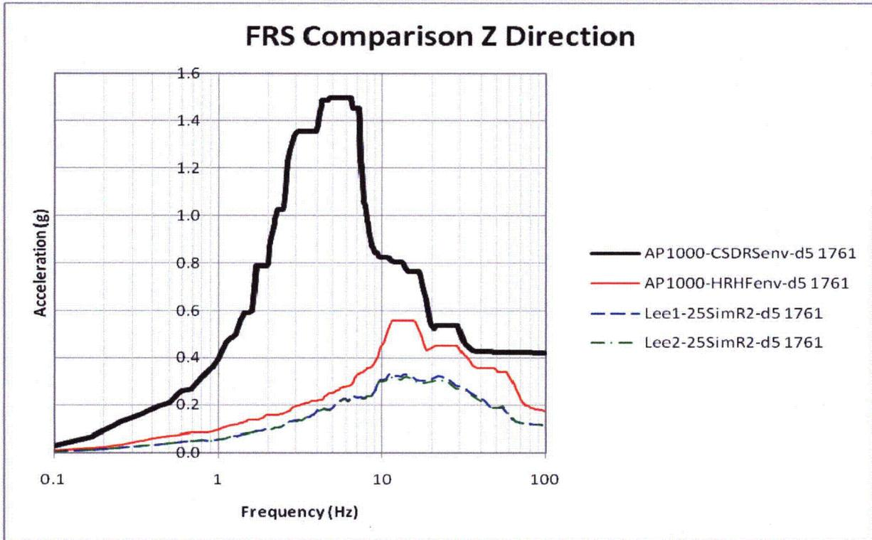
Figure 7-3: 3D FRS and AP1000 Envelope Comparison of Node 1761 in Z-Direction
