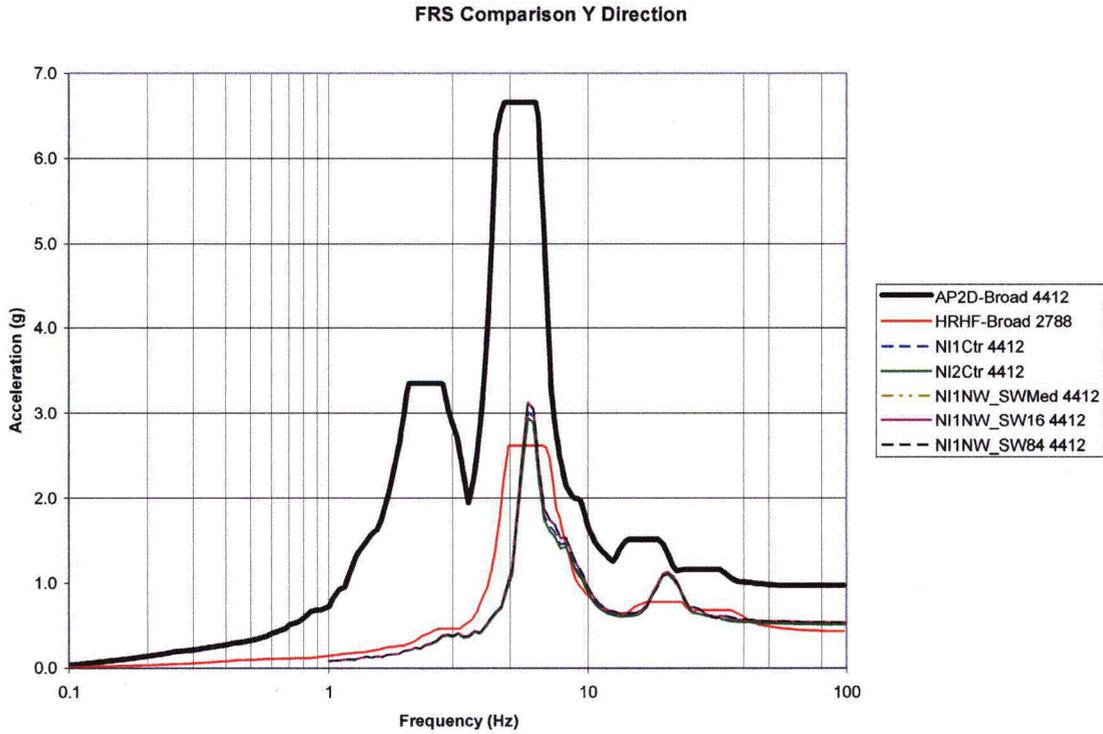
Figure C-9: 2D SW Backfill Parametric FRS Comparison of Node 4412 in Y-Direction
