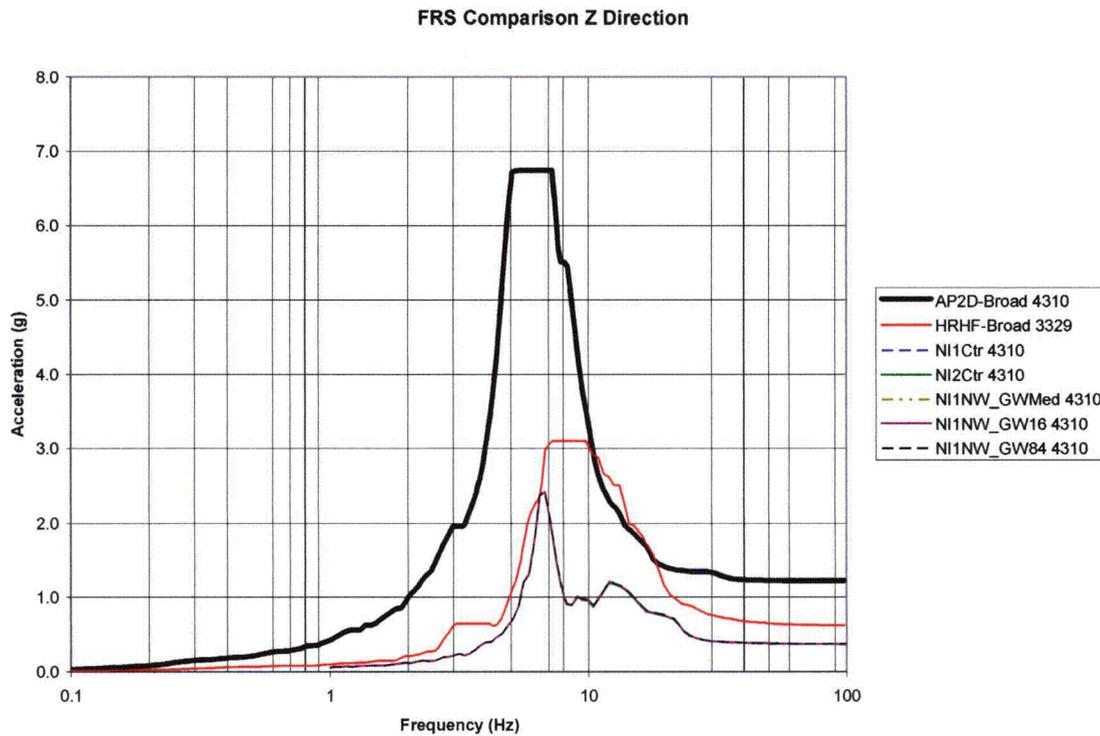
**Figure B-8: 2D GW Backfill Parametric FRS Comparison of Node 4310 in Z-Direction**
