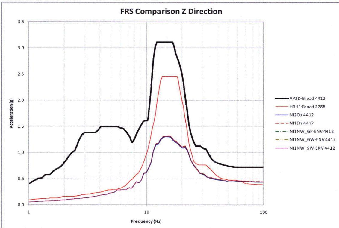
Figure 5-10: 2D Parametric FRS Comparison of Node 4412 in Z-Direction
