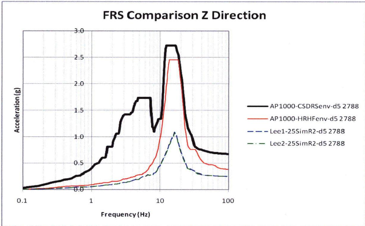
Figure 7-15: 3D FRS and AP1000 Envelope Comparison of Node 2788 in Z-Direction
