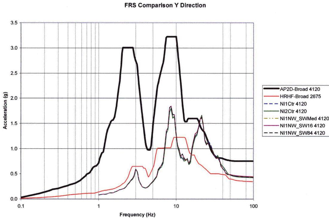
Figure C-5: 2D SW Backfill Parametric FRS Comparison of Node 4120 in Y-Direction
