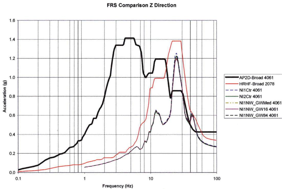
Figure B-4: 2D GW Backfill Parametric FRS Comparison of Node 4061 in Z-Direction
