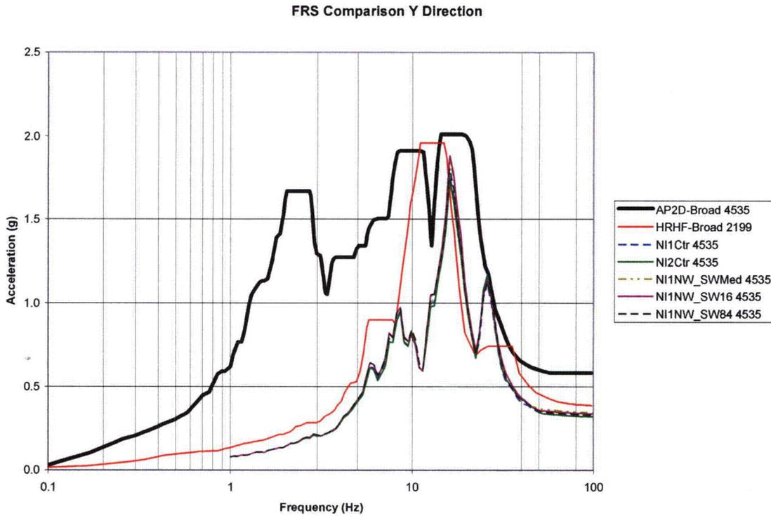
**Figure C-11: 2D SW Backfill Parametric FRS Comparison of Node 4535 in Y-Direction**
