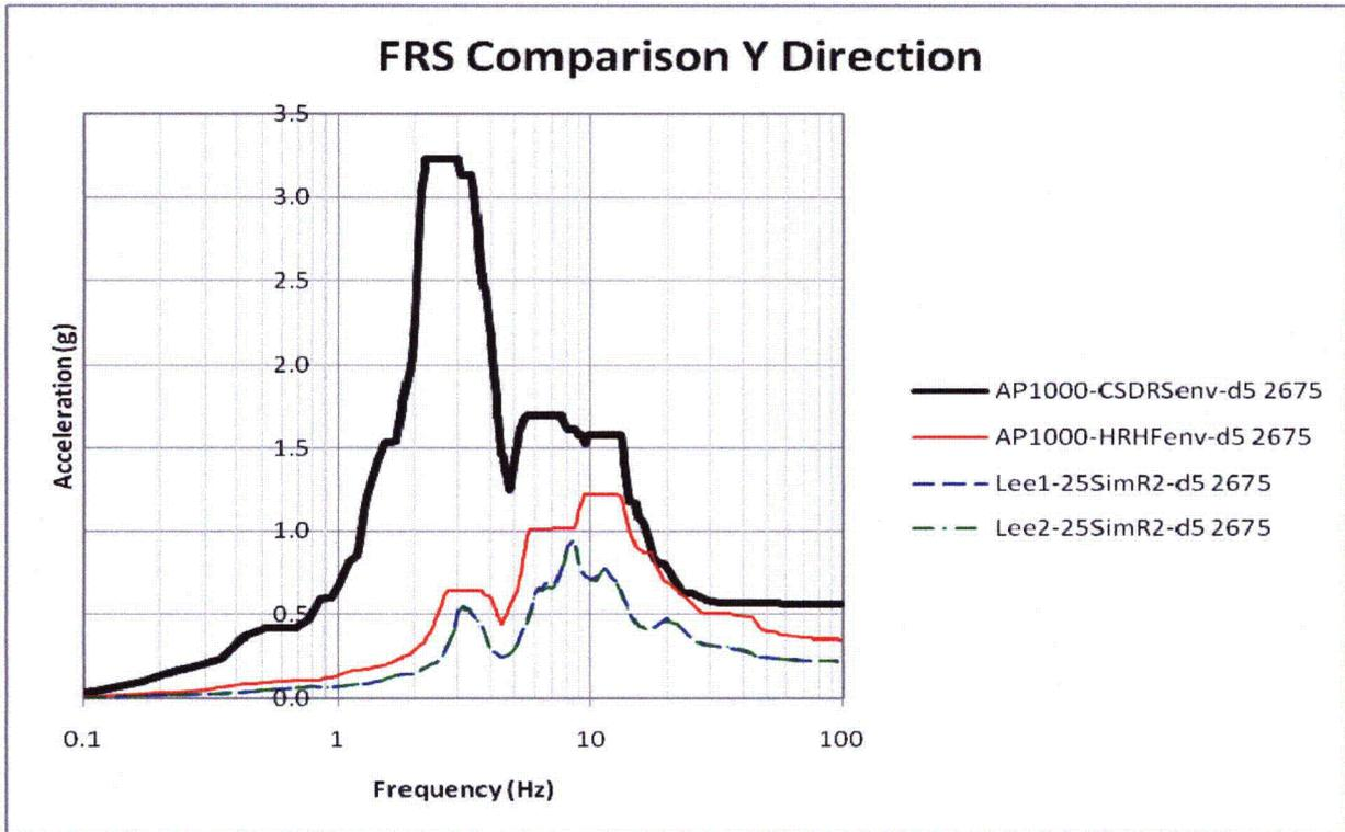
Figure 7-11: 3D FRS and AP1000 Envelope Comparison of Node 2675 in Y-Direction
