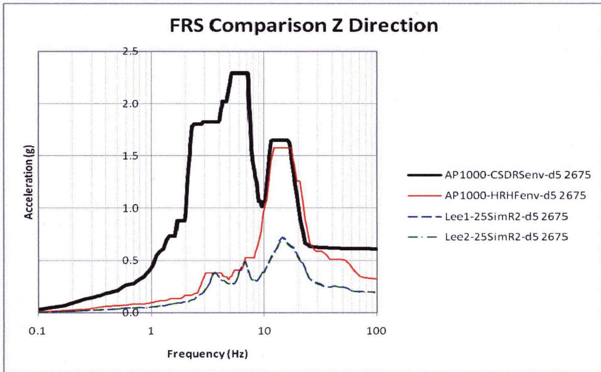
Figure 7-12: 3D FRS and AP1000 Envelope Comparison of Node 2675 in Z-Direction
