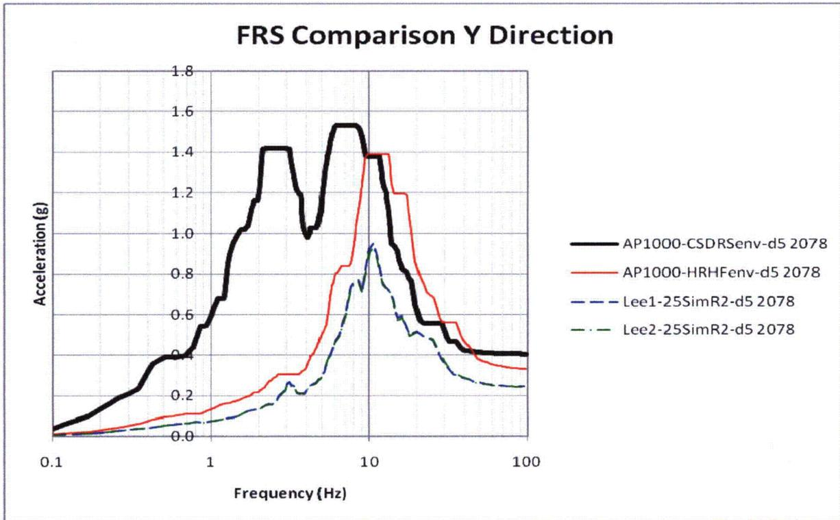
Figure 7-5: 3D FRS and AP1000 Envelope Comparison of Node 2078 in Y-Direction
