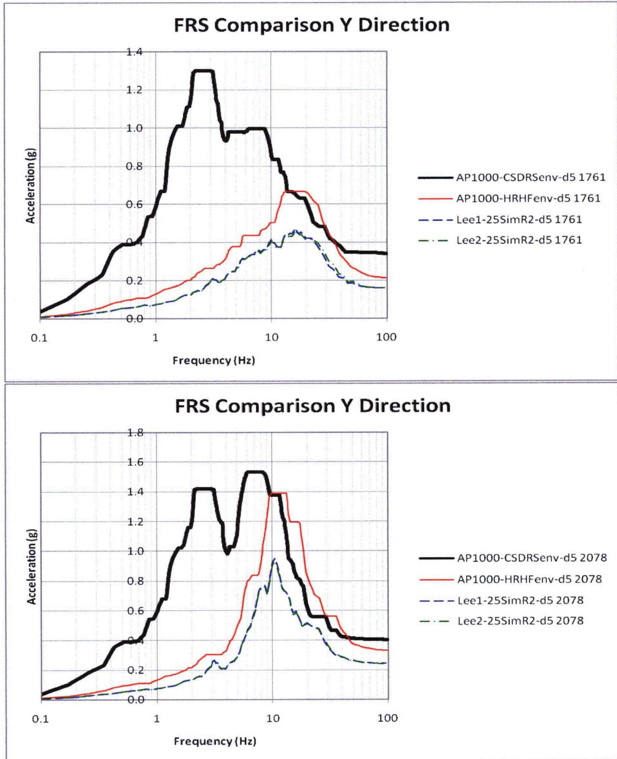
Figure 3.7-207a Comparison of 3D FRS and AP1000 Envelope (Y-Direction, Nodes 1761 and 2078)
