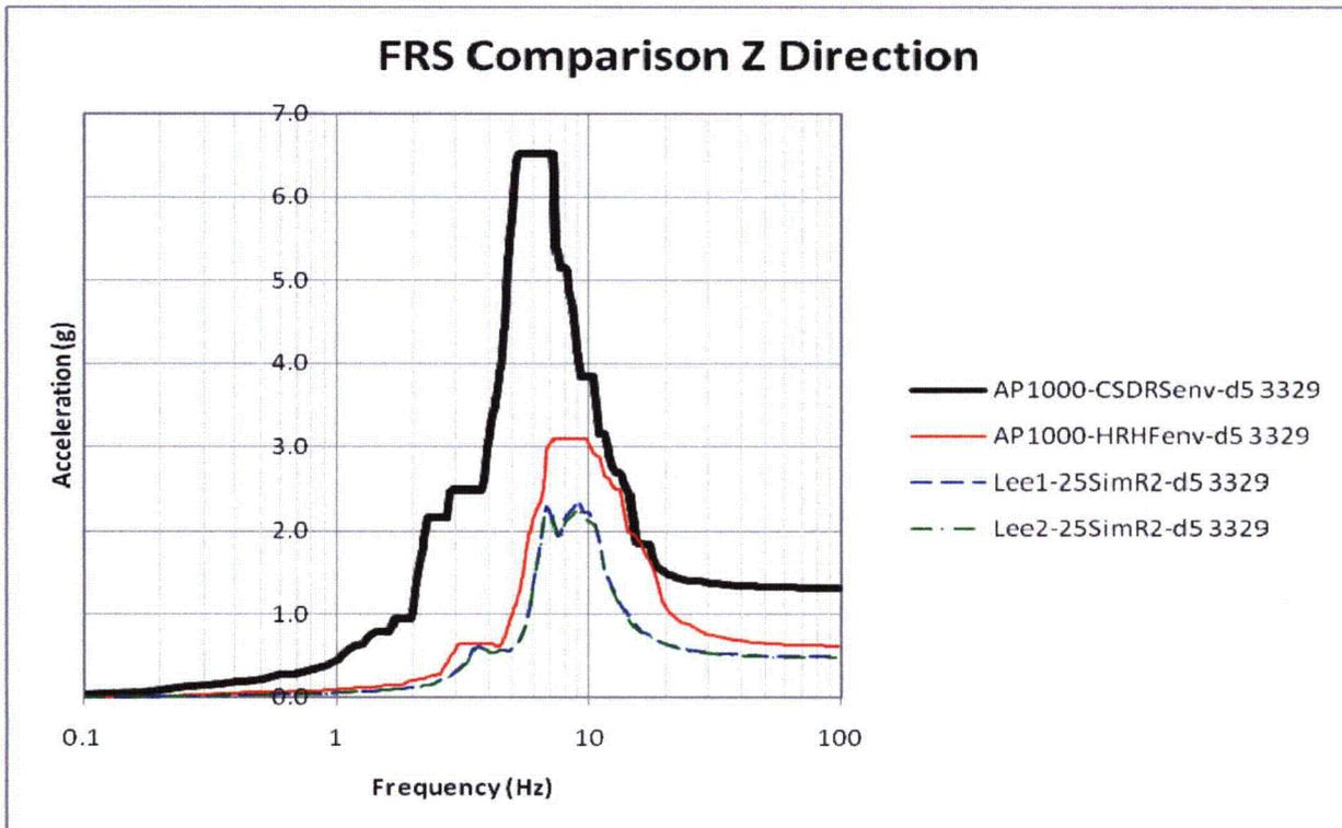
Figure 7-18: 3D FRS and AP1000 Envelope Comparison of Node 3329 in Z-Direction
