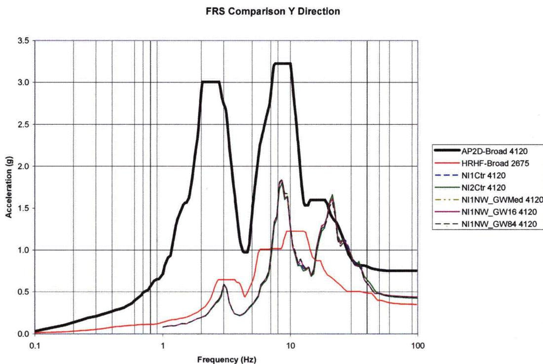
Figure B-5: 2D GW Backfill Parametric FRS Comparison of Node 4120 in Y-Direction
