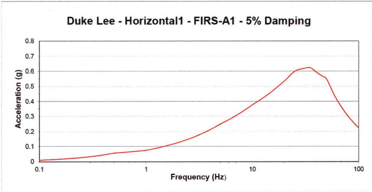
Figure 3-2: Duke Lee North-South Foundation Input Response Spectra at 5% Damping
