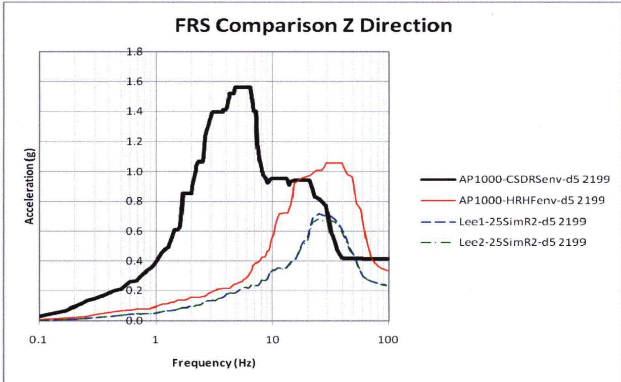
Figure 7-9: 3D FRS and AP1000 Envelope Comparison of Node 2199 in Z-Direction
