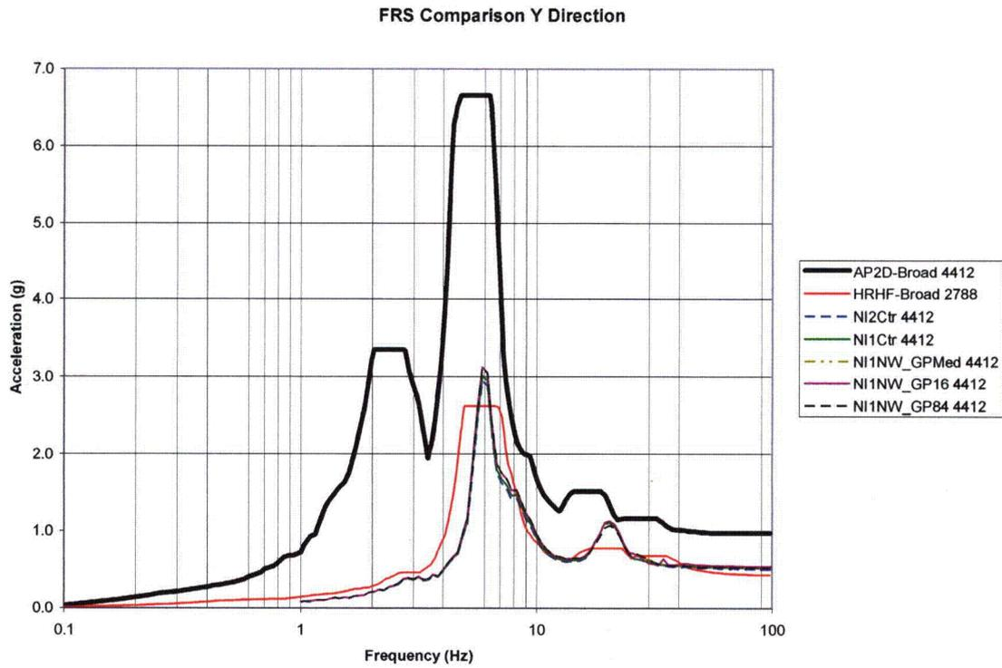
**Figure A-9: 2D GP Backfill Parametric FRS Comparison of Node 4412 in Y-Direction**
