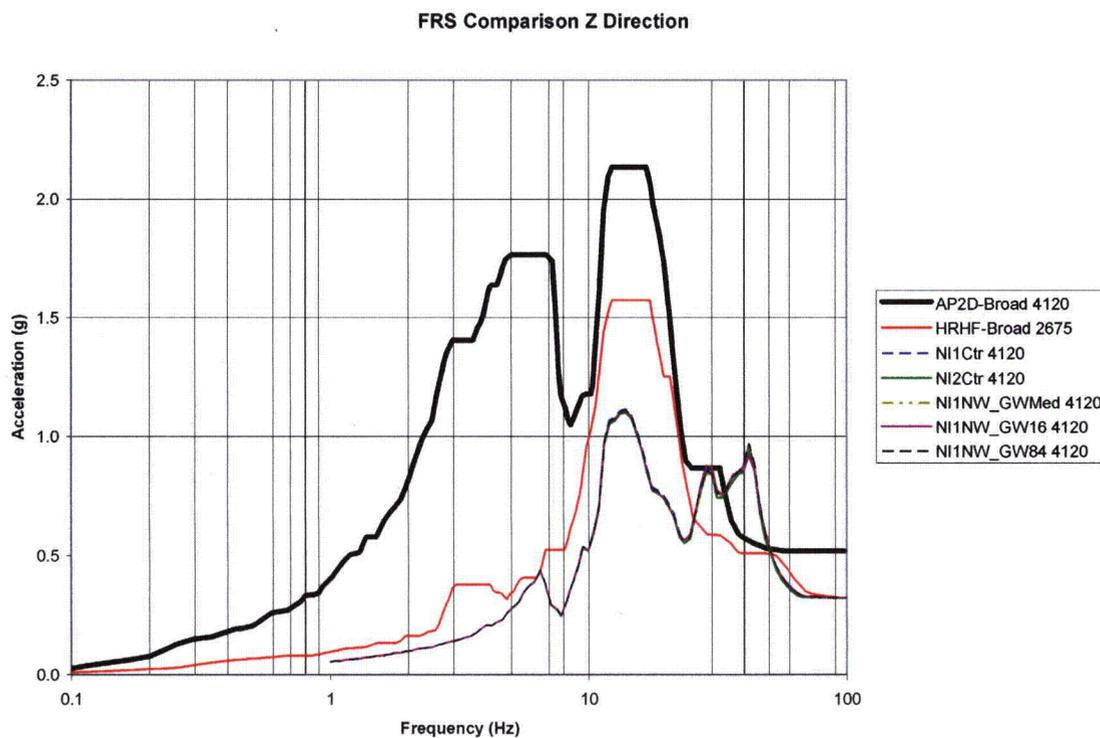
Figure B-6: 2D GW Backfill Parametric FRS Comparison of Node 4120 in Z-Direction
