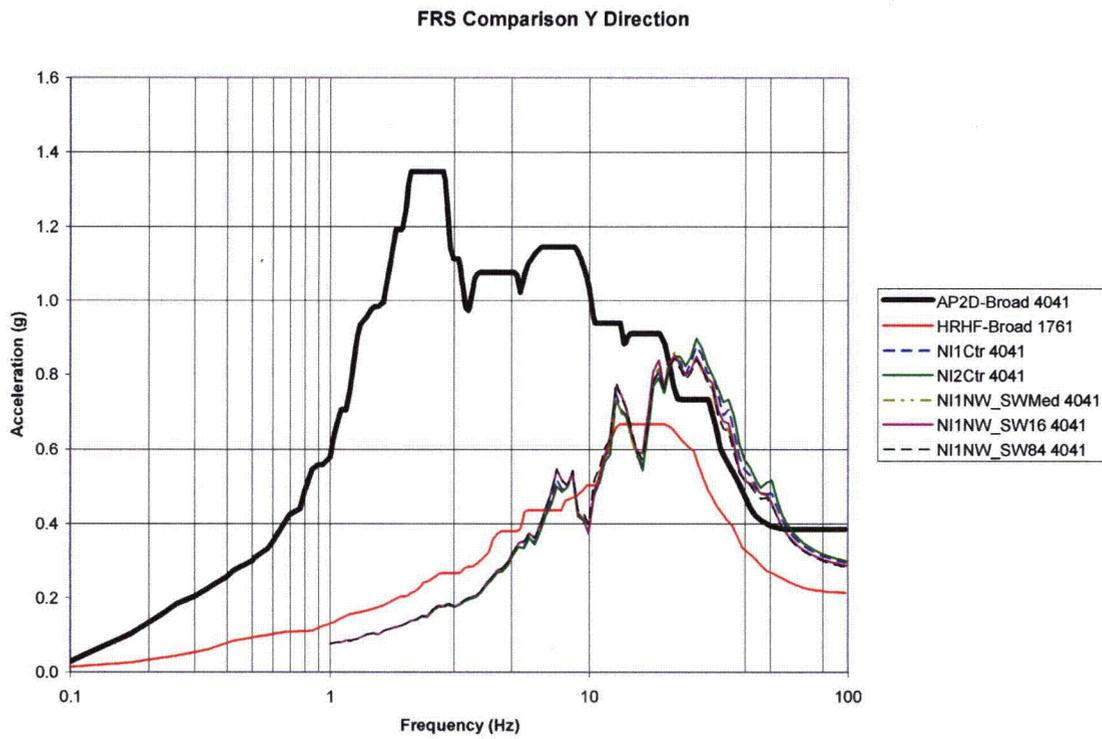
Figure C-1: 2D SW Backfill Parametric FRS Comparison of Node 4041 in Y-Direction
