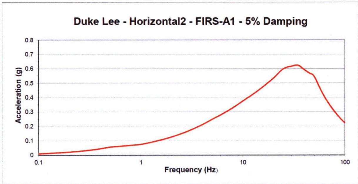
Figure 3-3: Duke Lee East-West Foundation Input Response Spectra at 5% Damping
