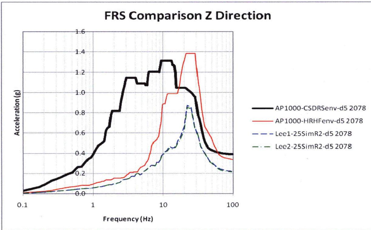
Figure 7-6: 3D FRS and AP1000 Envelope Comparison of Node 2078 in Z-Direction
