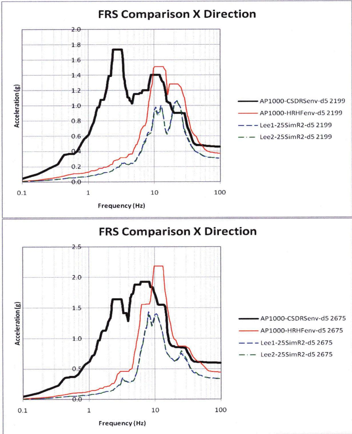
**Figure 3.7-206b Comparison of 3D FRS and AP1000 Envelope (X-Direction, Nodes 2199 and 2675)**
