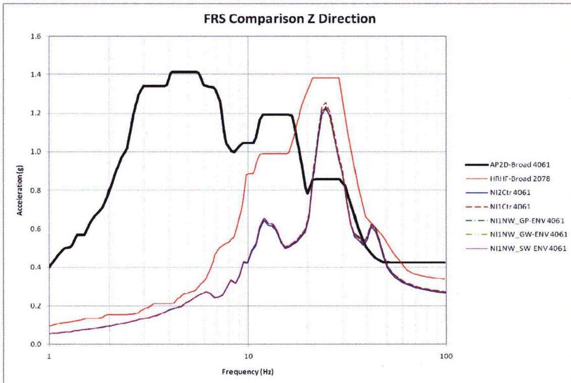
Figure 5-4: 2D Parametric FRS Comparison of Node 4061 in Z-Direction
