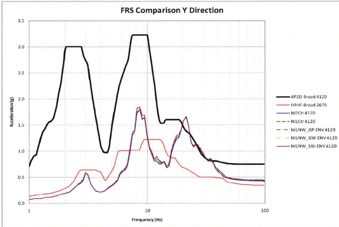
Figure 5-5: 2D Parametric FRS Comparison of Node 4120 in Y-Direction
