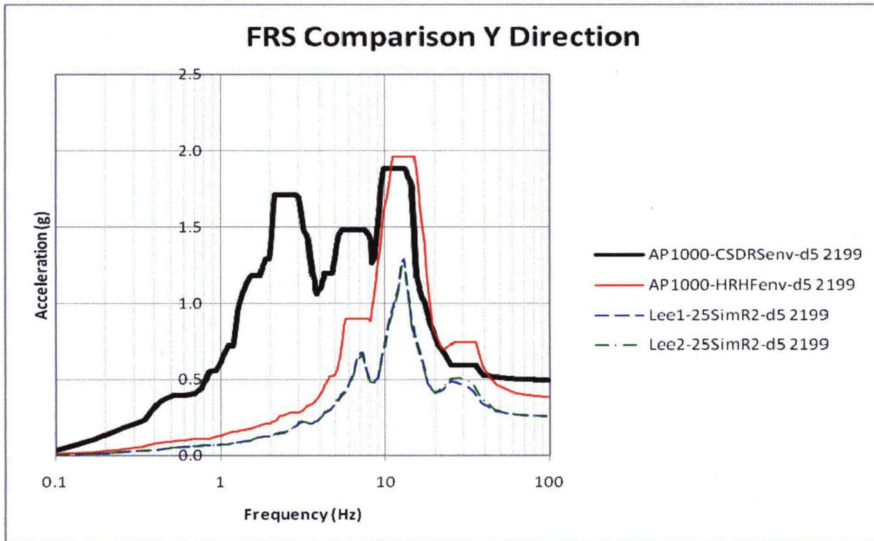
Figure 7-8: 3D FRS and AP1000 Envelope Comparison of Node 2199 in Y-Direction
