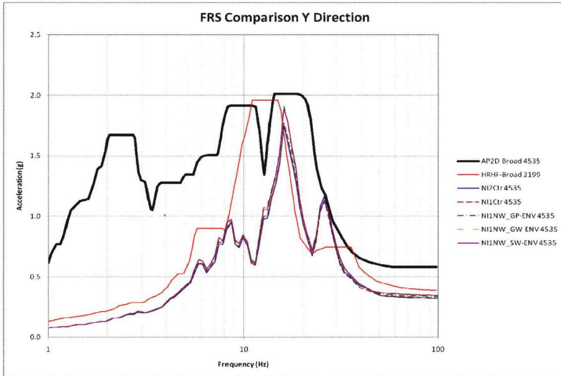
Figure 5-11: 2D Parametric FRS Comparison of Node 4535 in Y-Direction
