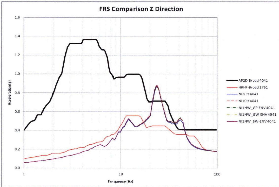
Figure 5-2: 2D Parametric FRS Comparison of Node 4041 in Z-Direction
