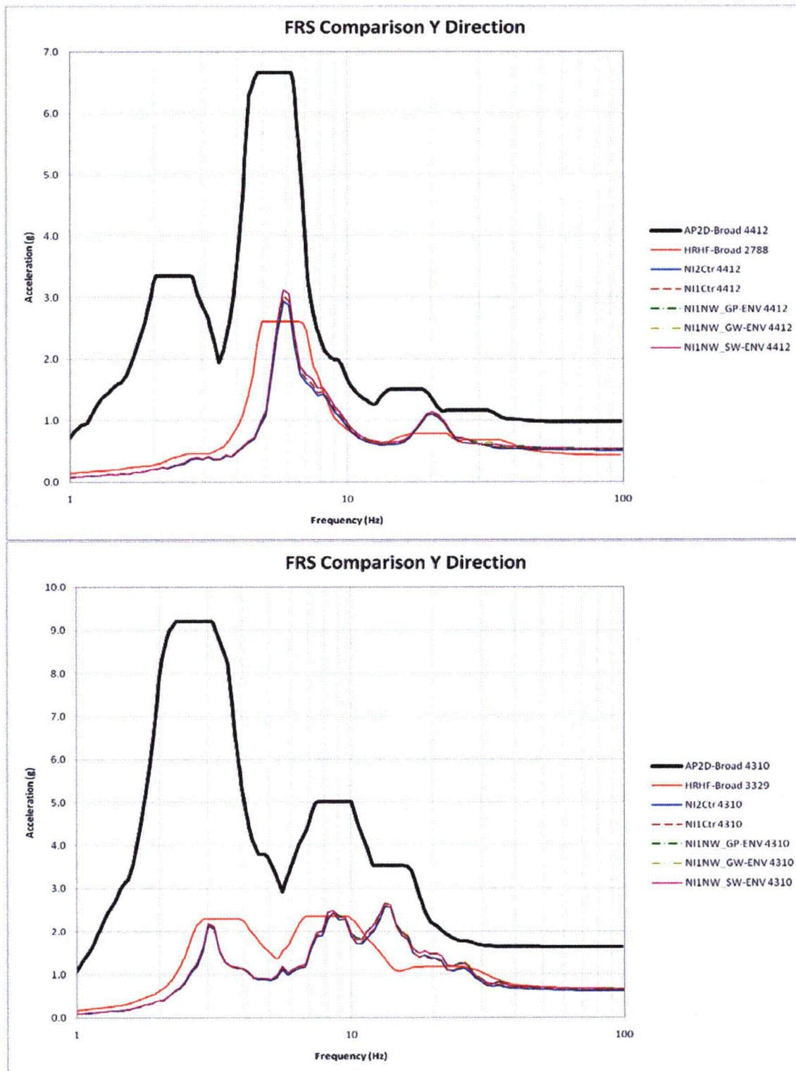
Figure 3.7-204c Comparison of 2D FRS and AP1000 Envelope (Y-Direction, Nodes 4412 and 4310)
