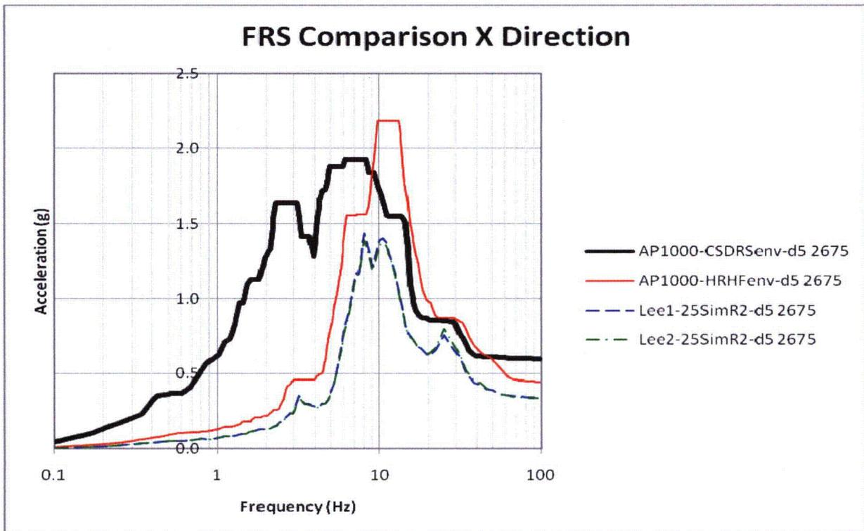
Figure 7-10: 3D FRS and AP1000 Envelope Comparison of Node 2675 in X-Direction
