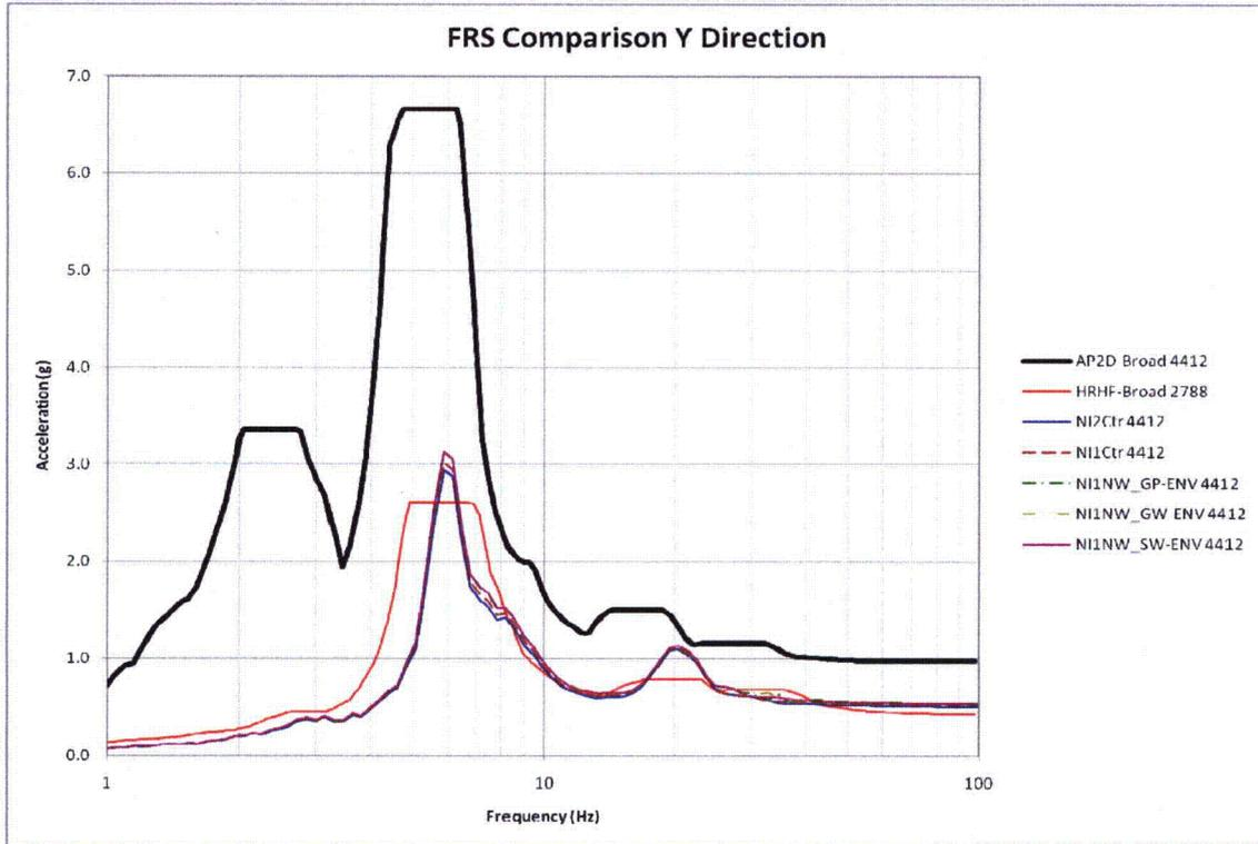
Figure 5-9: 2D Parametric FRS Comparison of Node 4412 in Y-Direction
