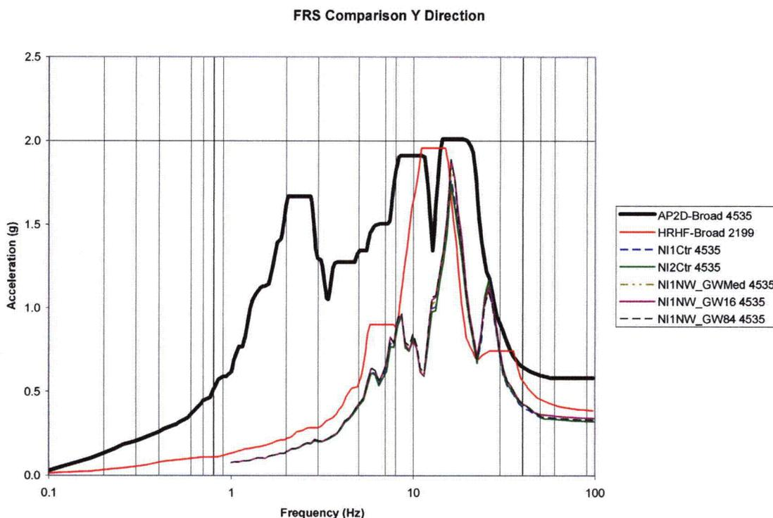
**Figure B-11: 2D GW Backfill Parametric FRS Comparison of Node 4535 in Y-Direction**
