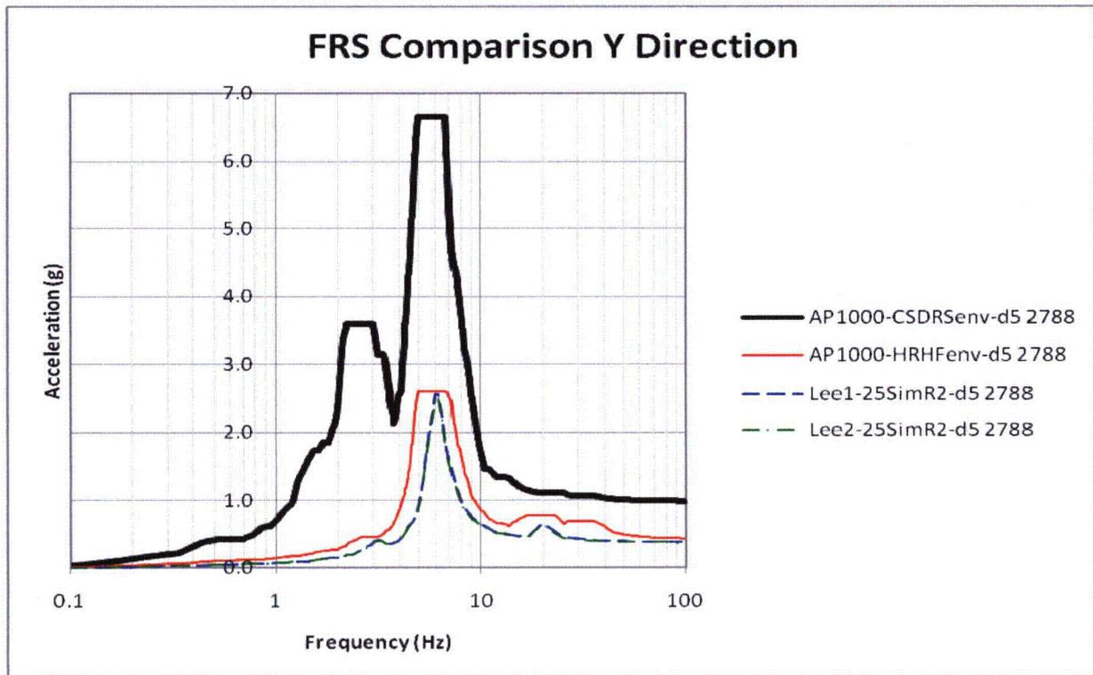
Figure 7-14: 3D FRS and AP1000 Envelope Comparison of Node 2788 in Y-Direction
