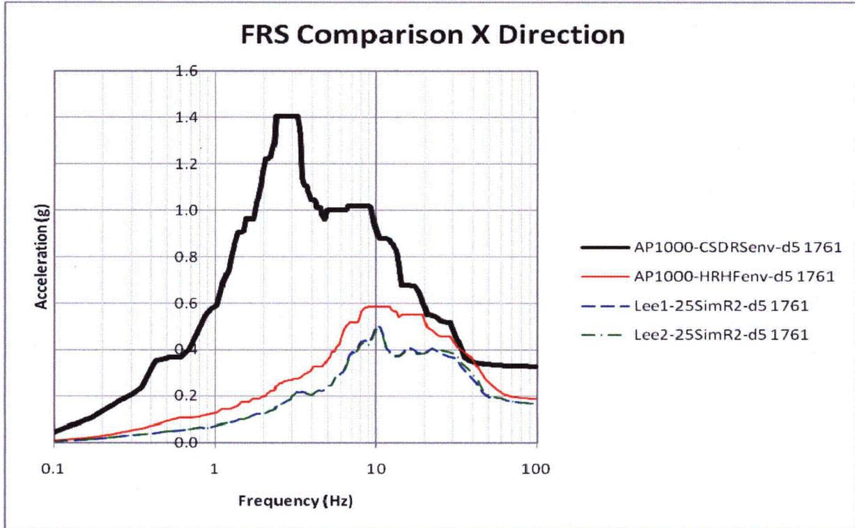
Figure 7-1: 3D FRS and AP1000 Envelope Comparison of Node 1761 in X-Direction
