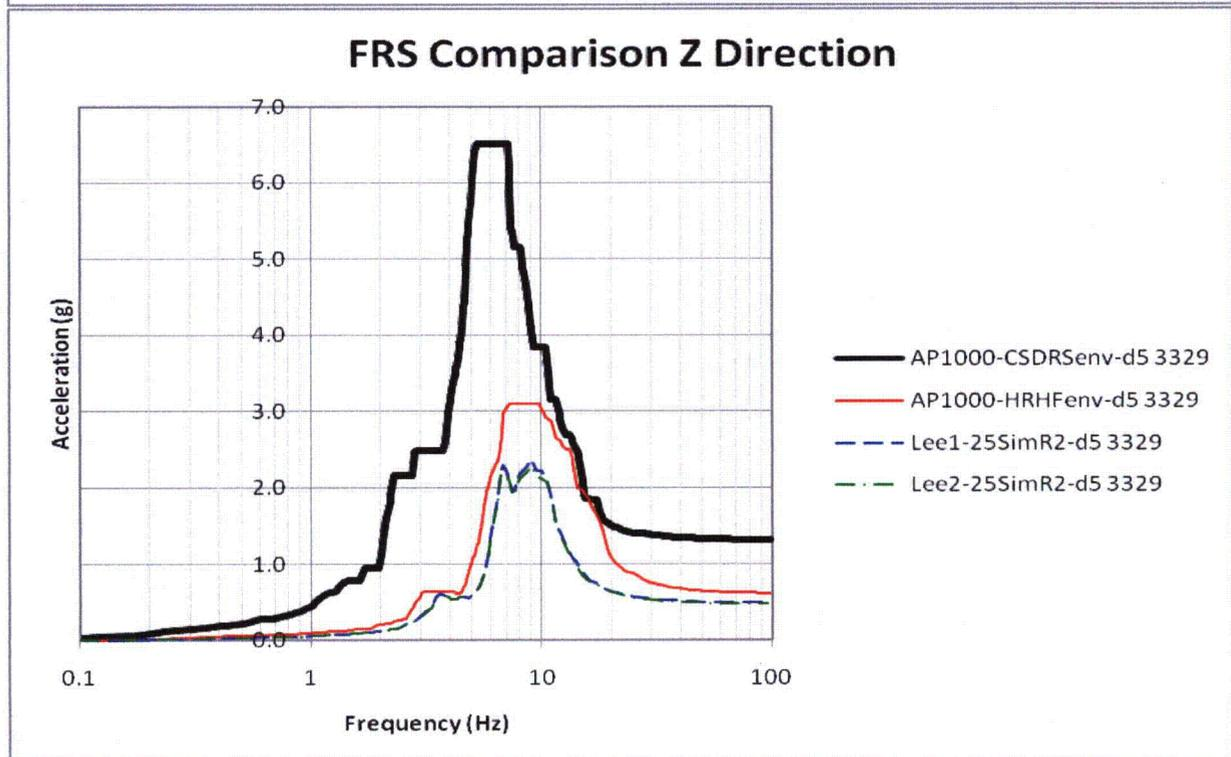
**Figure 3.7-208c Comparison of 3D FRS and AP1000 Envelope (Z-Direction, Nodes 2788 and 3329)**
