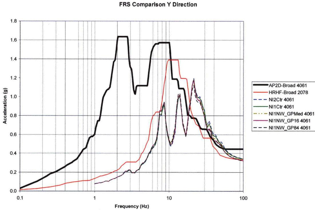
**Figure A-3: 2D GP Backfill Parametric FRS Comparison of Node 4061 in Y-Direction**
