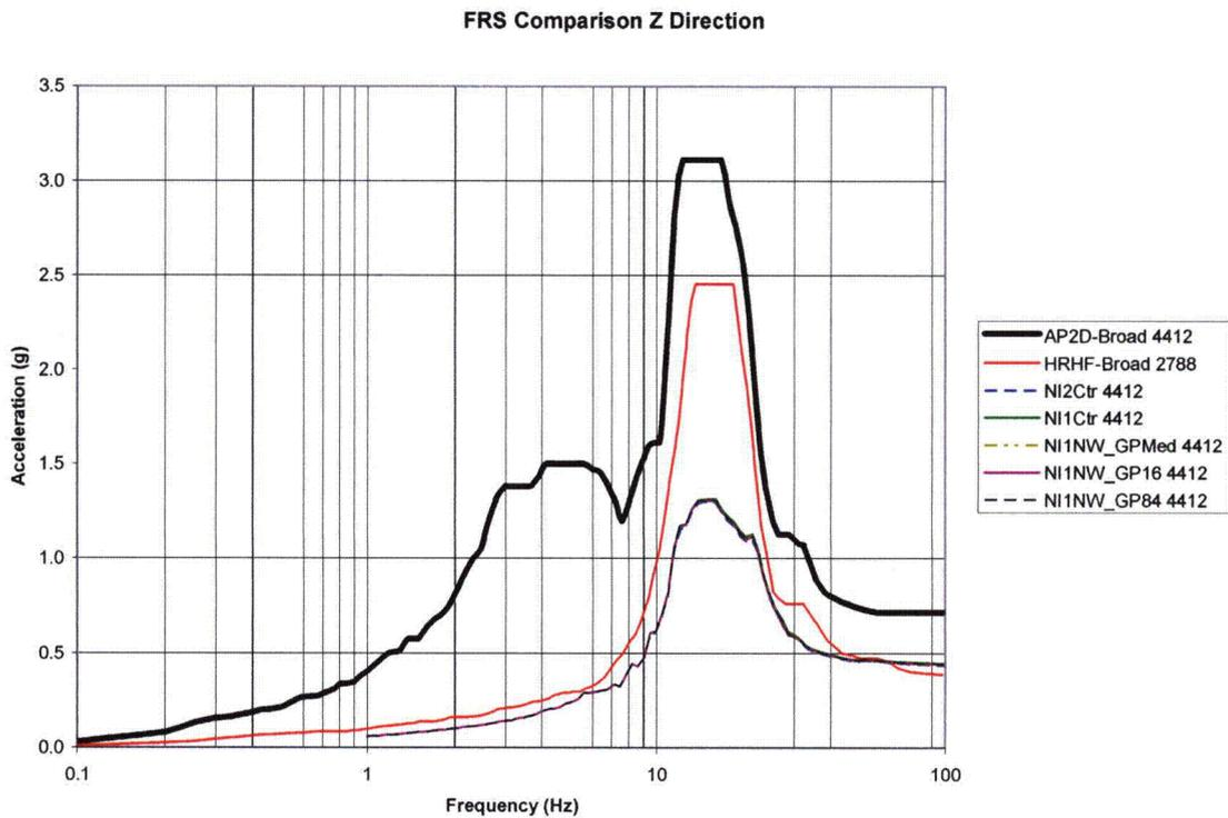
**Figure A-10: 2D GP Backfill Parametric FRS Comparison of Node 4412 in Z-Direction**
