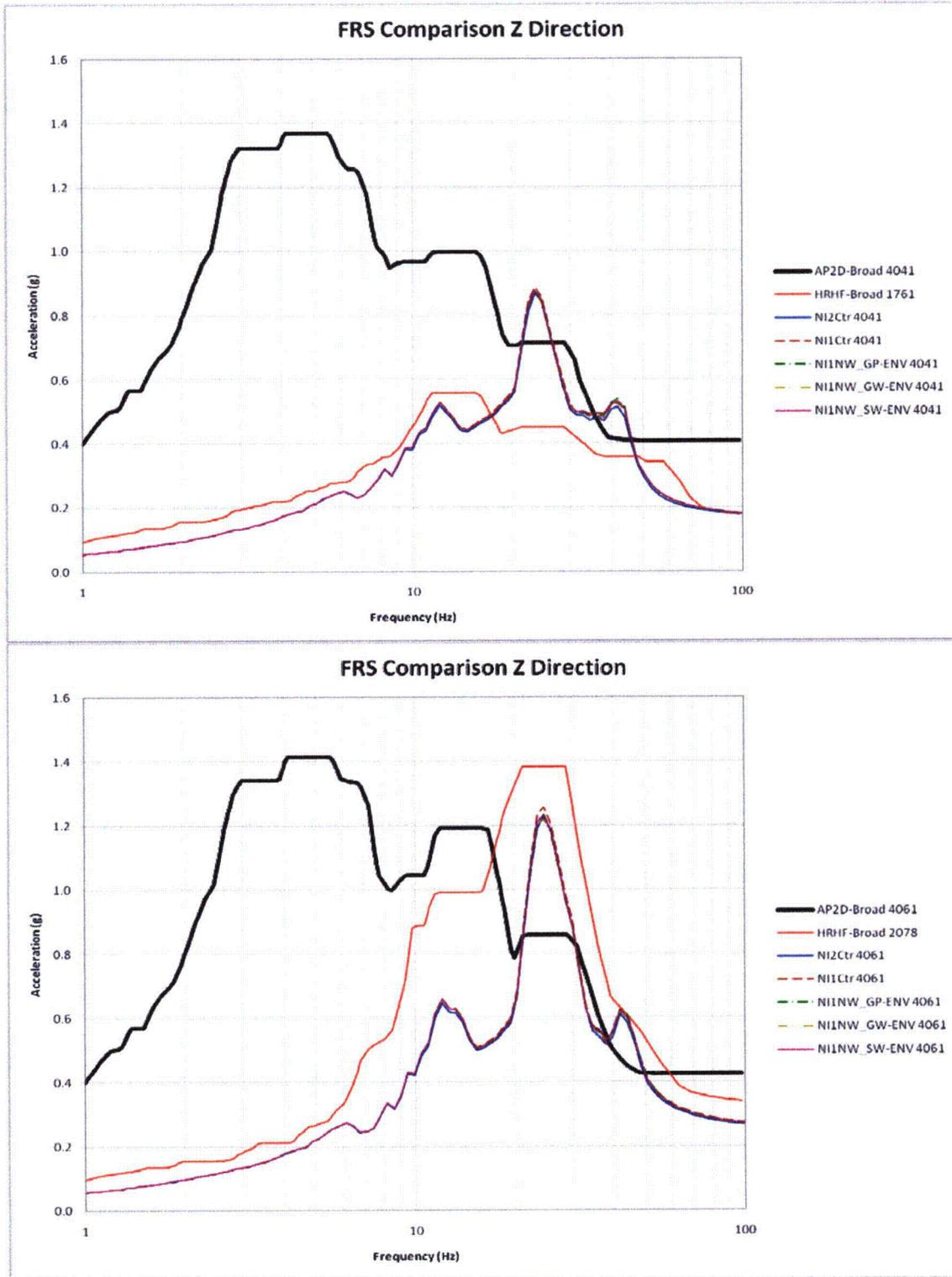
**Figure 3.7-205a Comparison of 2D FRS and AP1000 Envelope (Z-Direction, Nodes 4041 and 4061)**
