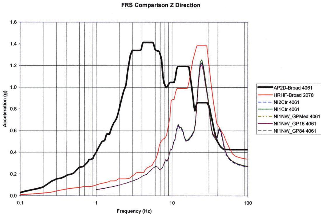
**Figure A-4: 2D GP Backfill Parametric FRS Comparison of Node 4061 in Z-Direction**
