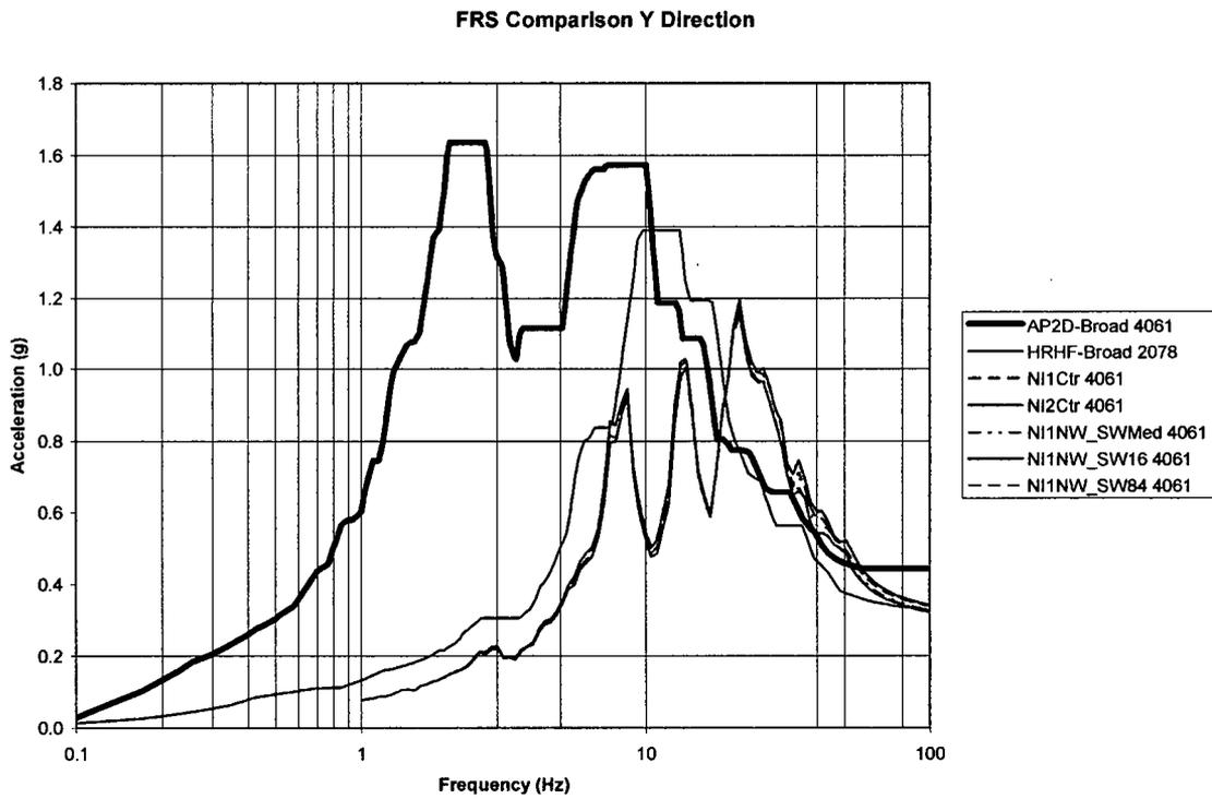
**Figure C-3: 2D SW Backfill Parametric FRS Comparison of Node 4061 in Y-Direction**
