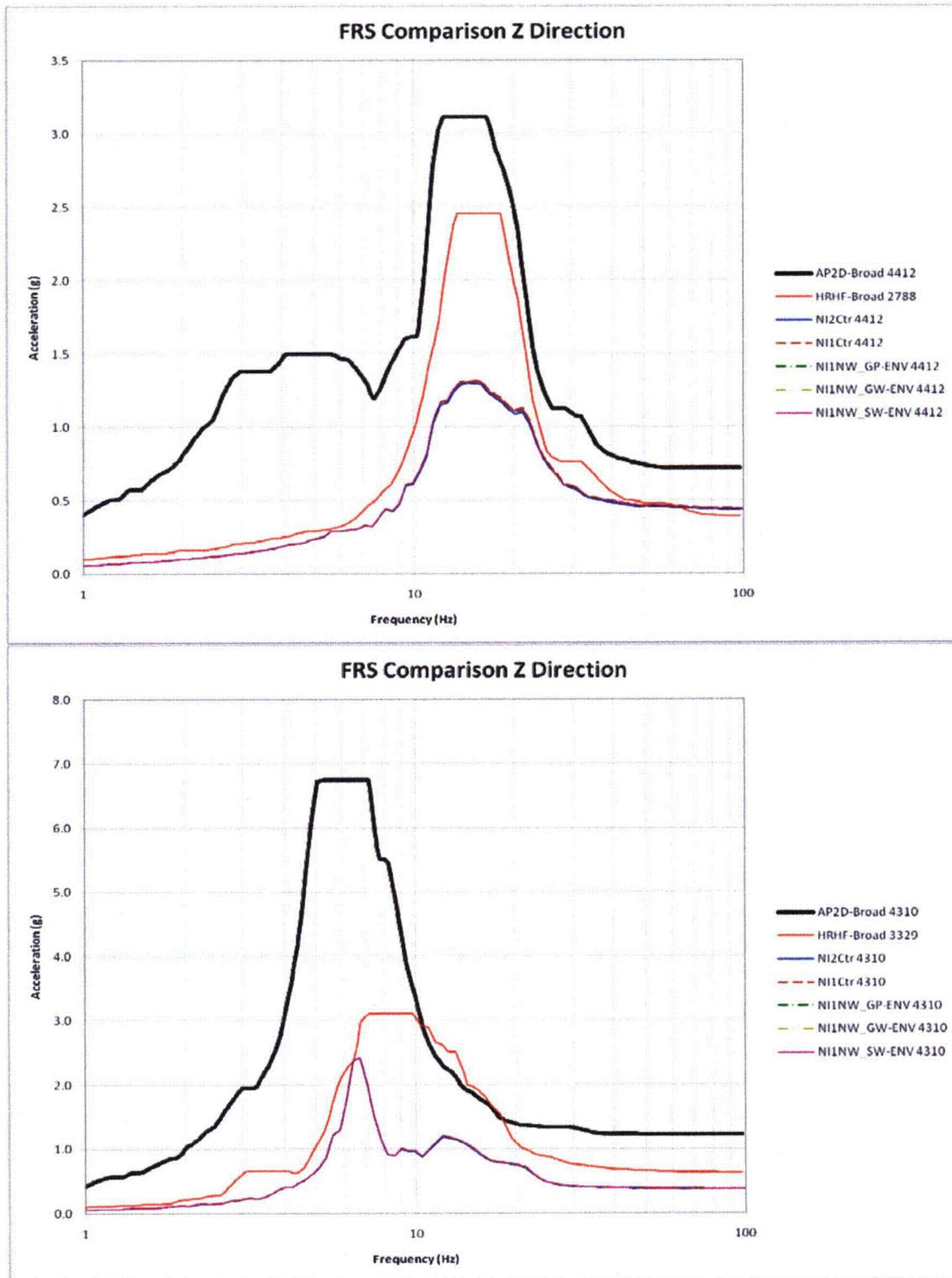
Figure 3.7-205c Comparison of 2D FRS and AP1000 Envelope (Z-Direction, Nodes 4412 and 4310)
