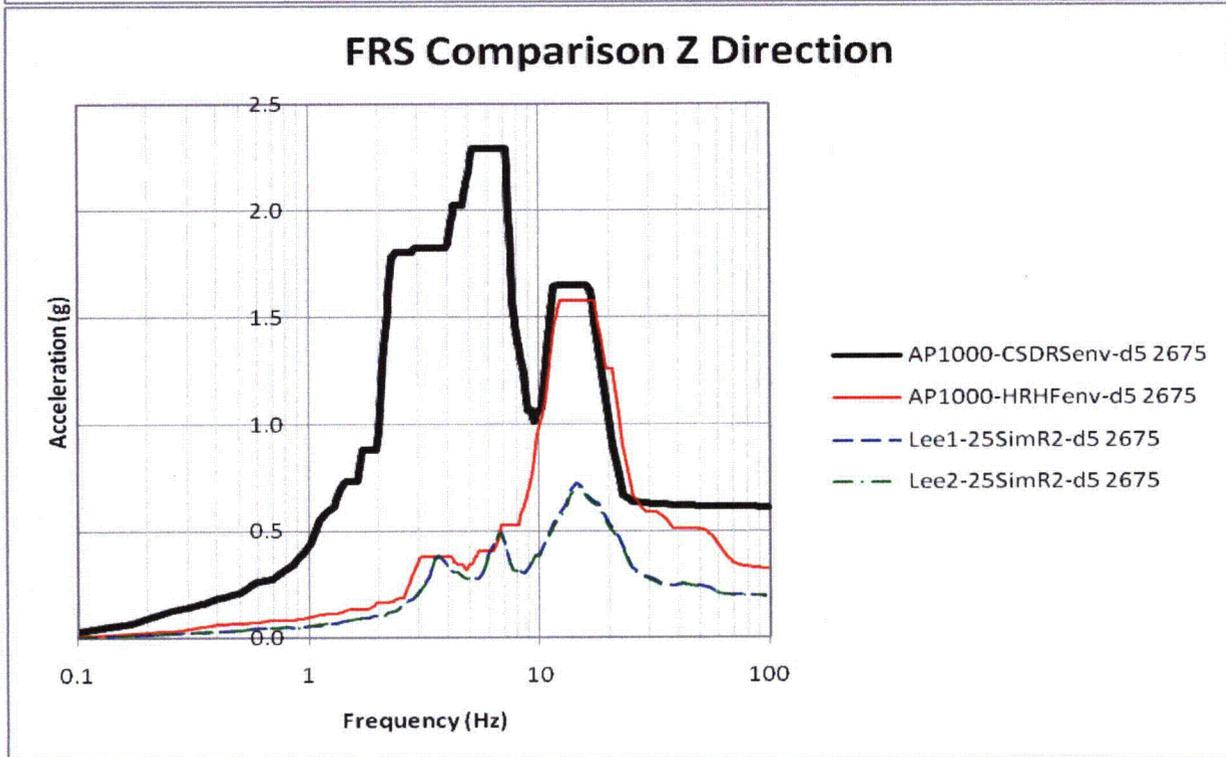
**Figure 3.7-208b Comparison of 3D FRS and AP1000 Envelope (Z-Direction, Nodes 2199 and 2675)**
