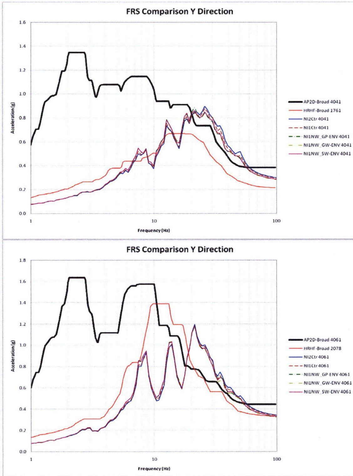
**Figure 3.7-204a Comparison of 2D FRS and AP1000 Envelope (Y-Direction, Nodes 4041 and 4061)**
