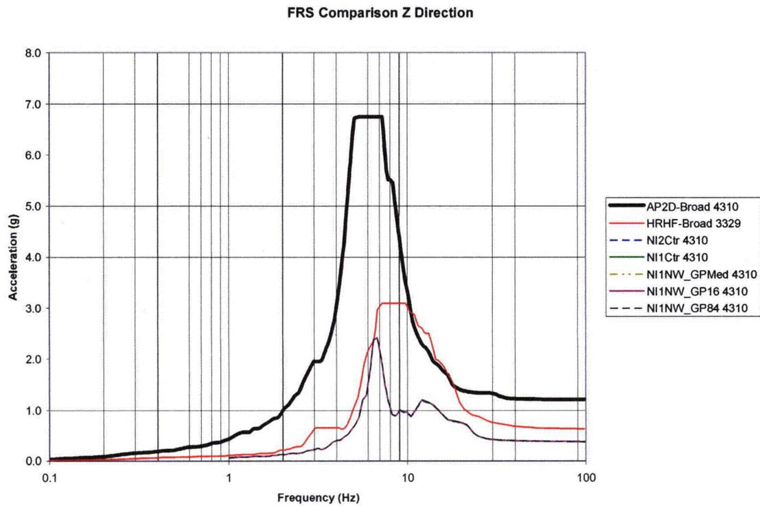
Figure A-8: 2D GP Backfill Parametric FRS Comparison of Node 4310 in Z-Direction
