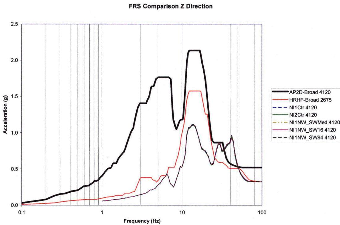
Figure C-6: 2D SW Backfill Parametric FRS Comparison of Node 4120 in Z-Direction
