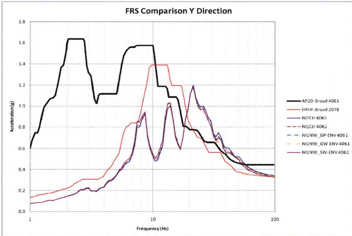
Figure 5-3: 2D Parametric FRS Comparison of Node 4061 in Y-Direction
