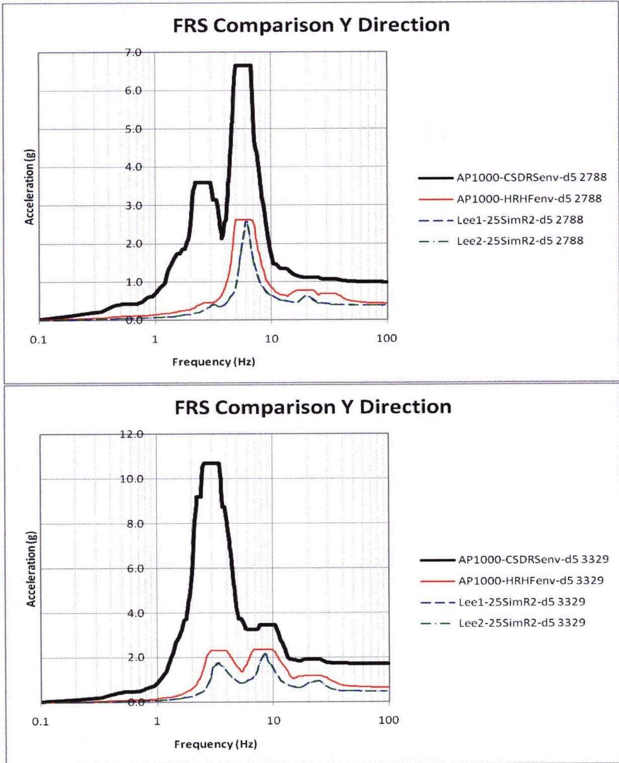
**Figure 3.7-207c Comparison of 3D FRS and AP1000 Envelope (Y-Direction, Nodes 2788 and 3329)**
