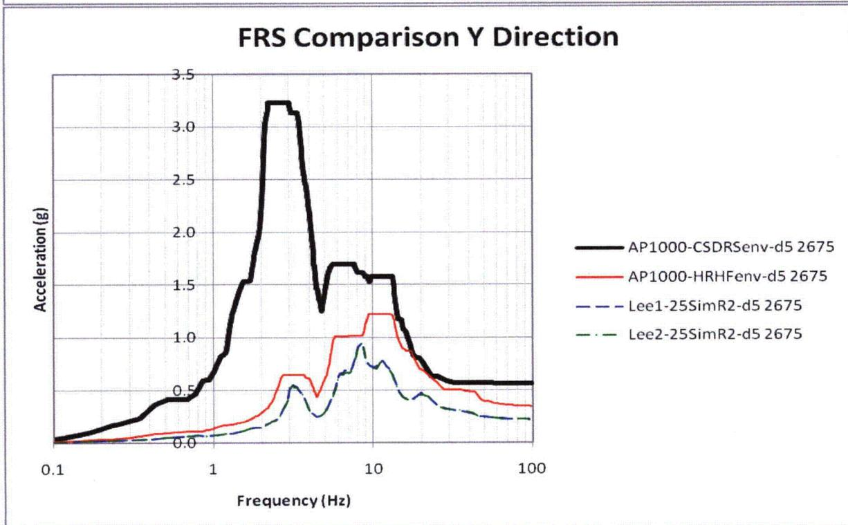
**Figure 3.7-207b Comparison of 3D FRS and AP1000 Envelope (Y-Direction, Nodes 2199 and 2675)**
