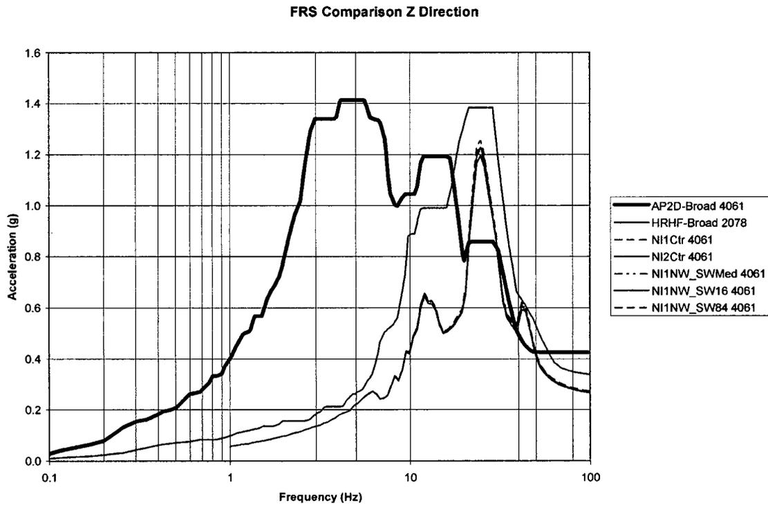
**Figure C-4: 2D SW Backfill Parametric FRS Comparison of Node 4061 in Z-Direction**
