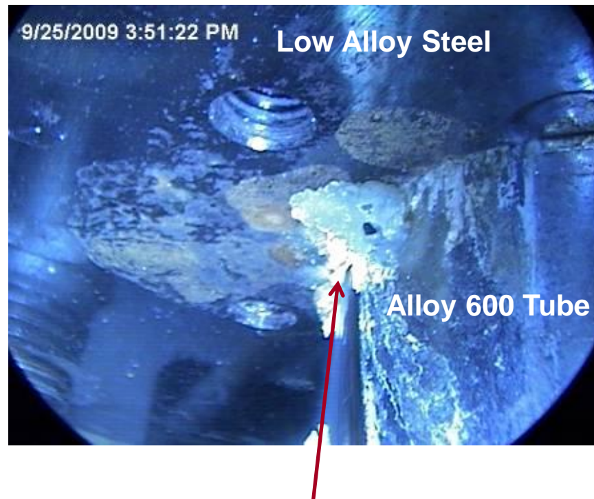
BMN Test 5: 0.006 GPM leakage Boric Acid Deposits Visible after 24 hours
