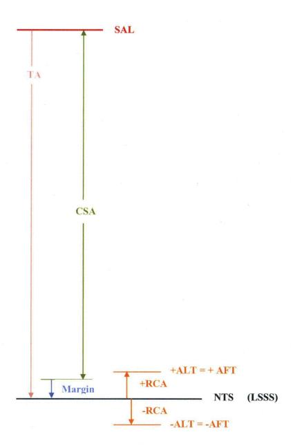
Figure 3-1 Westinghouse Setpoint Parameter Relationship Diagram (Increasing Function)
