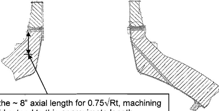
For the ~ 8" axial length for  $0.75\sqrt{Rt}$ , machining would extend to this approximate length.
