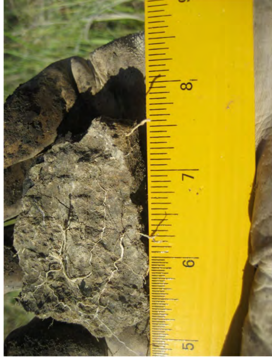
Fig. A.71. Digging block sample in thicker CCL.
