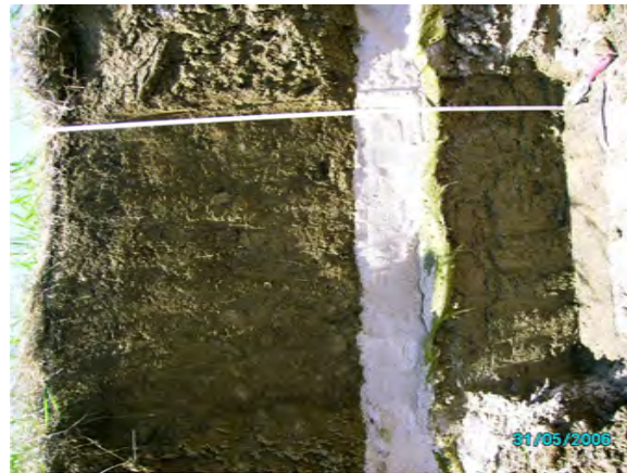
Fig. A.56. Roots extending into course layer in AO1.
