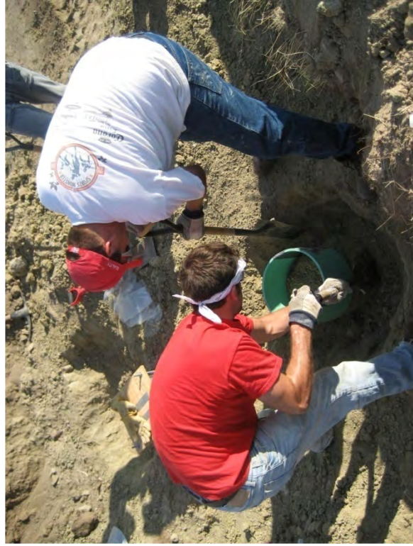
Fig. A.14. Filling SDRI, inner cap visible.
