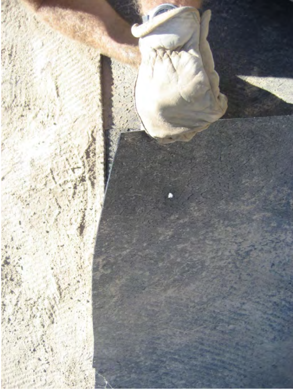
Fig A.6. Constructed defect in GM.
