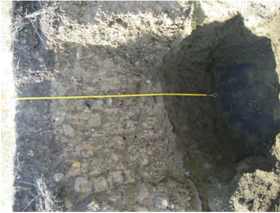
Fig. A.70. Thicker (3 ft) CCL profile (desiccated across profile).
