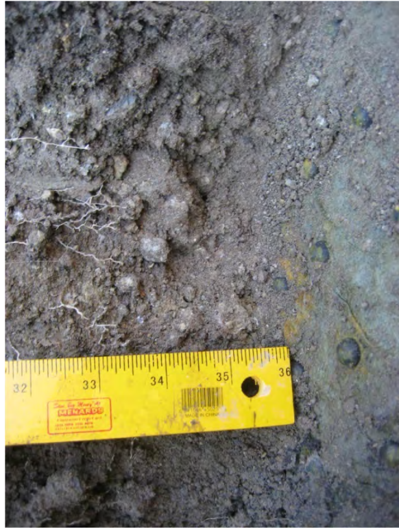
Fig. A.70. Thicker (3 ft) CCL profile (desiccated across profile).
