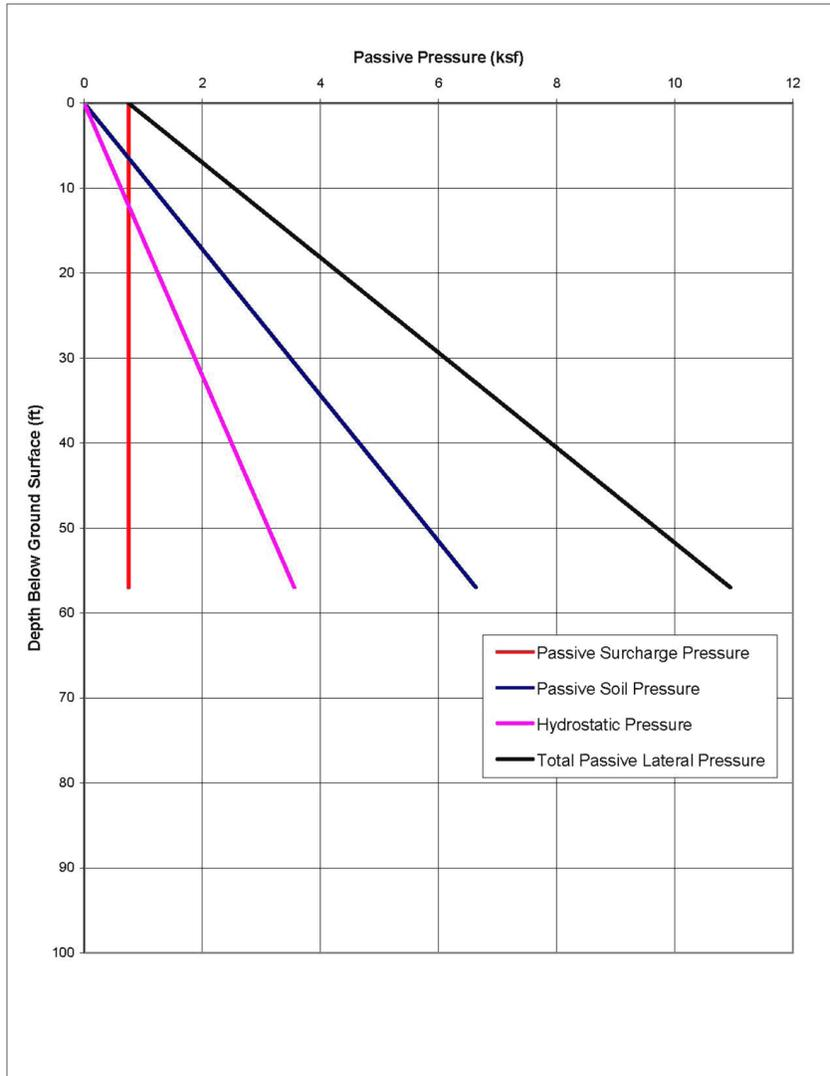
Figure 3H.3-4 Passive Lateral Earth Pressure on the RWB Walls
