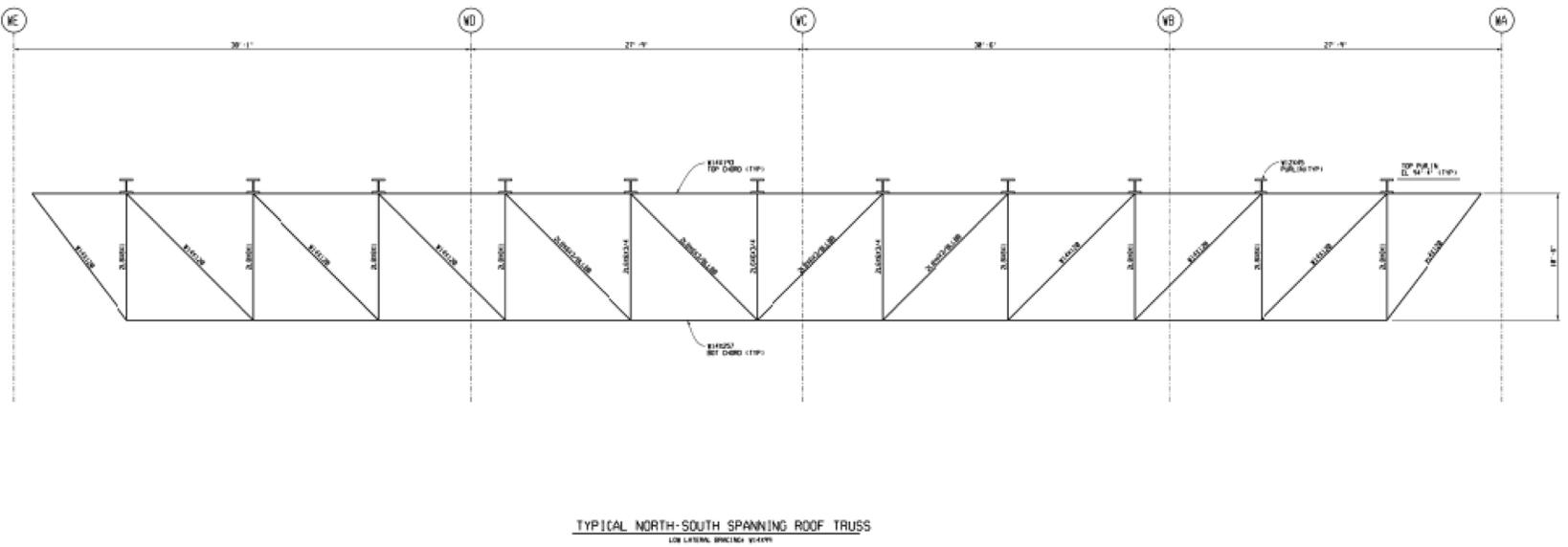
Figure 3H.3-49 Typical North-South Spanning Truss Between Column Lines WA-WE (Elevation View)
