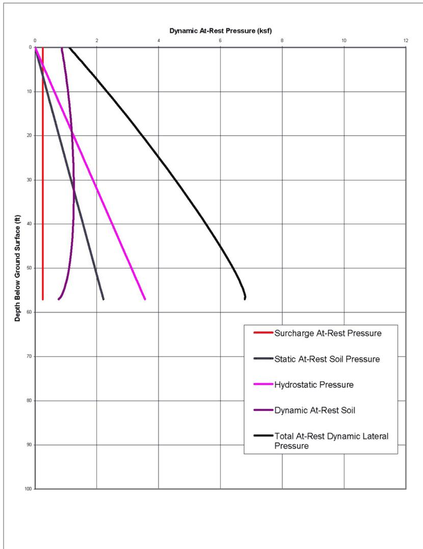
Figure 3H.3-2 Dynamic At-Rest Lateral Earth Pressure on the RWB Walls
