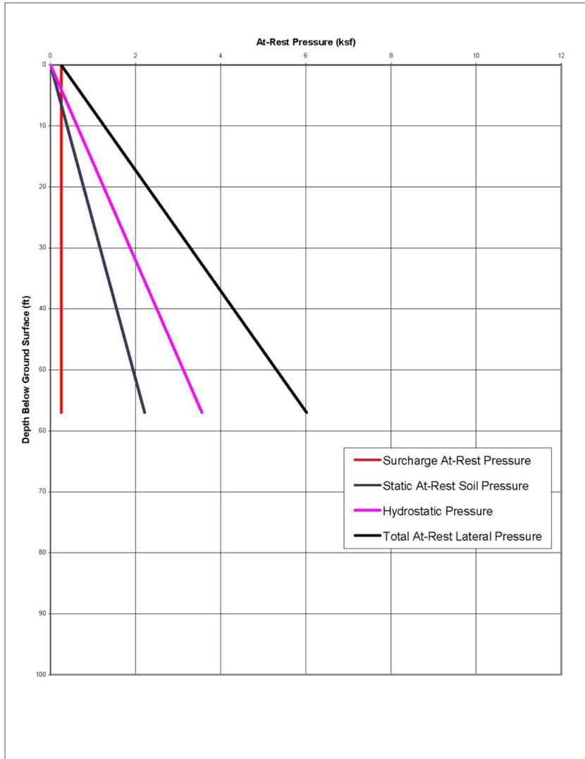
Figure 3H.3-1 At-Rest Lateral Earth Pressure on the RWB Walls
