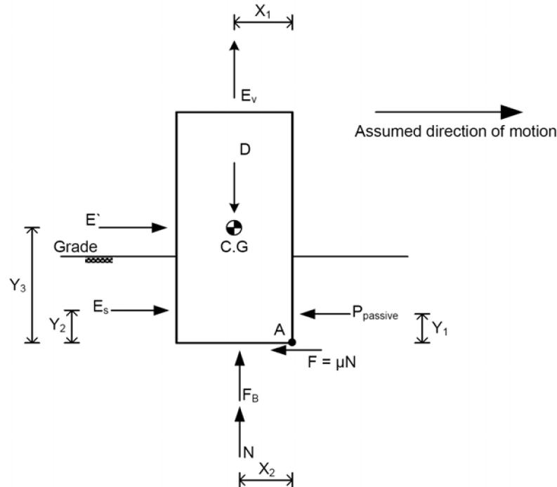
Factors of Safety against Sliding and Overturning about point A are calculated as follows:
