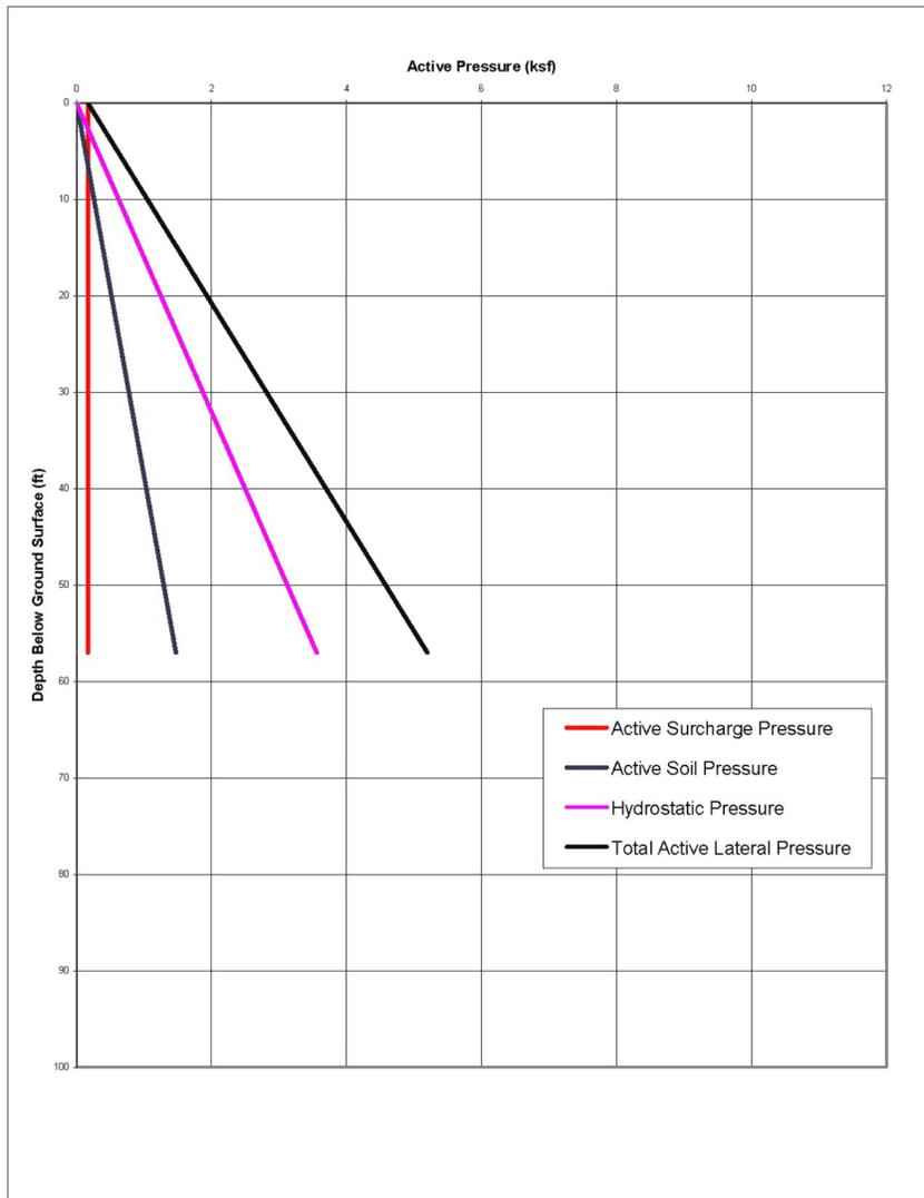
Figure 3H.3-3 Active Lateral Earth Pressure on the RWB Walls
