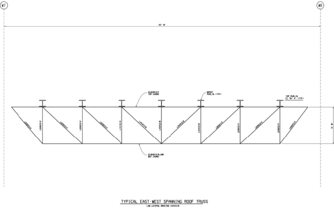
Figure 3H.3-48 Typical East-West Spanning Roof Truss Between Column Lines W7-W8 (Elevation View)
