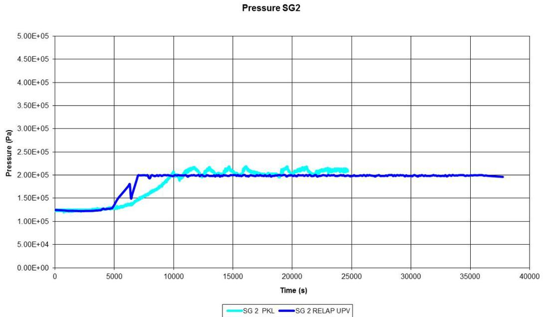
**Figure 14: Pressure in the SG2 Secondary Side**
