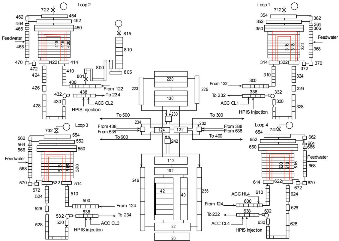
Figure 4: RELAP5 nodalization of PKL facility
