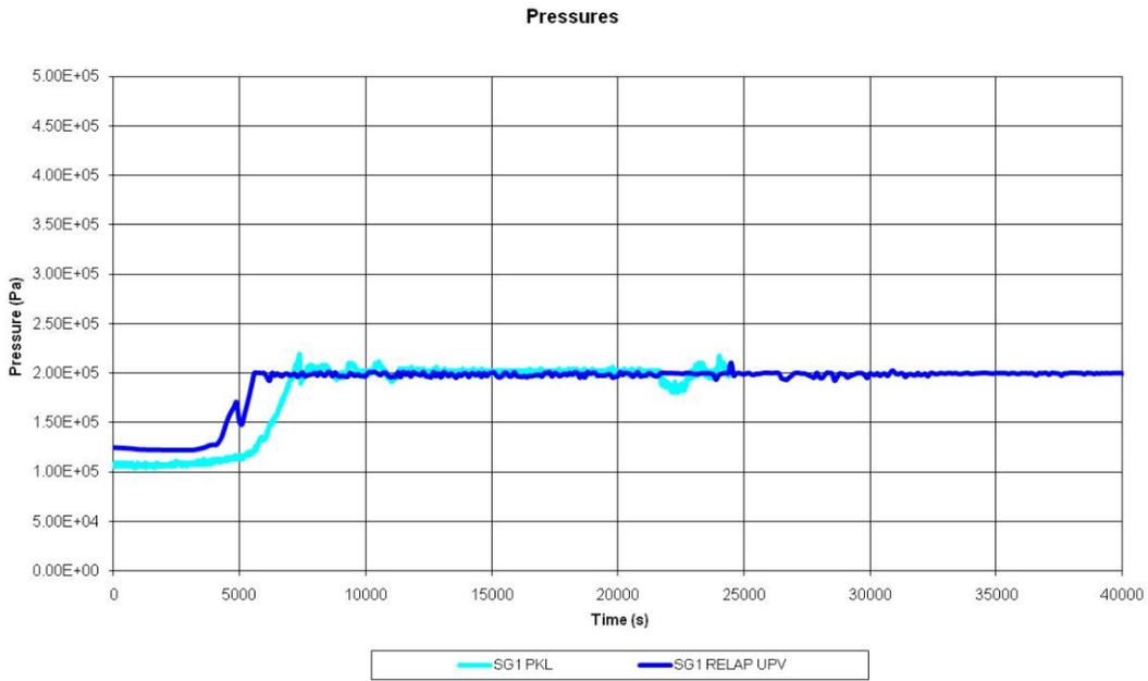
**Figure 7: Secondary side pressure in steam generator one**
