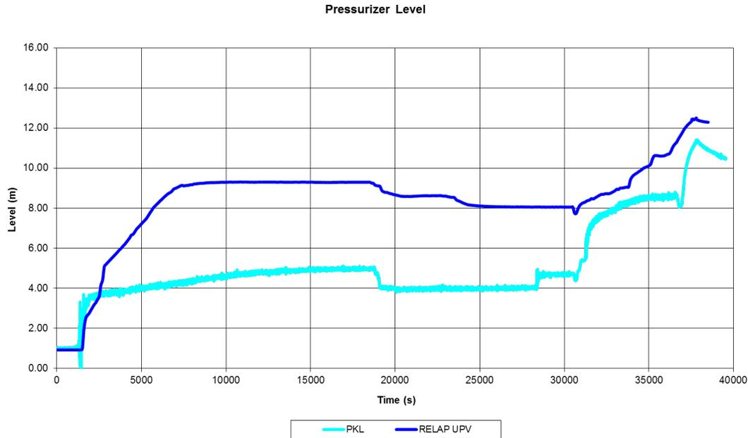
**Figure 16: Pressurizer Level**
