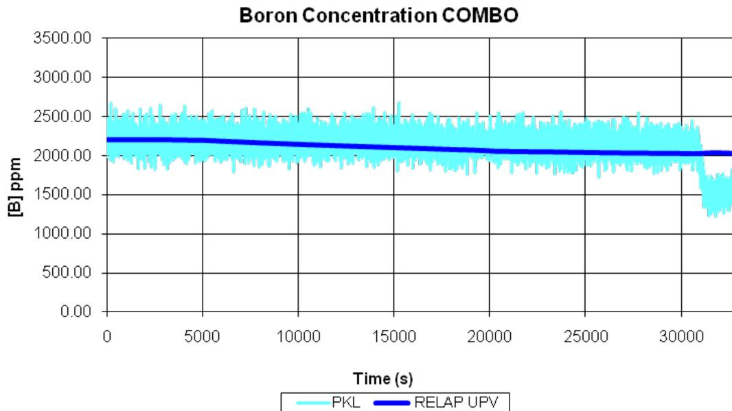
**Figure 18: Boron concentration at the core inlet**
