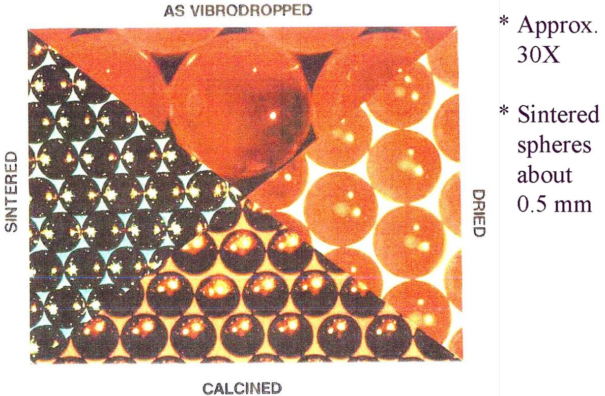
The fuel kernels are sorted by sieving to ensure 100% meet the specified size and sphericity. The finished fuel kernels are measured and classified by size and roundness within the specified tolerance band. The reference German fuel for the AVR design had a sintered fuel kernel mean diameter of 500  $\mu\text{m}$ . The PBMR fuel is based on this reference.
