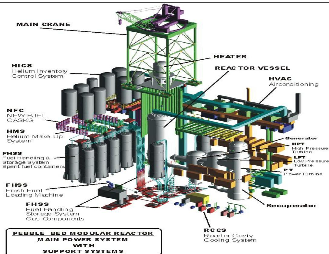
The PBMR is a helium-cooled, graphite-moderated high temperature reactor (HTR). The PBMR consists of a vertical steel pressure vessel, 6m in diameter and 20m high. The pressure vessel is lined with a layer of graphite bricks. This graphite layer serves as an outer reflector for the neutrons generated by the nuclear reaction and a passive heat transfer medium. The graphite brick lining is drilled with vertical holes to house the control elements. This graphite reflector
