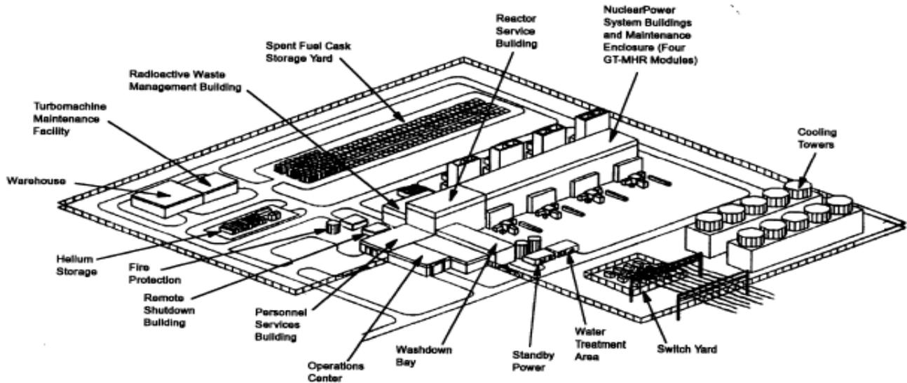
Almost all components and systems of each module, which are required to meet regulatory requirements, are independent of other modules and are localized within the individual concrete structures. These include plant protection and decay heat removal systems.
