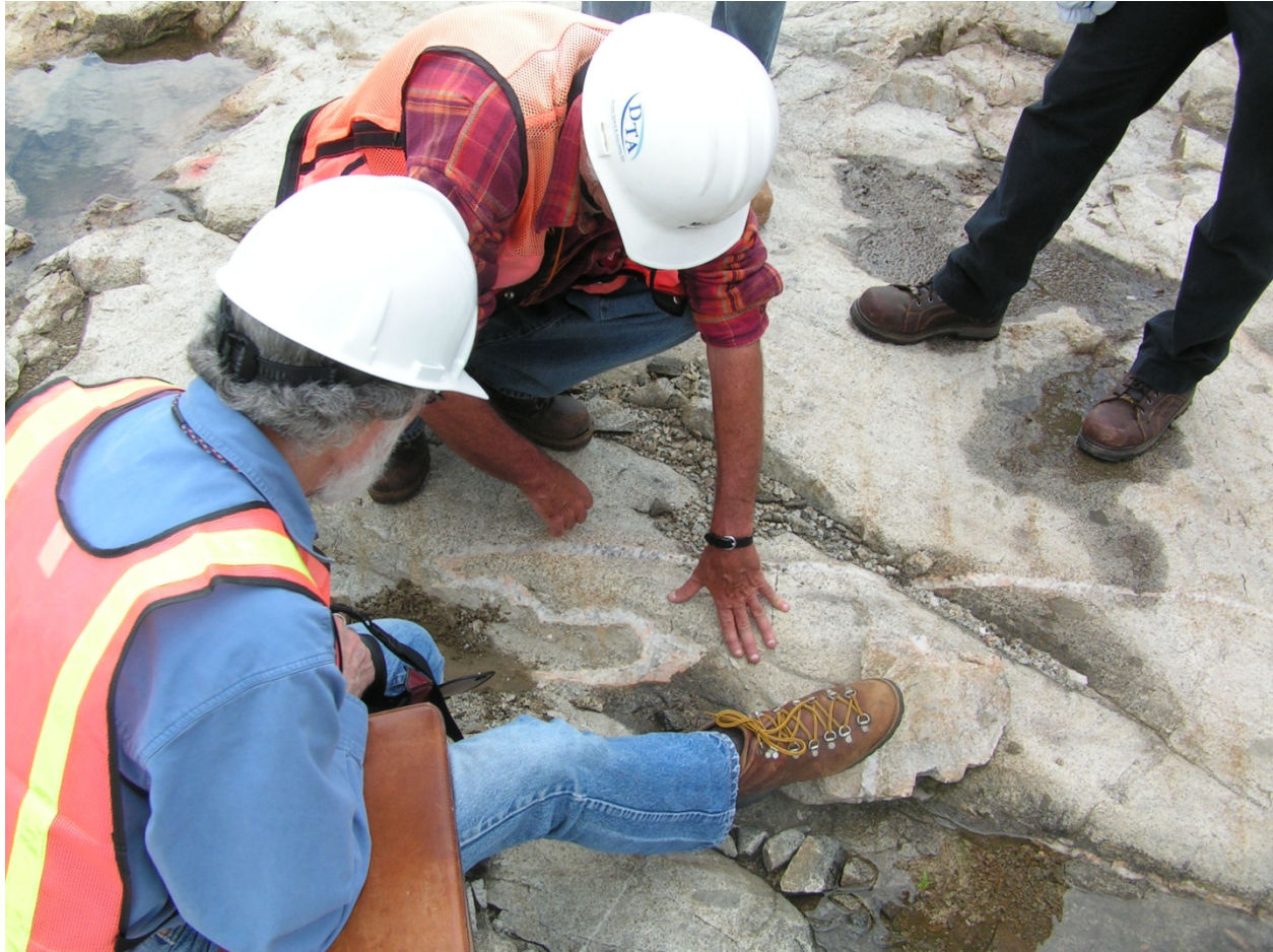
Figure 2. April-May 2008 Lee Nuclear Site Field Audit: NRC Senior Geologist, Dr. Gerry L. Stirewalt, and the applicant's geologic consultant, Dr. Malcolm Schaeffer, examining a folded igneous vein, an old deformation feature, in foundation grade level bedrock in the original CNS Unit 2 excavation.
