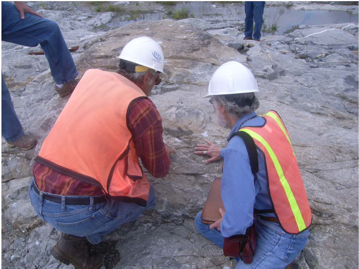
Figure 1. April-May 2008 Lee Nuclear Site Field Audit: NRC Senior Geologist, Dr. Gerry L. Stirewalt, and the applicant's geologic consultant, Dr. Malcolm Schaeffer, examining rock units and old deformation fabrics in foundation grade level bedrock in the original CNS Unit 2 excavation, which is located between Lee Nuclear Site Units 1 and 2. Dr. Schaeffer was the lead geologist involved with the original geologic mapping of all excavations at the former CNS site in the 1970s.
