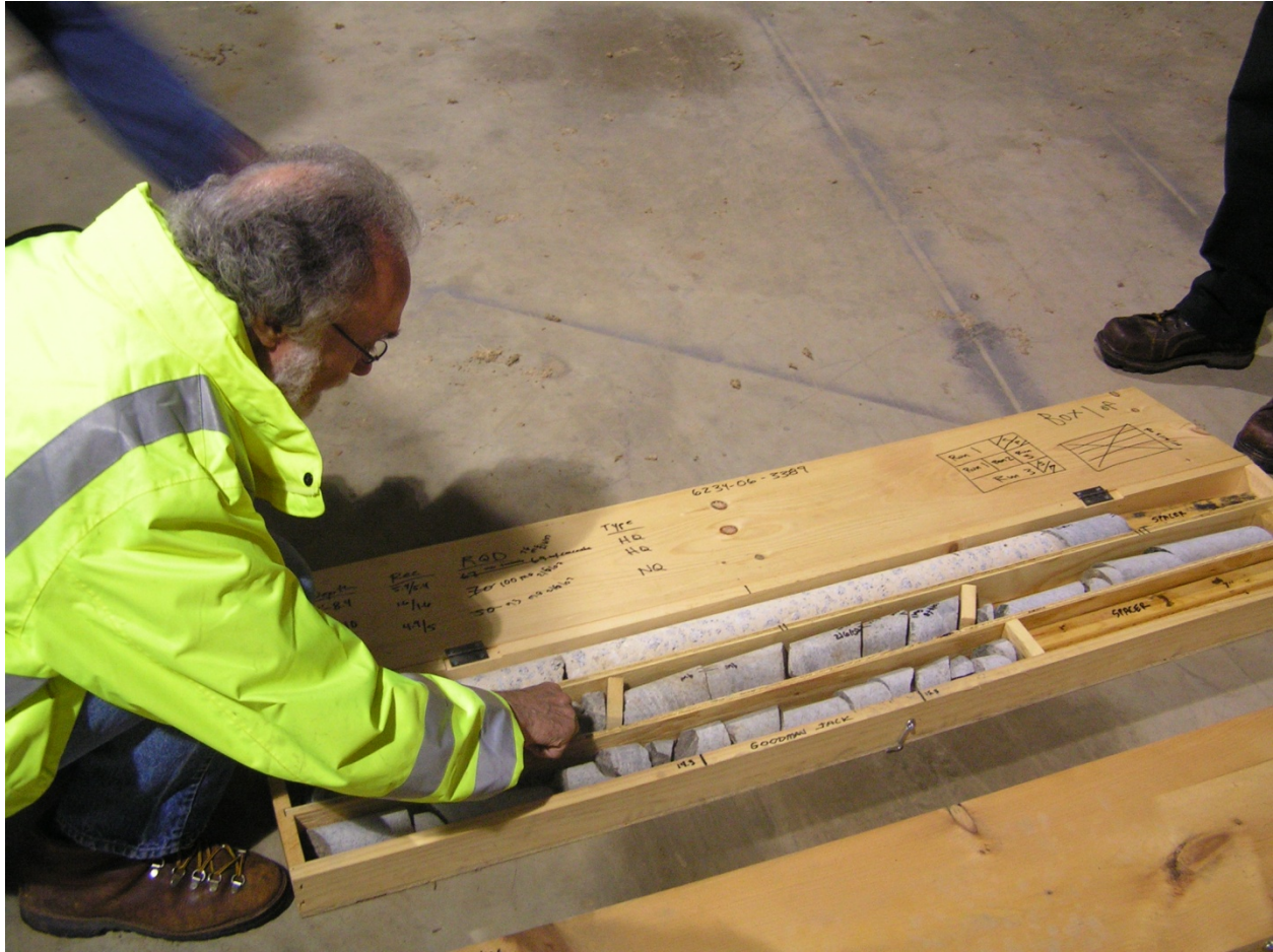
Figure 3. April-May 2008 Lee Nuclear Site Field Audit: NRC Senior Geologist, Dr. Gerry L. Stirewalt, examining core from CNS Unit 1 (Lee Nuclear Site Unit 1), including foundation bedrock (darker-colored core in the center and on the right side of the core box) and old concrete (lighter-colored core on the left side of the core box) currently covering the excavation for former CNS Unit 1 (Lee Nuclear Site Unit 1). The contact between the old concrete and bedrock is shown by the color change in the core at the upper left side of the core box. This core was taken during site characterization investigations for the Lee Nuclear Site COL application specifically to penetrate the old concrete and extend into foundation bedrock.
