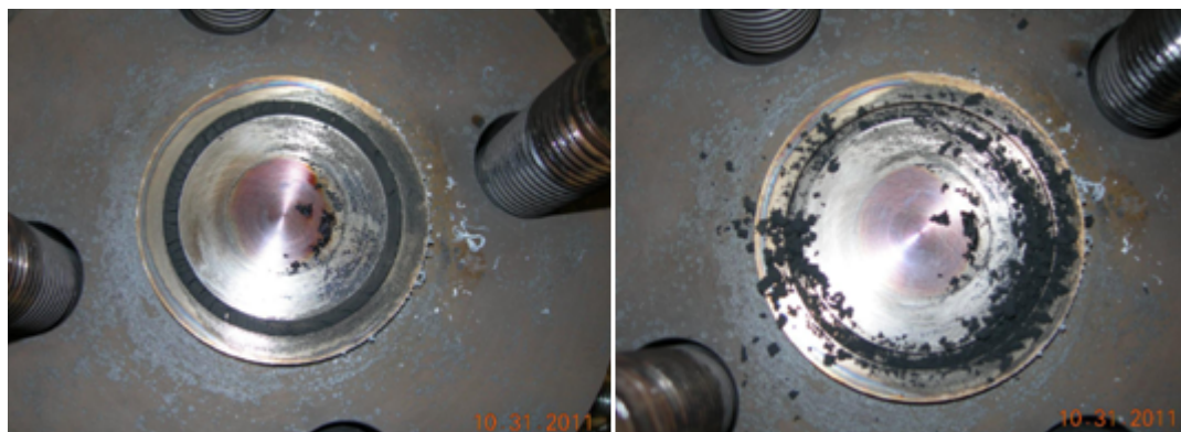
Figure 6: Photograph of Test #15 ethylene-propylene O-ring after heat up showing packed layer of powdery charred material (left) and destroyed seal after the attempt to remove it (right)
