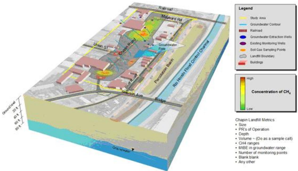
Figure 5.3 An advanced conceptual site model integrated into a GIS/Visualization system (courtesy of VisualNavigator.com).
