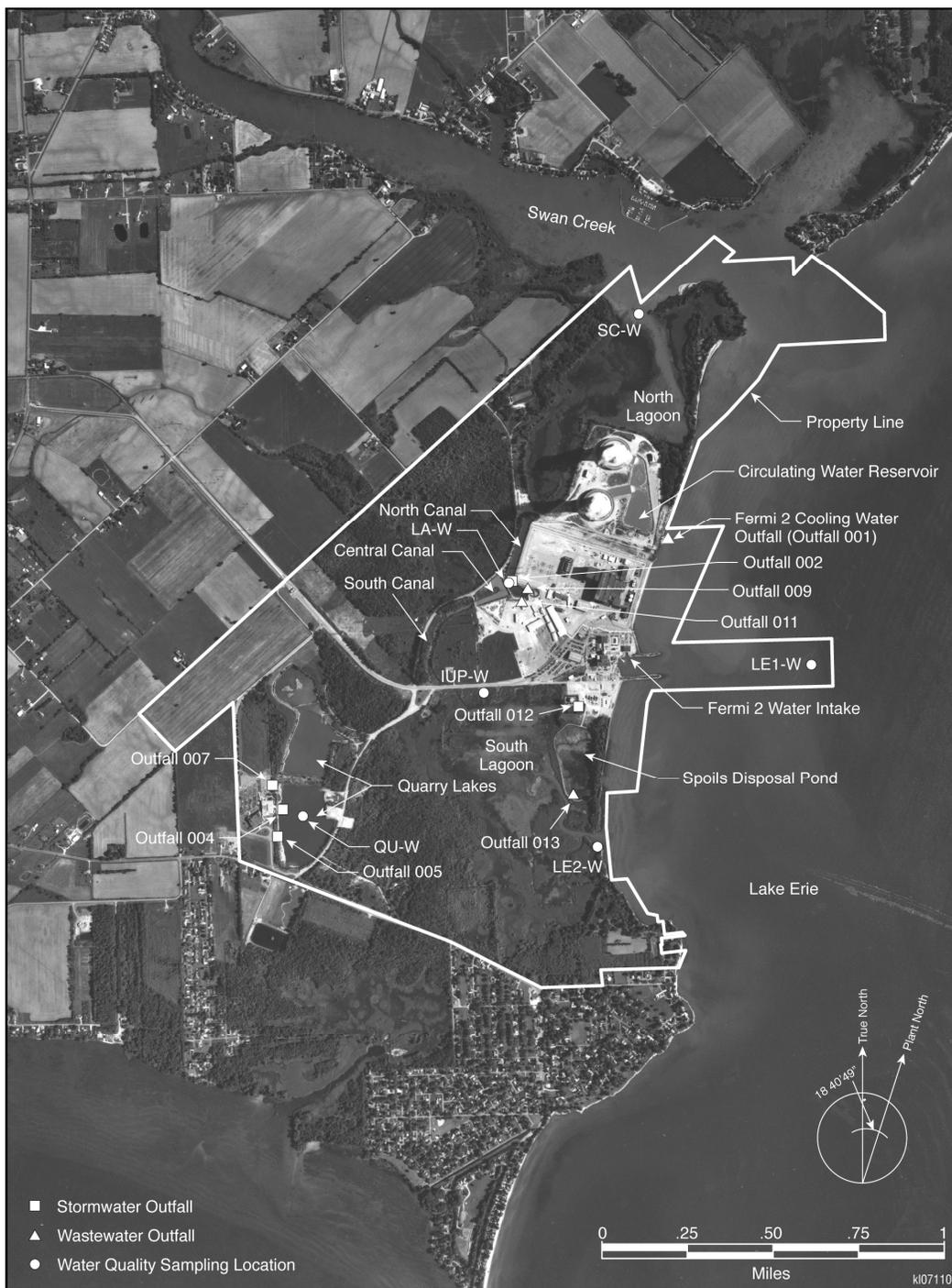
**Figure 2-4.** Surface Water Features, Discharge Outfalls, and Water Quality Sampling Locations on the Fermi Site
