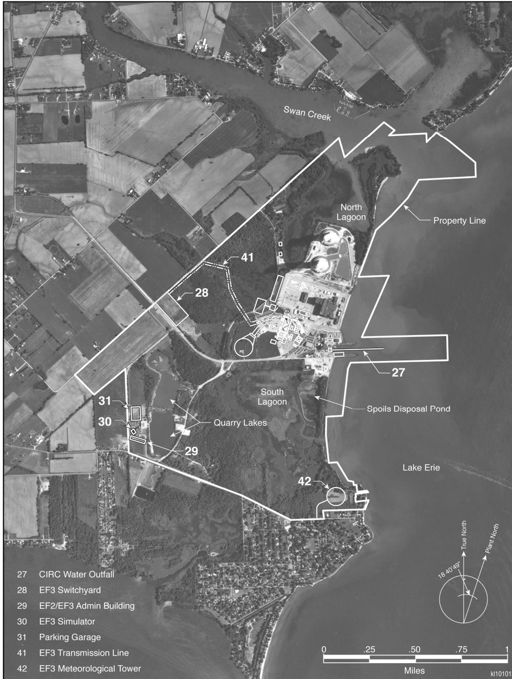
**Figure 2-1.** Fermi Site and Proposed Fermi 3 Facilities (Source: Detroit Edison 2011a)
